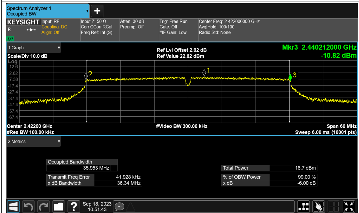
-6dB Bandwidth NVNT n40 2437MHz Ant14
