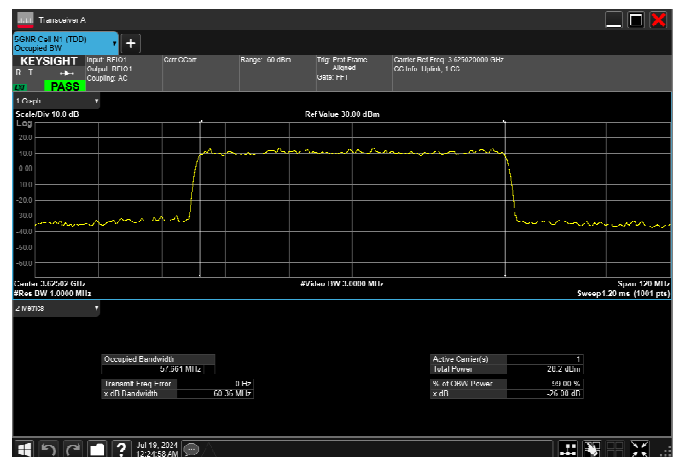
n78_2_60MHz_30kHz_3625MHz_DFT-s-OFDM 16 QAM_RB162@0 57.661MHz
