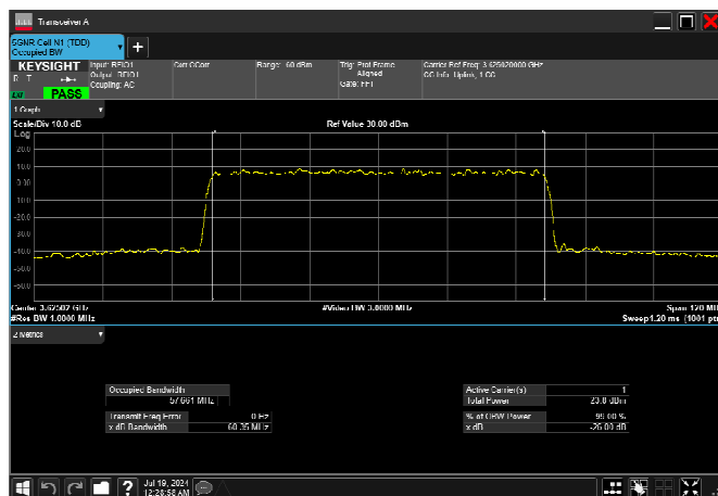
n78_2_60MHz_30kHz_3625MHz_CP-OFDM 256 QAM_RB162@0 57.661MHz
