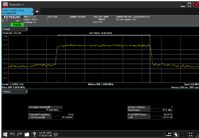
n78_2_80MHz_30kHz_3625MHz_CP-OFDM 64 QAM_RB217@0 77.245MHz
