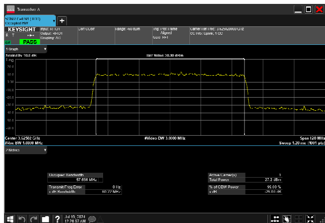
n78_2_60MHz_30kHz_3625MHz_CP-OFDM 64 QAM_RB162@0 57.680MHz
