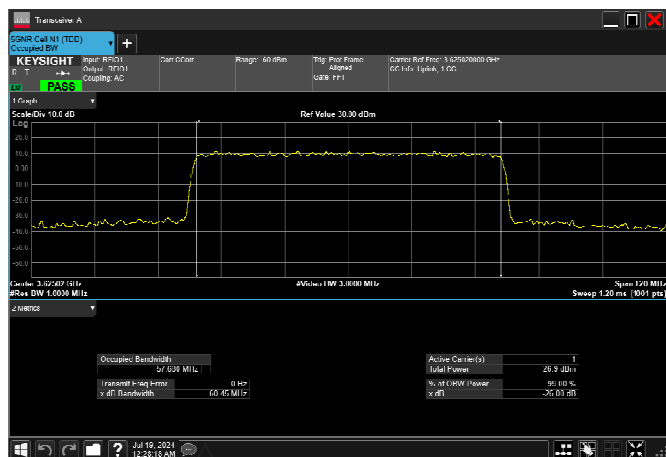
n78_2_60MHz_30kHz_3625MHz_CP-OFDM 64 QAM_RB162@0 57.680MHz
