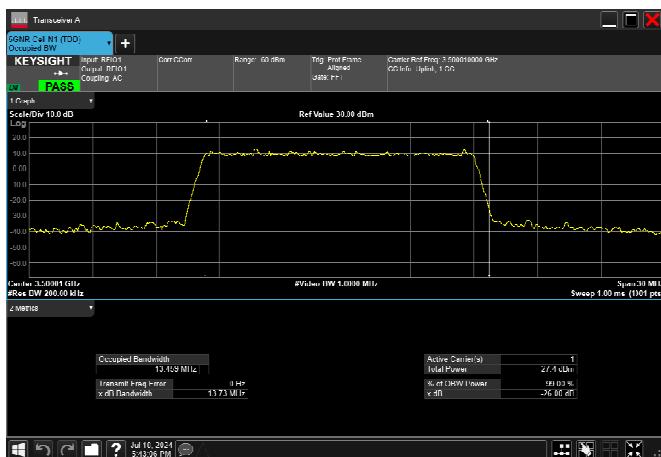
n77_1_15MHz_30kHz_3500MHz_DFT-s-OFDM QPSK_RB36@0 13.459MHz
