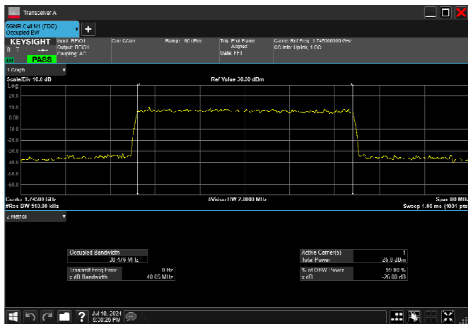
n66_40MHz_15kHz_1745MHz_CP-OFDM QPSK_RB216@0 38.446MHz
