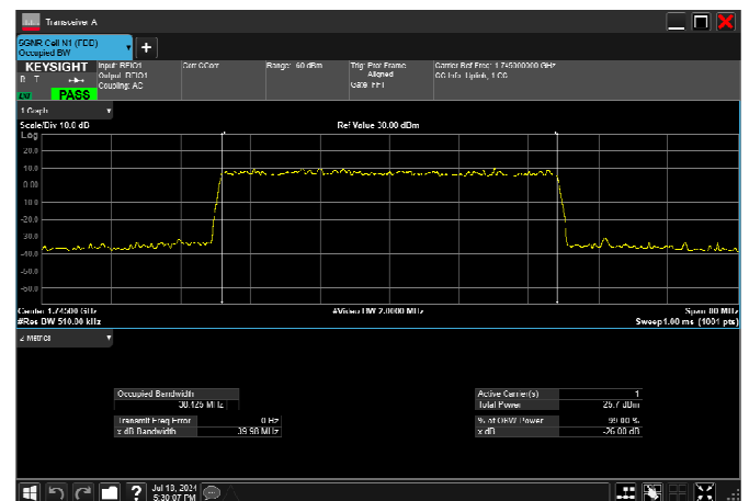
n66_40MHz_15kHz_1745MHz_DFT-s-OFDM 16 QAM_RB216@0 38.425MHz
