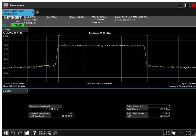
n77_1_50MHz_30kHz_3500MHz_DFT-s-OFDM QPSK_RB128@0 47.281MHz
