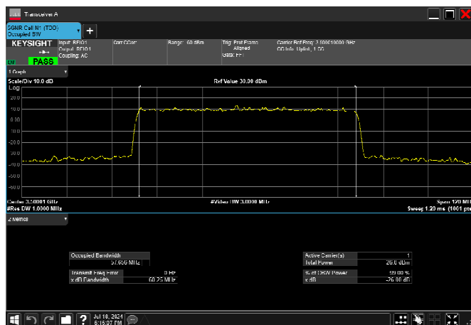
n77_1_60MHz_30kHz_3500MHz_CP-OFDM QPSK_RB162@0 57.656MHz
