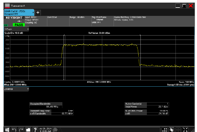
n77_1_70MHz_30kHz_3500MHz_DFT-s-OFDM 16 QAM_RB180@0 66.566MHz
