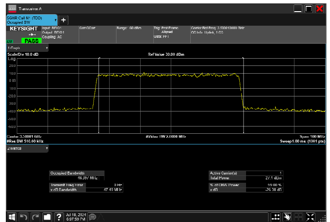
n77_1_50MHz_30kHz_3500MHz_DFT-s-OFDM 16 QAM_RB128@0 46.897MHz
