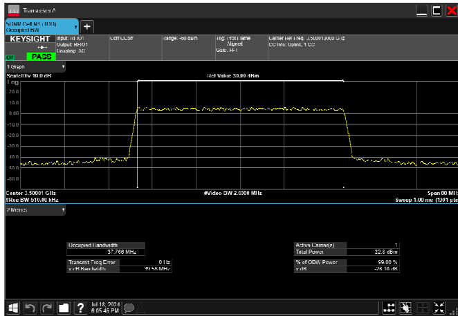
n77_1_50MHz_30kHz_3500MHz_DFT-s-OFDM QPSK_RB128@0 47.281MHz
