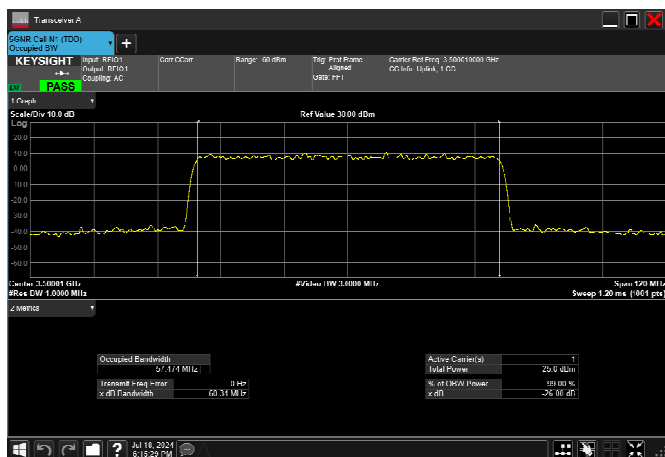
n77_1_60MHz_30kHz_3500MHz_DFT-s-OFDM 256 QAM_RB162@0 57.474MHz
