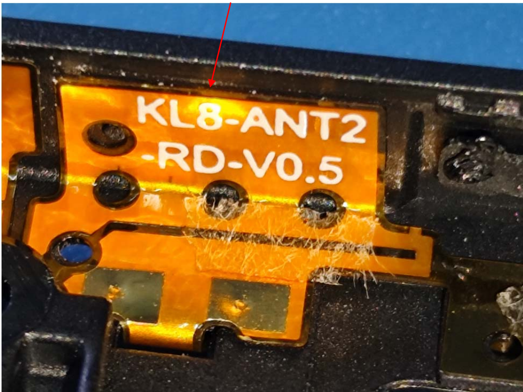
ANT2 (BT/WIFI_2.4G (chain 1) + B42/N77/78 PRX MIMO)
