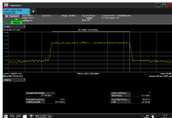
n77_3_50MHz_30kHz_3840MHz_DFT-s-OFDM \pi/2 BPSK RB128@0 47.046MHz
