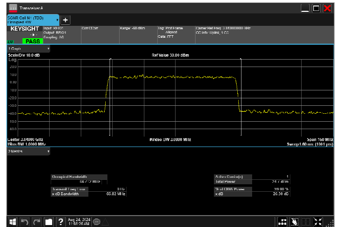
n77_3_70MHz_30kHz_3840MHz_DFT-s-OFDM 16 QAM_RB180@0 66.348MHz
