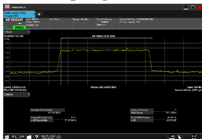
n77_3_50MHz_30kHz_3840MHz_DFT-s-OFDM 16 QAM RB128@0 47.029MHz
