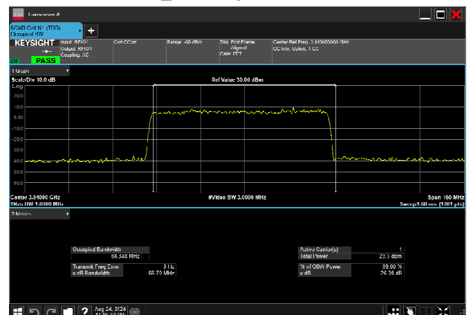
n77_3_70MHz_30kHz_3840MHz_DFT-s-OFDM 16 QAM_RB180@0 66.348MHz
