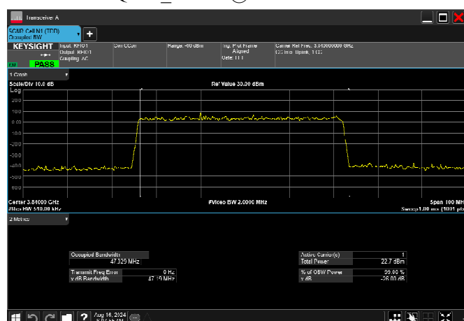
n77_3_50MHz_30kHz_3840MHz_DFT-s-OFDM 16 QAM RB128@0 47.029MHz
