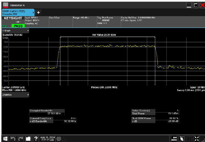
n77_3_70MHz_30kHz_3840MHz_DFT-s-OFDM QPSK_RB180@0 66.645MHz
