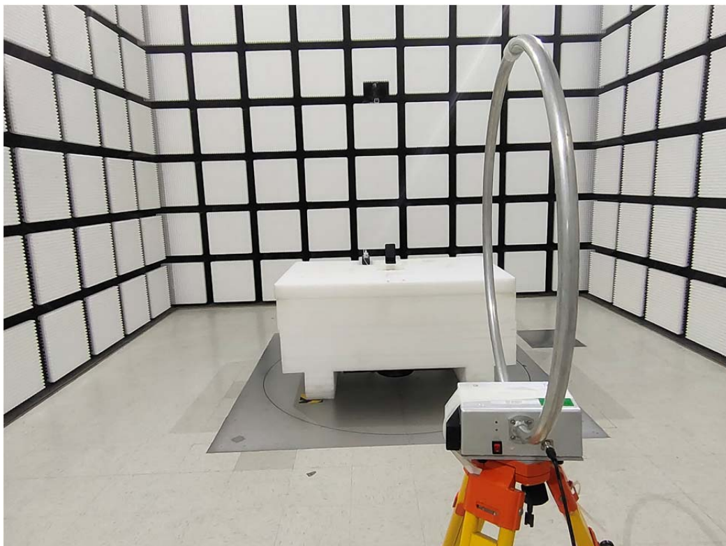
Radiated Emission 9 kHz-30 MHz Perpendicular View
