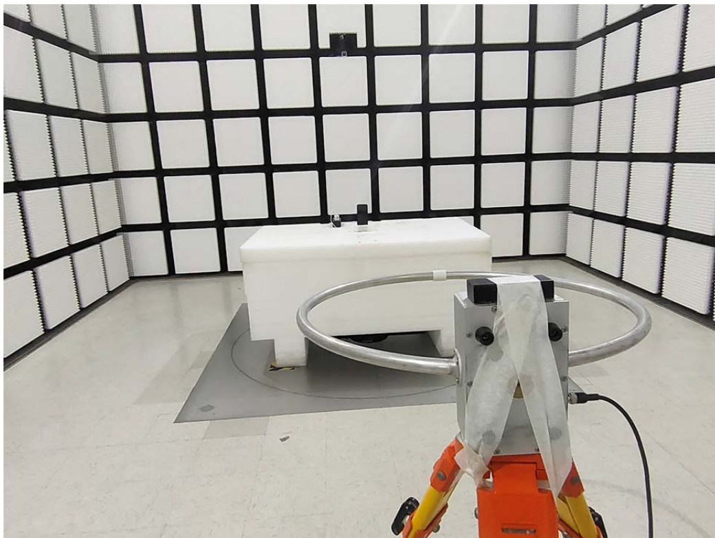
Radiated Emission 9 kHz-30 MHz Ground-parallel View
