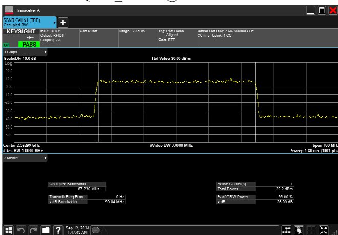
n41_90MHz_30kHz_2592.99MHz_CP-OFDM 64 QAM_RB245@0 87.236MHz
