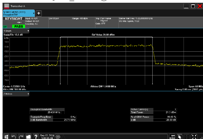
n66_30MHz_15kHz_1725MHz_CP-OFDM 256 OAM RB160@0 28.490MHz
