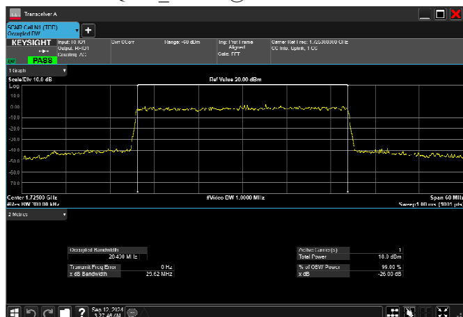
n66_30MHz_15kHz_1725MHz_CP-OFDM 256 OAM RB160@0 28.490MHz
