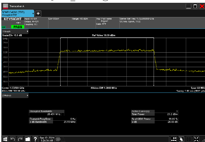
n66_30MHz_15kHz_1725MHz_DFT-s-OFDM QPSK_RB160@0 28.491MHz
