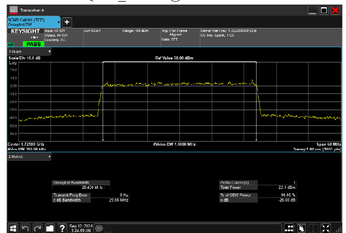
n66_30MHz_15kHz_1725MHz_DFT-s-OFDM 16 QAM_RB160@0 28.460MHz
