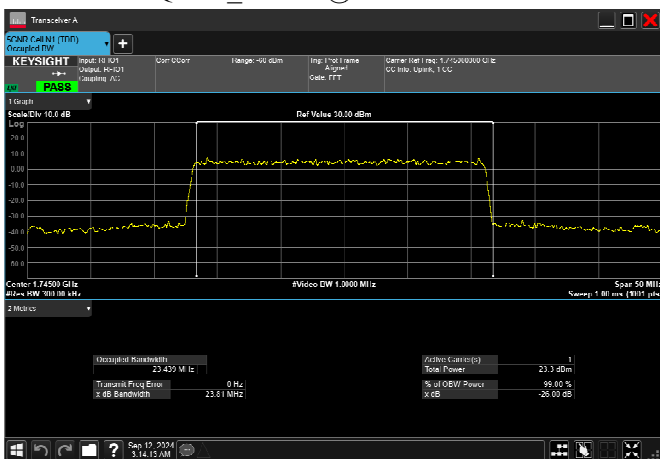
n66_25MHz_15kHz_1745MHz_DFT-s-OFDM QPSK_RB128@0 23.439MHz
