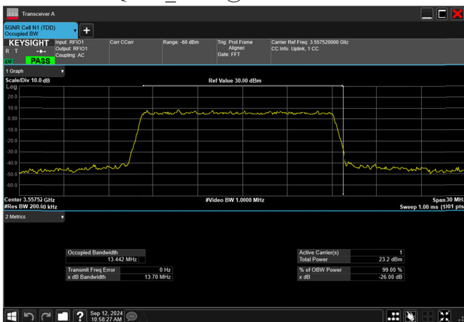
n77_2_15MHz_30kHz_3557.5MHz_DFT-s-OFDM QPSK_RB36@0 13.442MHz
