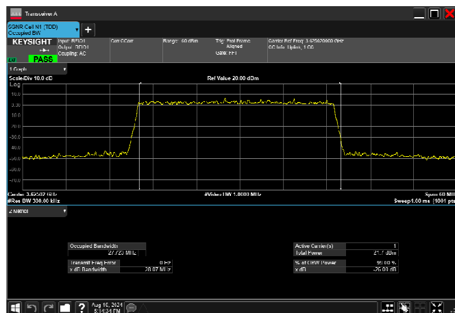
n77_2_30MHz_30kHz_3625MHz_DFT-s-OFDM 16 QAM RB75@0 27.723MHz
