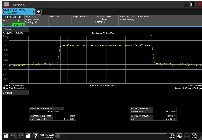
n78_3_50MHz_30kHz_3750MHz_CP-OFDM 256 QAM_RB133@0 47.282MHz
