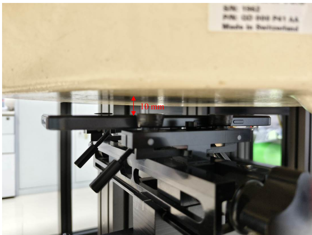
Body (Worn) Back Setup Photo (10 mm)
