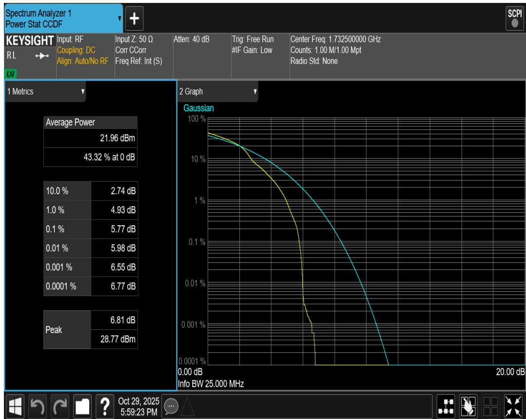
Band4 QAM16 BW=3MHz Channel=20175 RB Size=1 Position=#0
