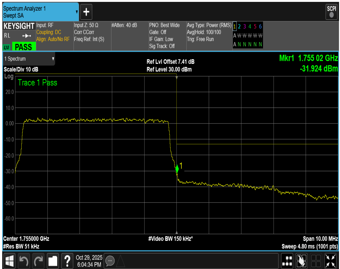
Band4 QPSK BW=1.4MHz Channel=19957 RB Size=6 Position=#0
