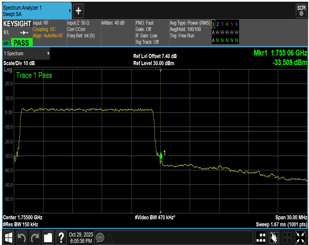
Band4 QAM16 BW=20MHz Channel=20050 RB Size=100 Position=#0
