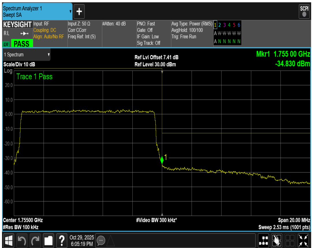
Band4 QAM16 BW=15MHz Channel=20025 RB Size=75 Position=#0
