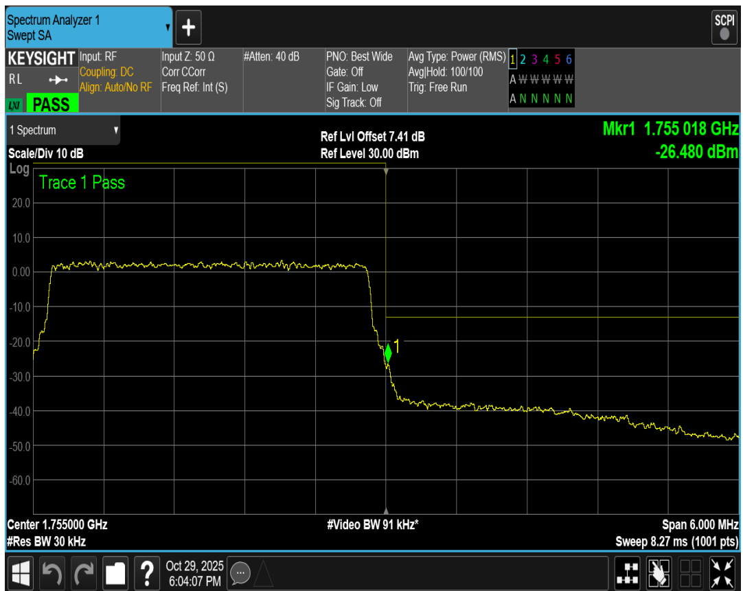
Band4 QAM16 BW=5MHz Channel=19975 RB Size=25 Position=#0
