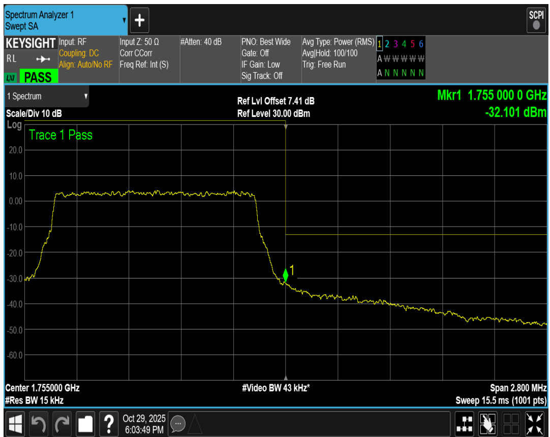
Band4 QAM16 BW=10MHz Channel=20000 RB Size=50 Position=#0
