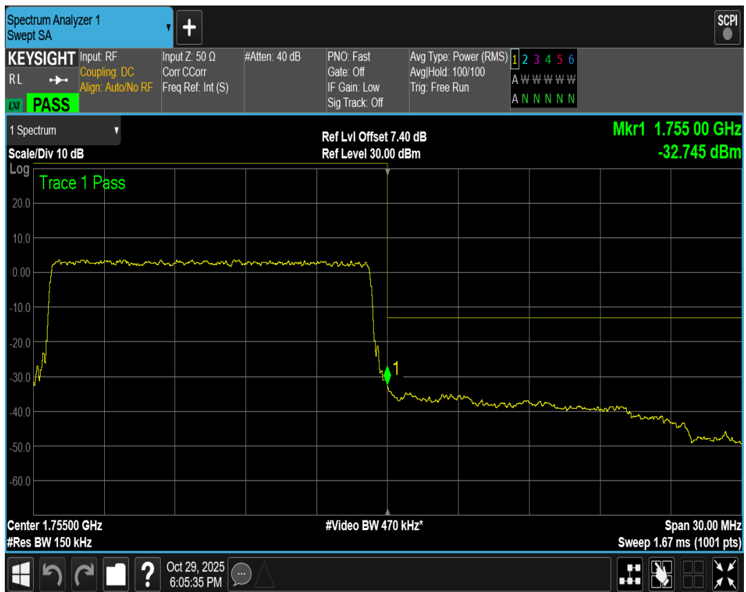
Band4 QPSK BW=20MHz Channel=20050 RB Size=100 Position=#0
