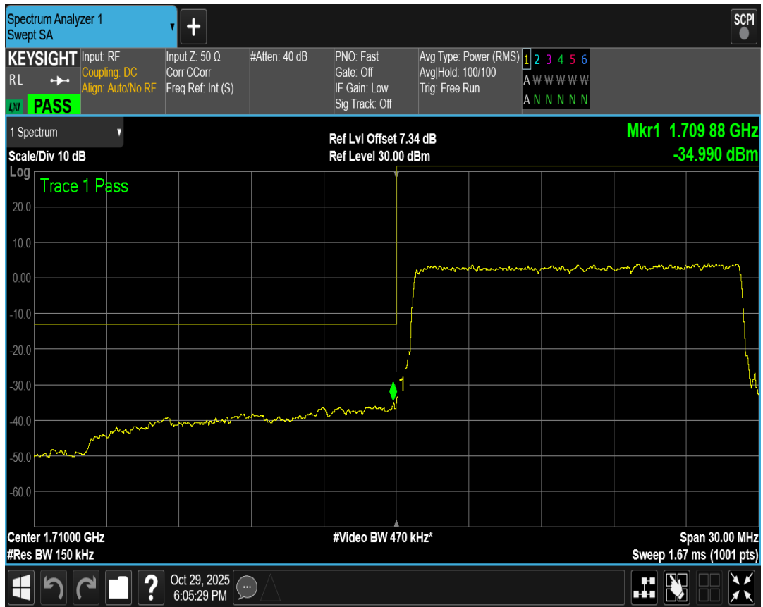
Band4 QPSK BW=15MHz Channel=20325 RB Size=75 Position=#0
