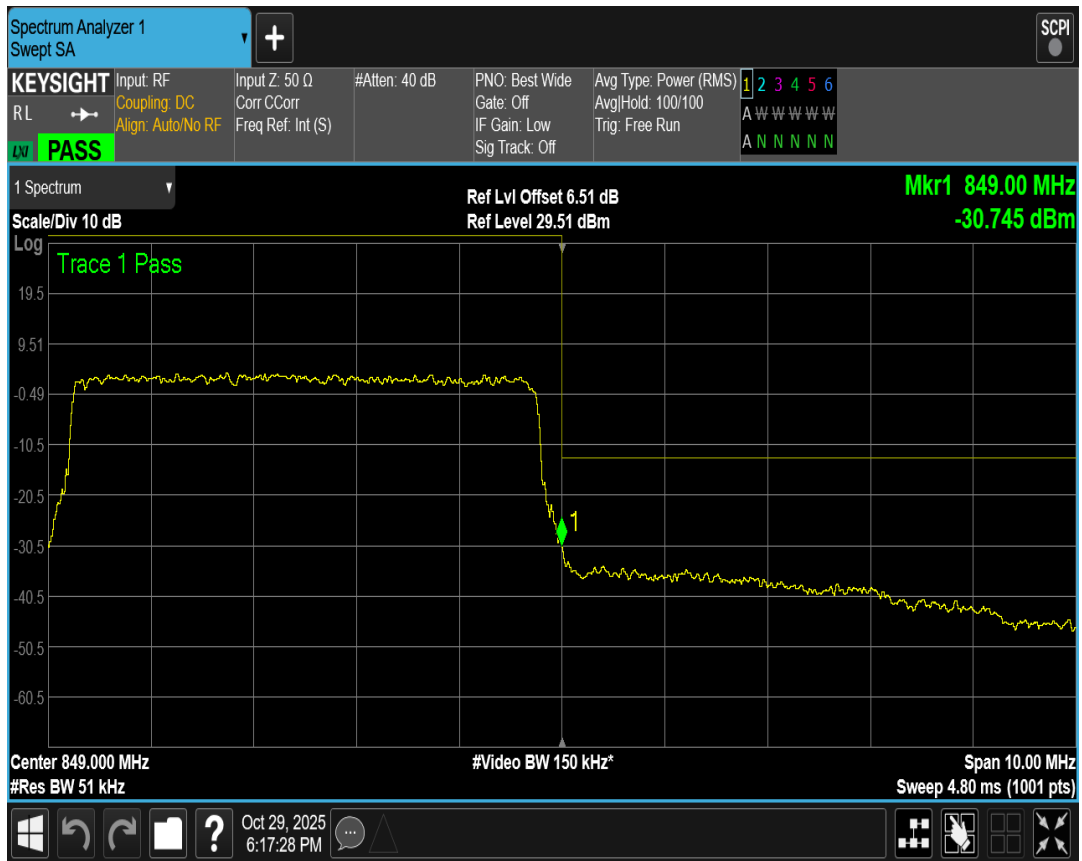
Band5 QPSK BW=1.4MHz Channel=20407 RB Size=6 Position=#0
