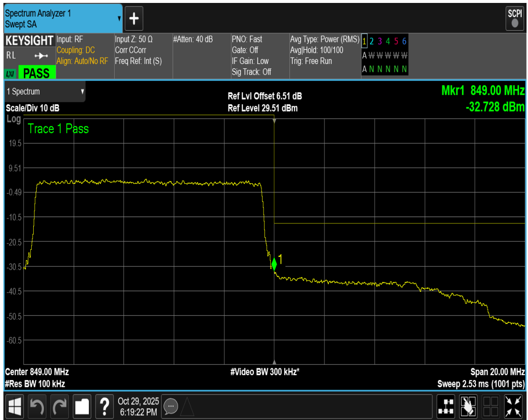
Band5 QPSK BW=3MHz Channel=20415 RB Size=15 Position=#0
