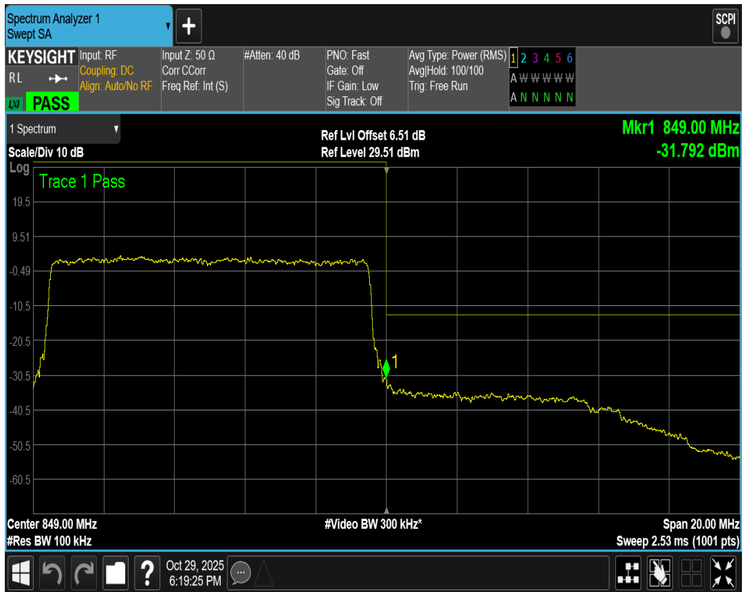
Band5 QAM16 BW=3MHz Channel=20415 RB Size=15 Position=#0
