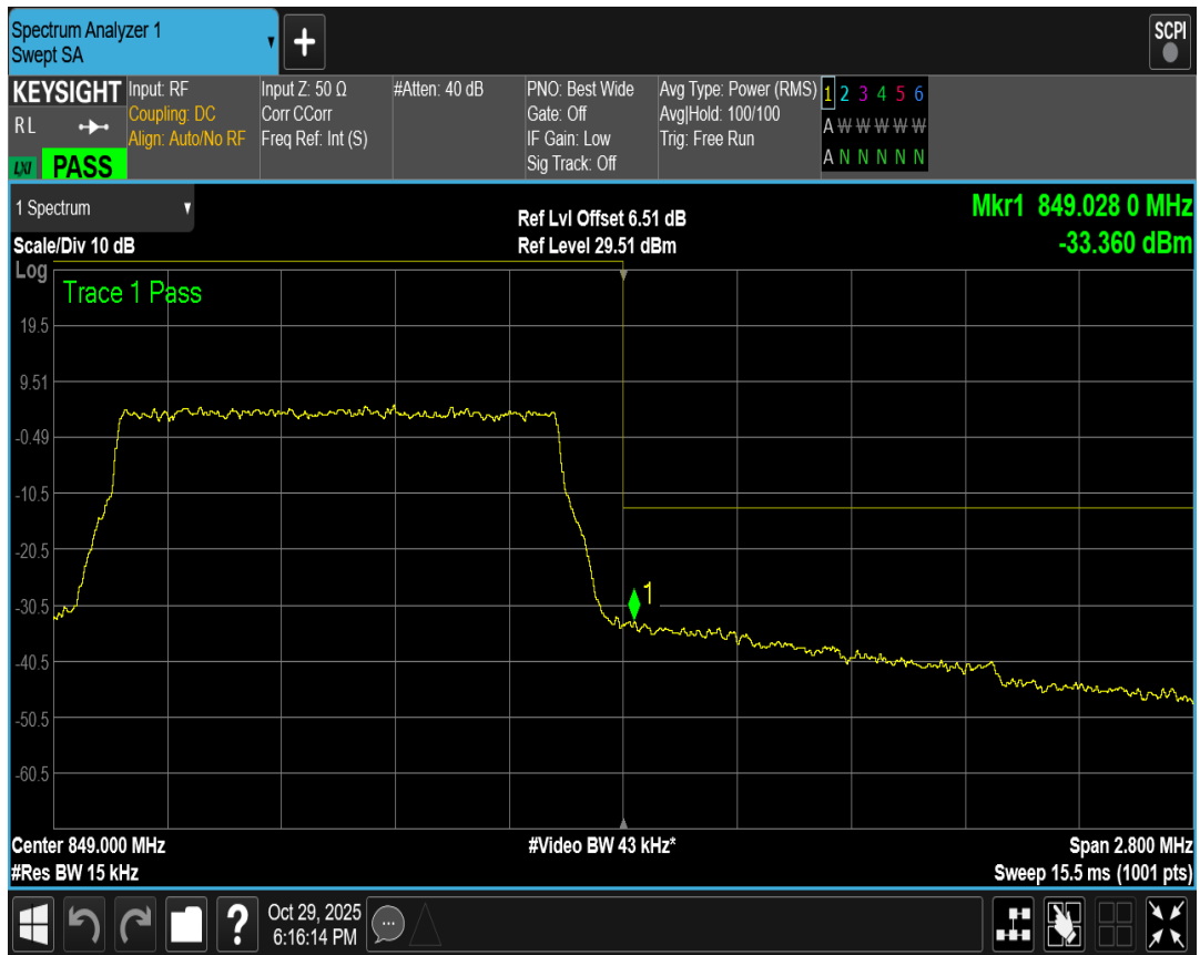
Band5 QAM16 BW=10MHz Channel=20450 RB Size=50 Position=#0
