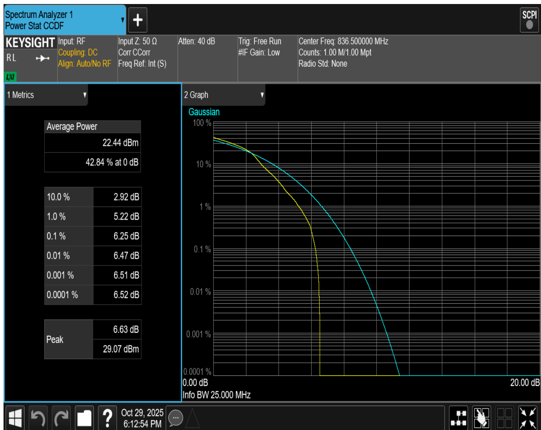
Band5 QAM16 BW=5MHz Channel=20525 RB Size=1 Position=#0
