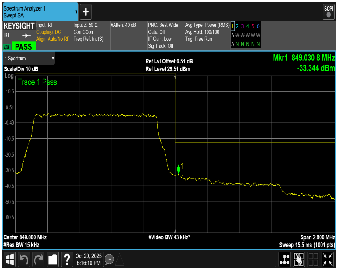
Band5 QPSK BW=10MHz Channel=20450 RB Size=50 Position=#0
