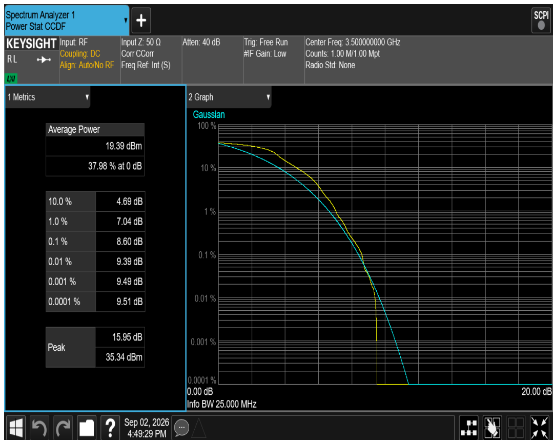
Band42(3450-3550) QPSK BW=15MHz Channel=42590 RB Size=1 Position=#0
