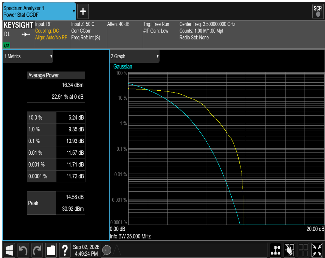
Band42(3450-3550) QPSK BW=10MHz Channel=42590 RB Size=1 Position=#0
