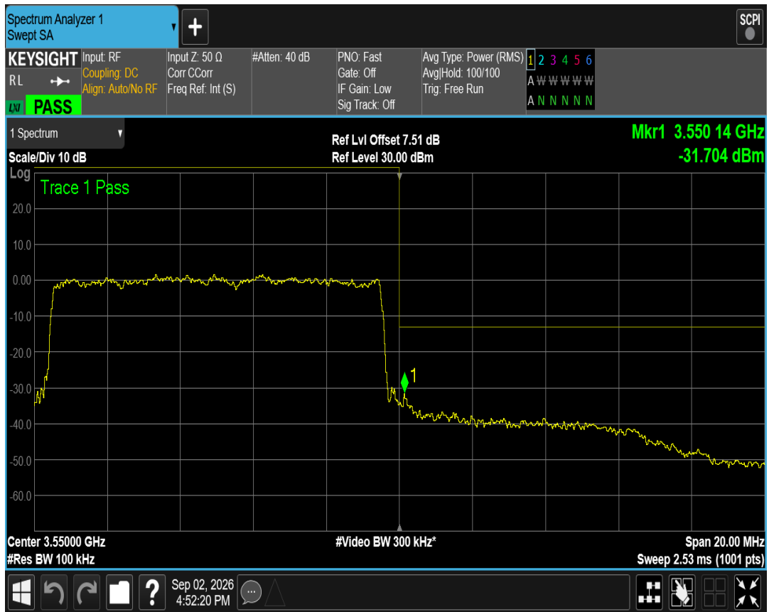
Band42(3450-3550) QPSK BW=15MHz Channel=42165 RB Size=75 Position=#0
