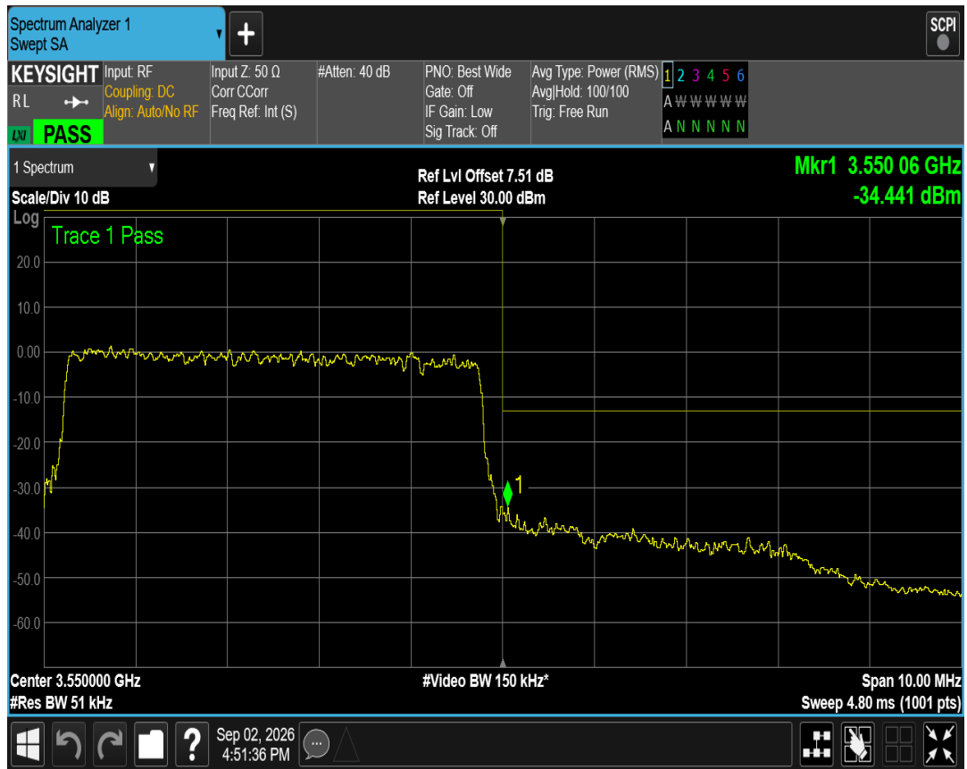
Band42(3450-3550) QPSK BW=10MHz Channel=42140 RB Size=50 Position=#0
