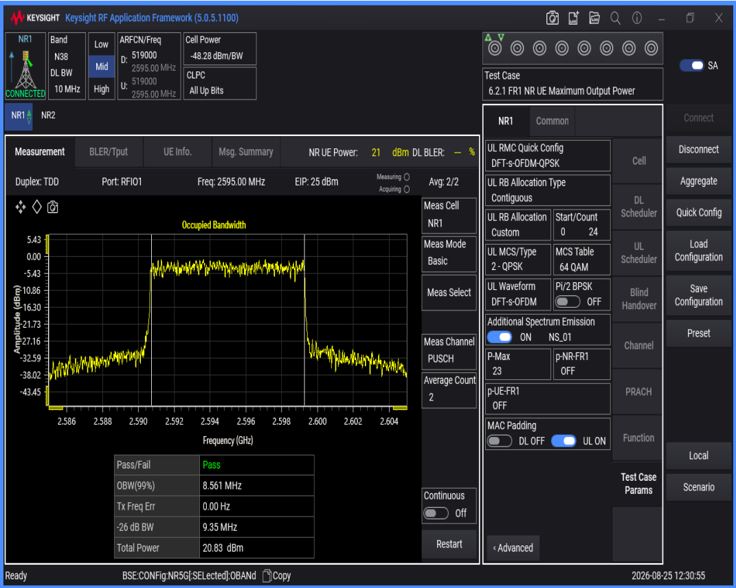
n38 SCS=30kHz DFT_QAM16 BW=10MHz Channel=519000 RB=24@0
