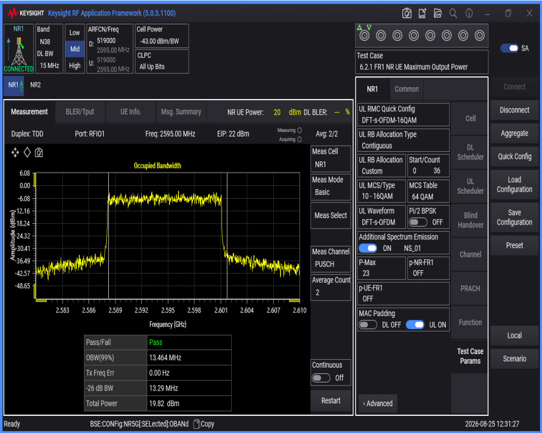
n38 SCS=30kHz DFT_QAM64 BW=15MHz Channel=519000 RB=36@0
