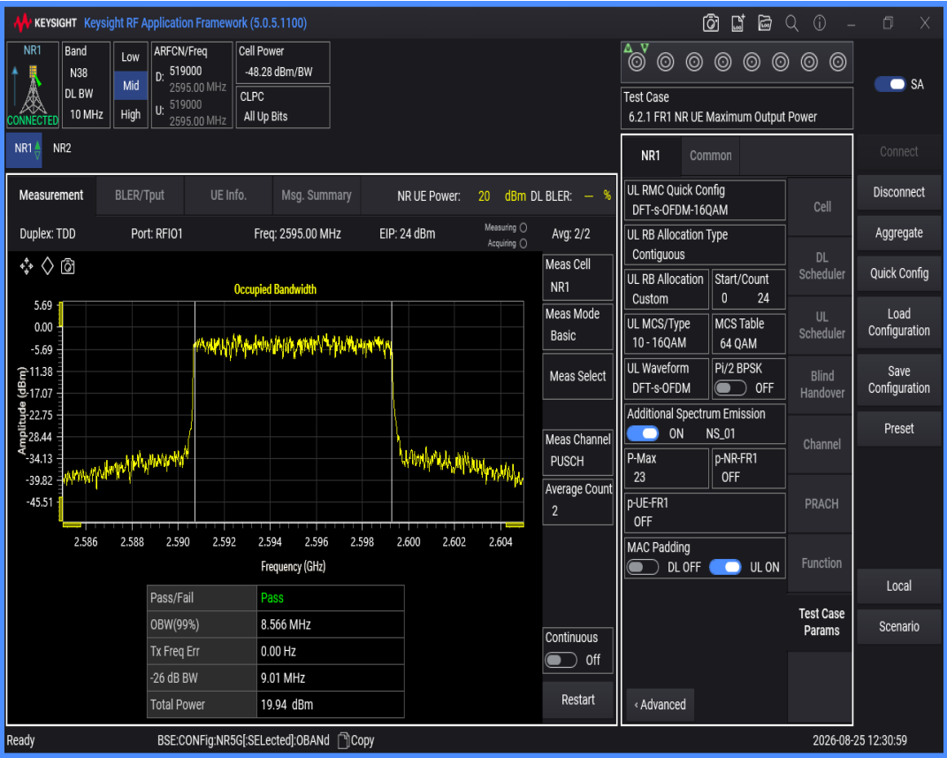
n38 SCS=30kHz DFT_QAM64 BW=10MHz Channel=519000 RB=24@0
