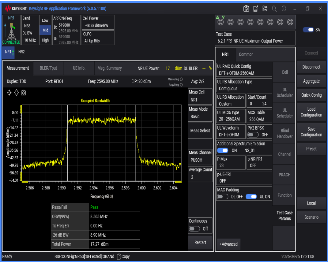
n38 SCS=30kHz DFT_BPSK BW=15MHz Channel=519000 RB=36@0
