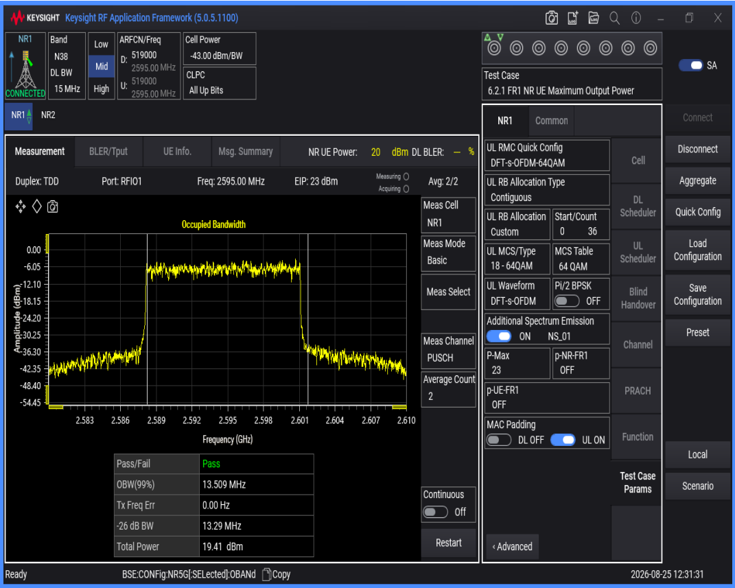
n38 SCS=30kHz DFT_QAM256 BW=15MHz Channel=519000 RB=36@0
