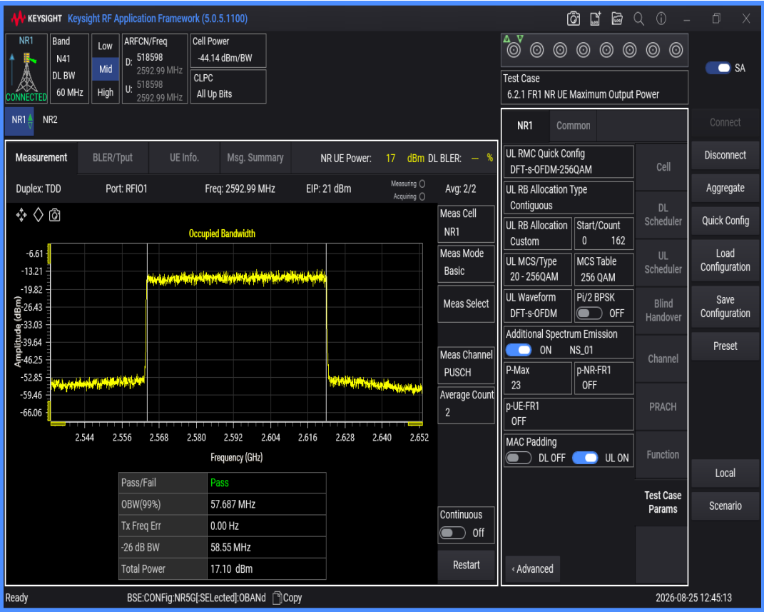
n41 SCS=30kHz DFT_BPSK BW=80MHz Channel=518598 RB=216@0
