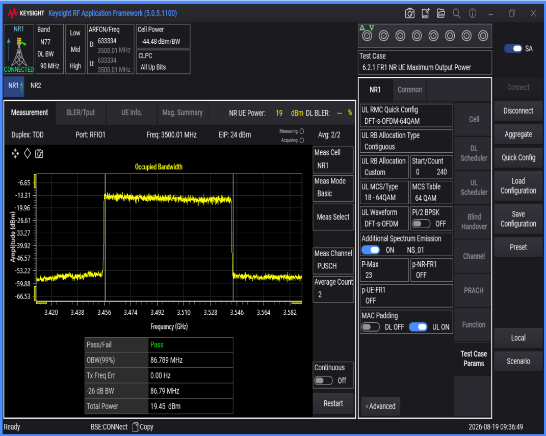
n77(3450-3550) SCS=30kHz DFT_QAM256 BW=90MHz Channel=633334 RB=240@0
