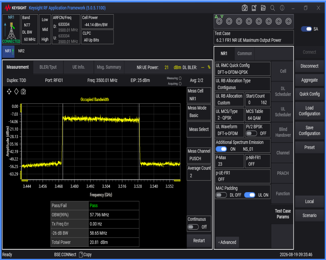
n77(3450-3550) SCS=30kHz DFT_QAM16 BW=60MHz Channel=633334 RB=162@0
