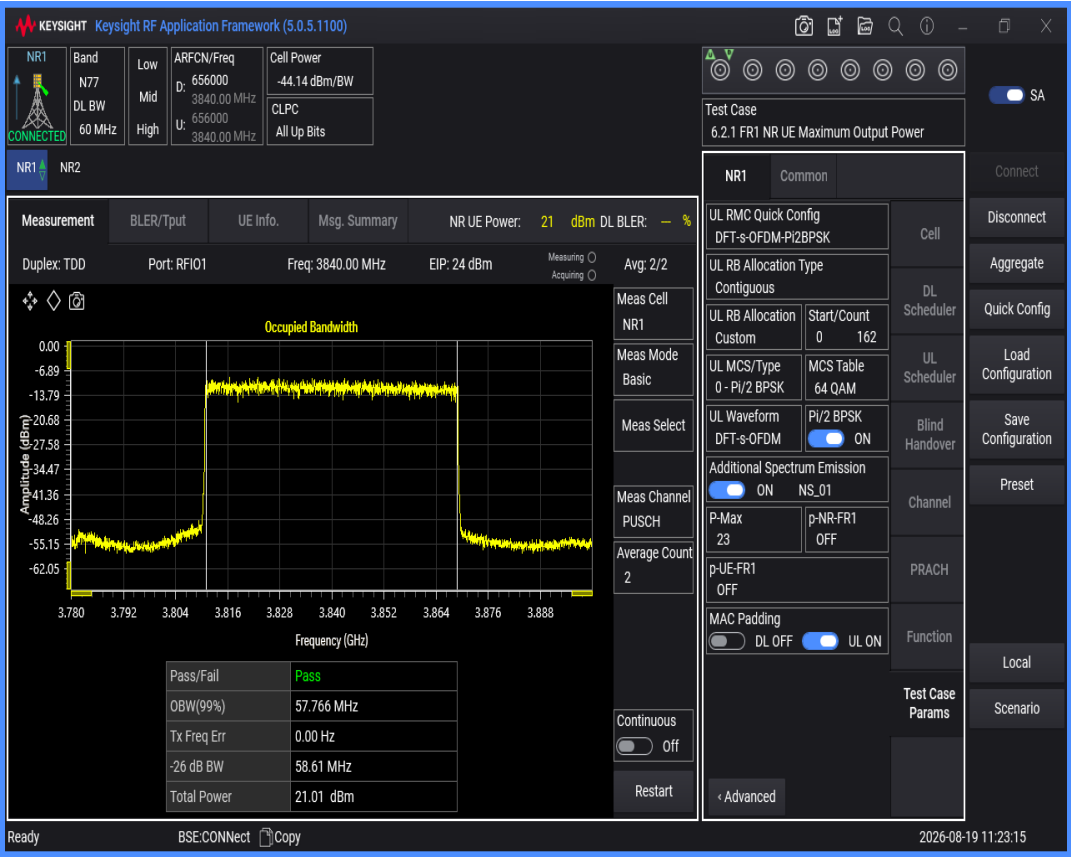
n77(3700-3980) SCS=30kHz DFT_QPSK BW=60MHz Channel=656000 RB=162@0
