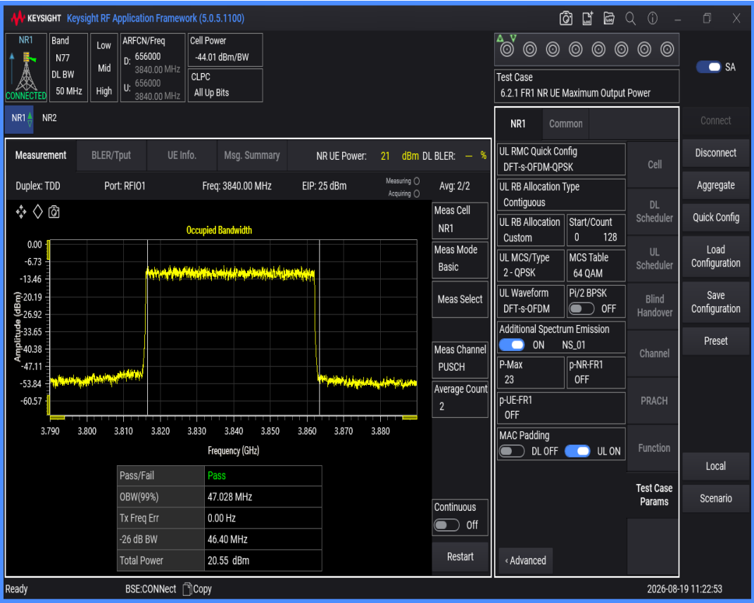
n77(3700-3980) SCS=30kHz DFT_QAM16 BW=50MHz Channel=656000 RB=128@0
