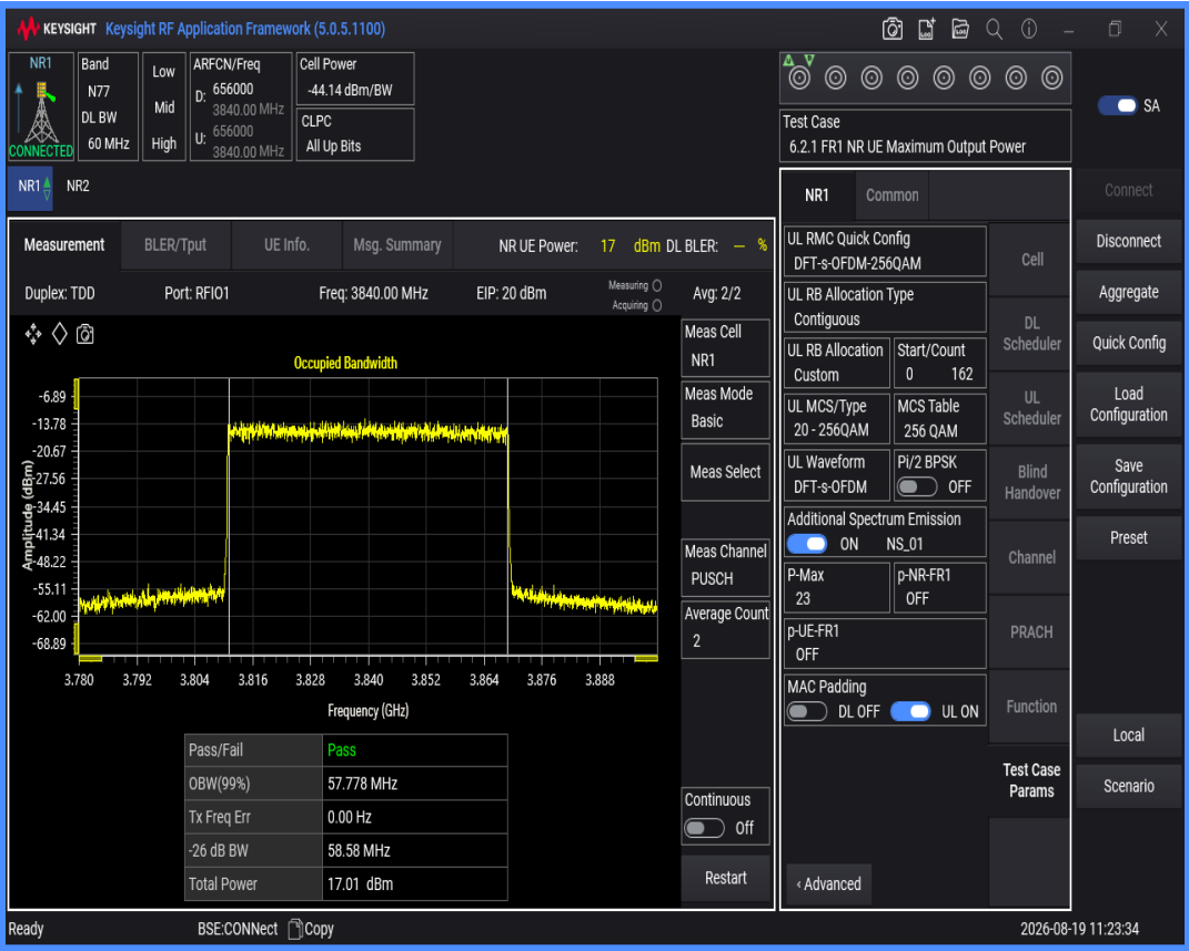
n77(3700-3980) SCS=30kHz DFT_BPSK BW=80MHz Channel=656000 RB=216@0
