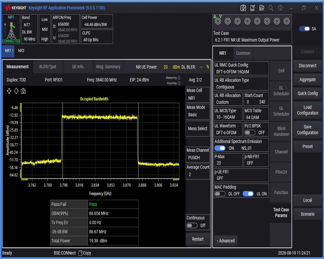
n77(3700-3980) SCS=30kHz DFT_QAM64 BW=90MHz Channel=656000 RB=240@0
