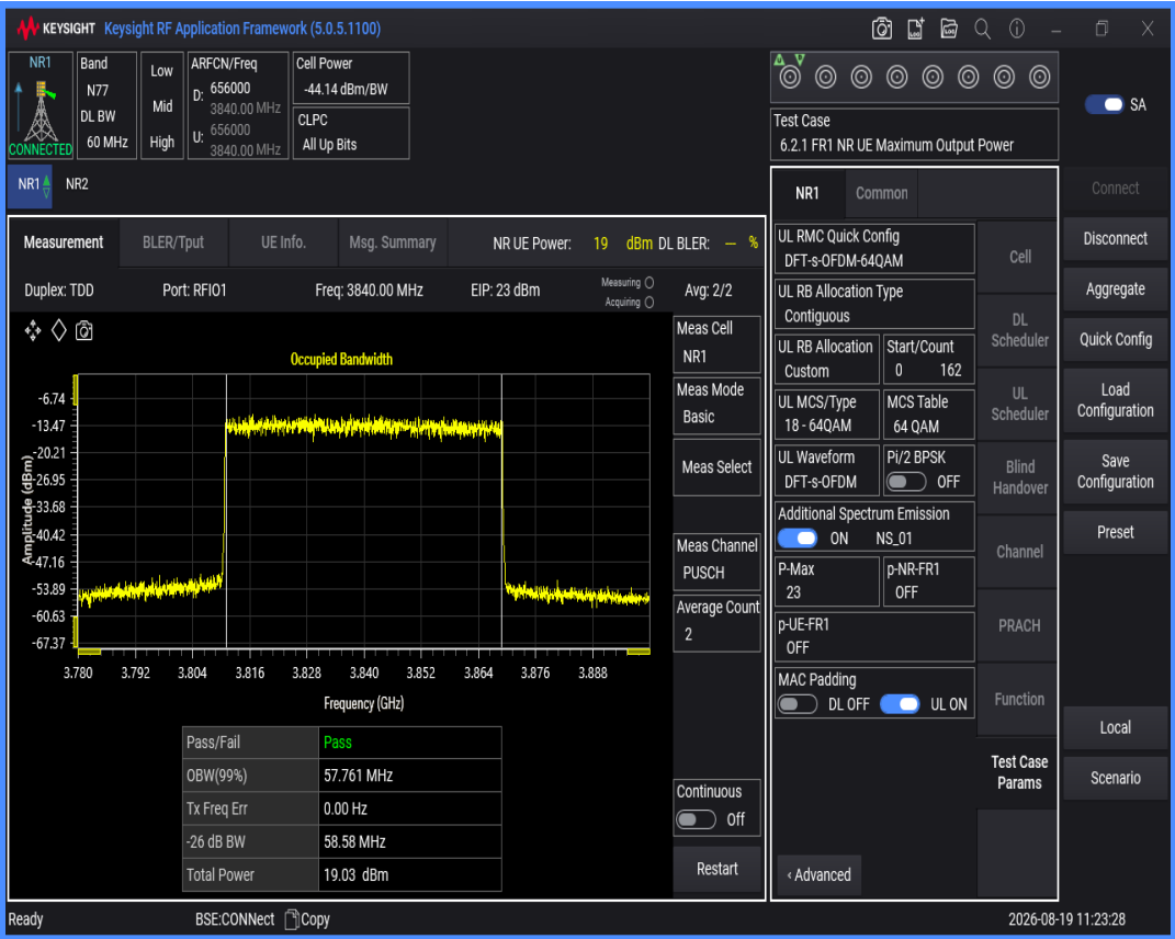
n77(3700-3980) SCS=30kHz DFT_QAM256 BW=60MHz Channel=656000 RB=162@0
