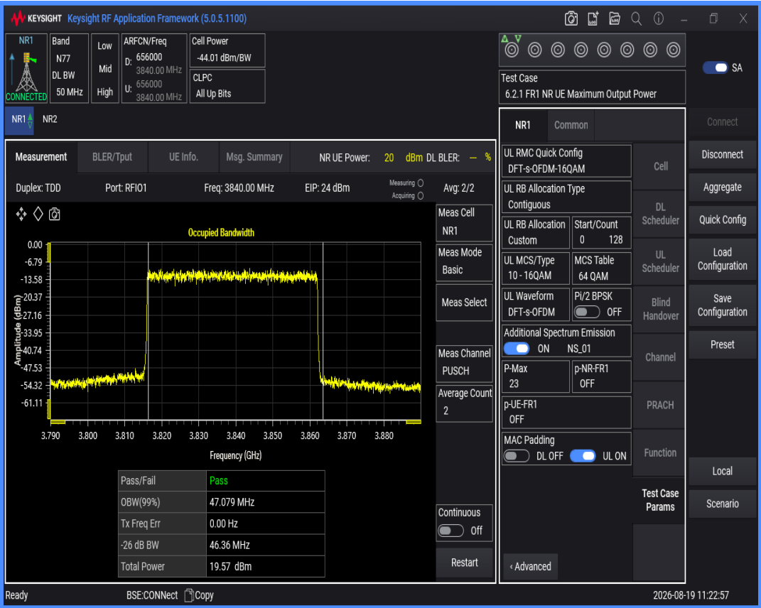
n77(3700-3980) SCS=30kHz DFT_QAM64 BW=50MHz Channel=656000 RB=128@0
