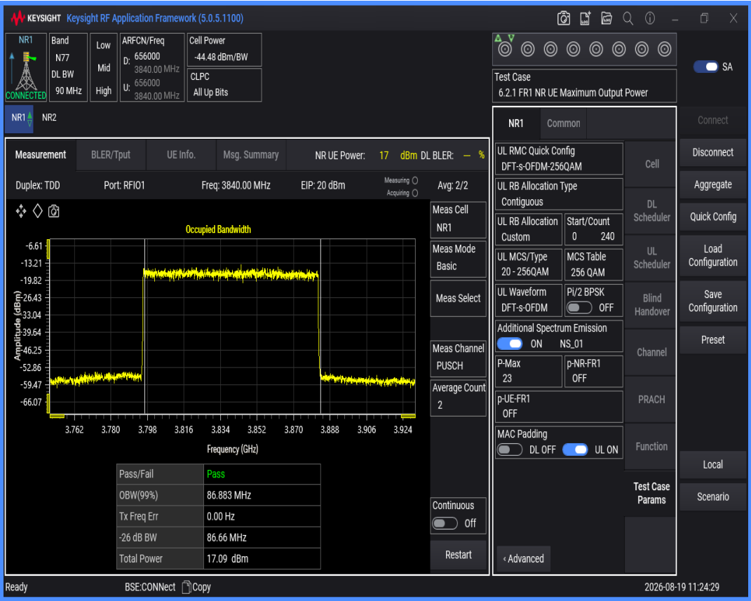
n77(3700-3980) SCS=30kHz DFT_BPSK BW=100MHz Channel=656000 RB=270@0
