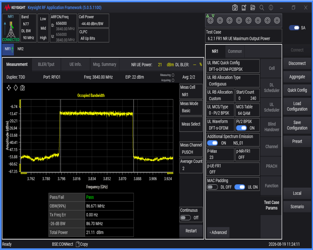
n77(3700-3980) SCS=30kHz DFT_QPSK BW=90MHz Channel=656000 RB=240@0
