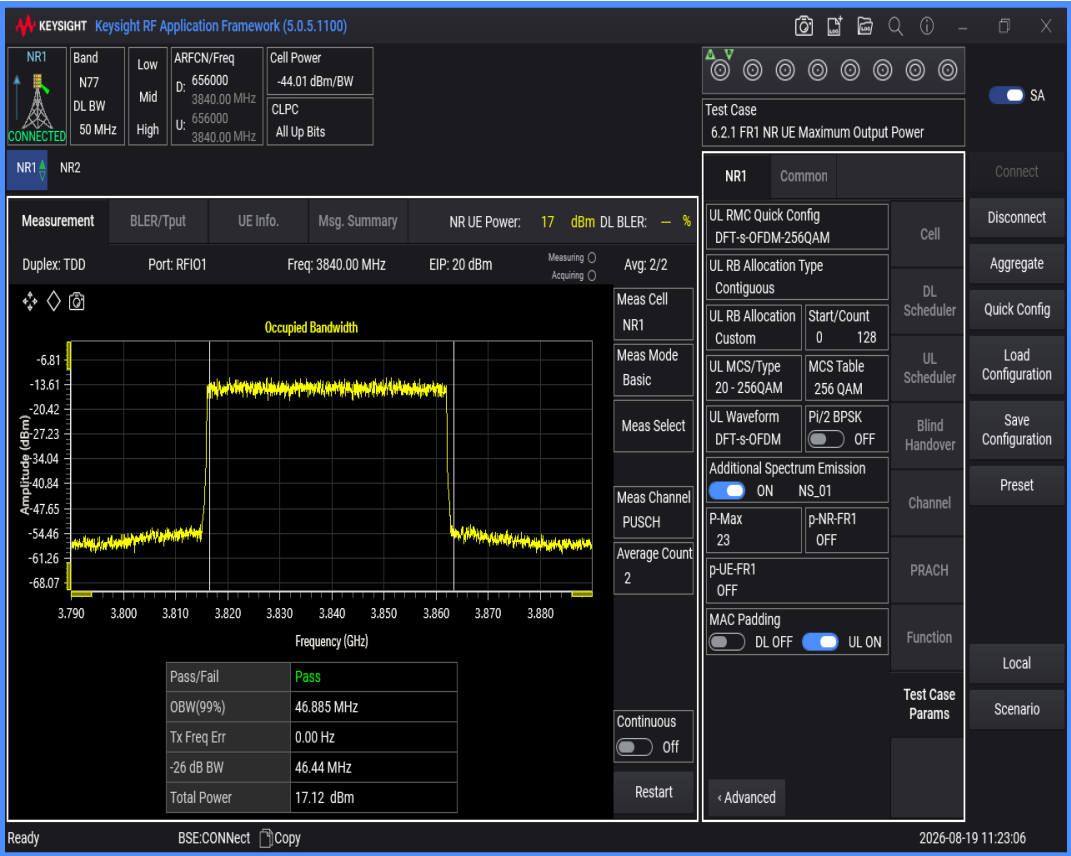
n77(3700-3980) SCS=30kHz DFT_BPSK BW=60MHz Channel=656000 RB=162@0
