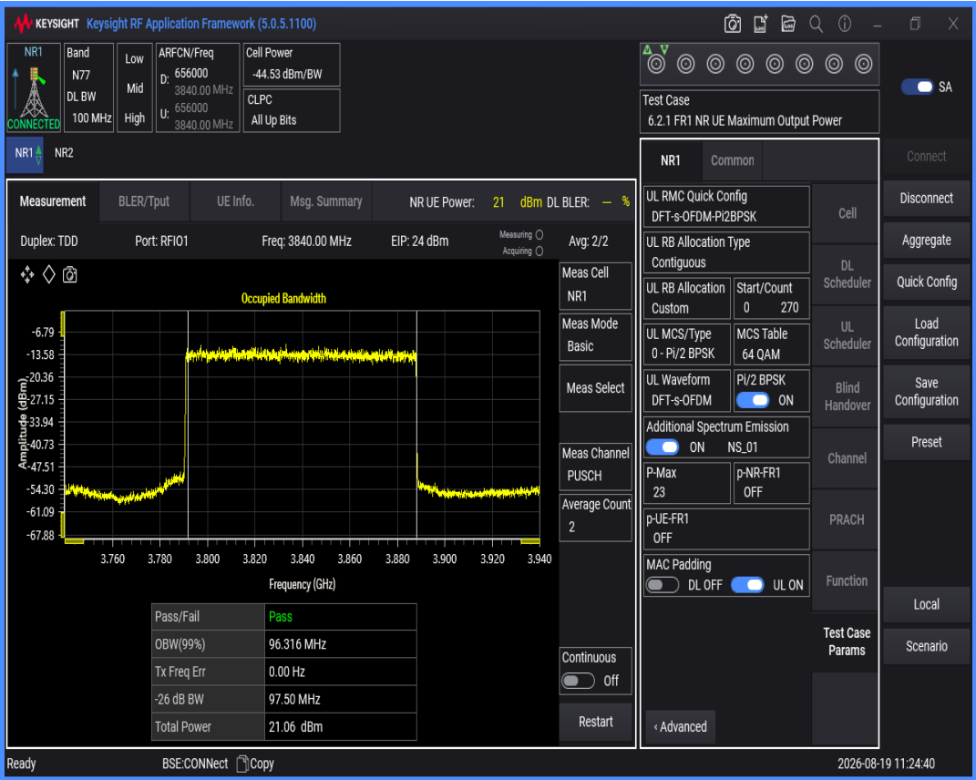
n77(3700-3980) SCS=30kHz DFT_QPSK BW=100MHz Channel=656000 RB=270@0
