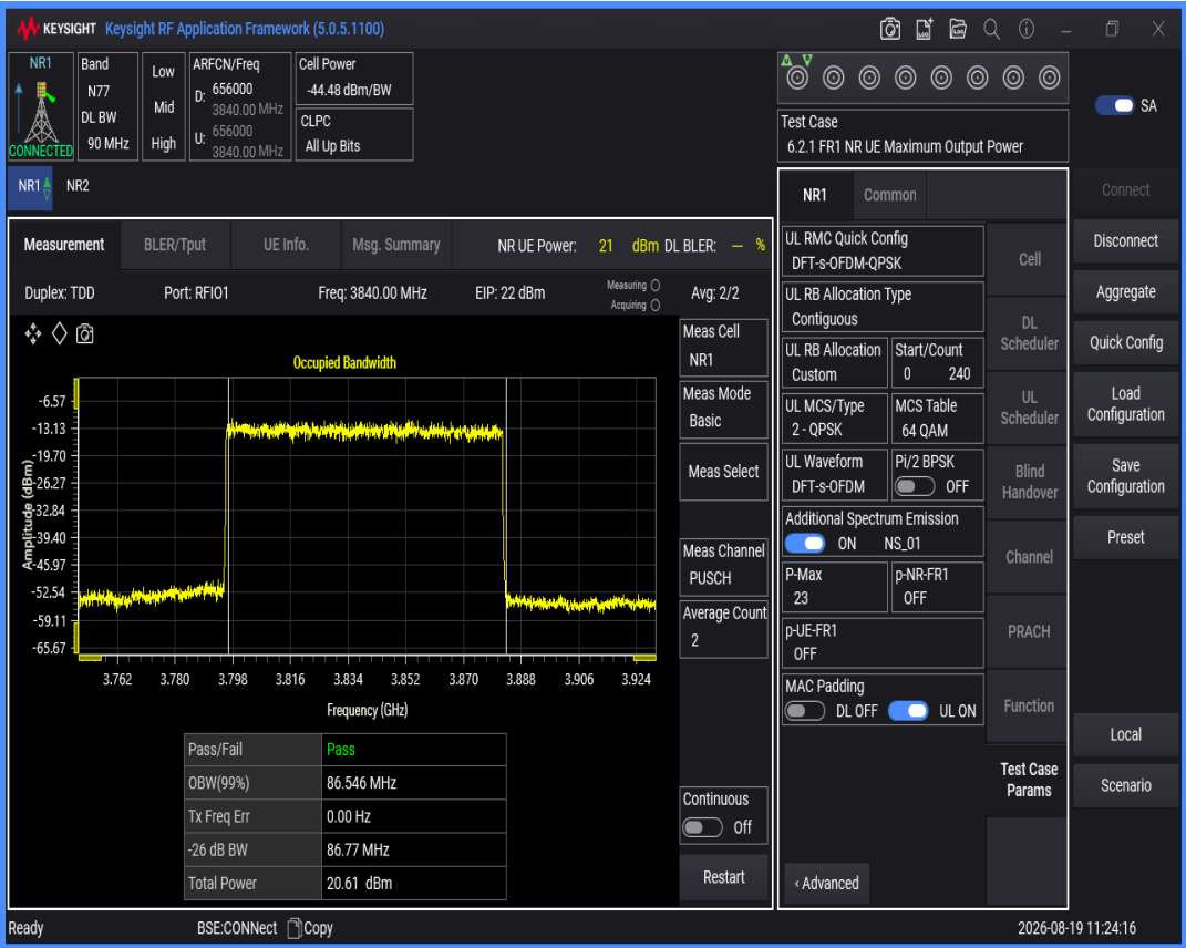
n77(3700-3980) SCS=30kHz DFT_QAM16 BW=90MHz Channel=656000 RB=240@0
