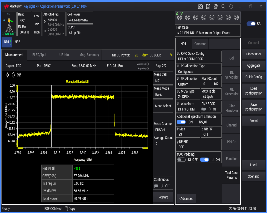
n77(3700-3980) SCS=30kHz DFT_QAM16 BW=60MHz Channel=656000 RB=162@0
