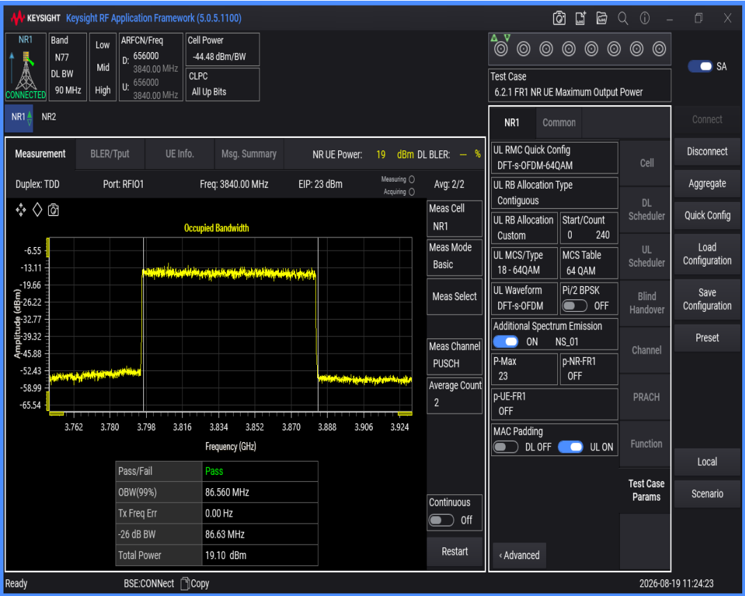
n77(3700-3980) SCS=30kHz DFT_QAM256 BW=90MHz Channel=656000 RB=240@0
