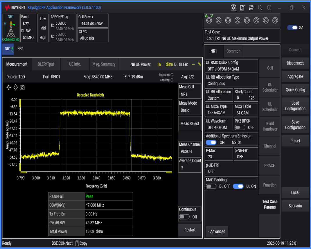
n77(3700-3980) SCS=30kHz DFT_QAM256 BW=50MHz Channel=656000 RB=128@0
