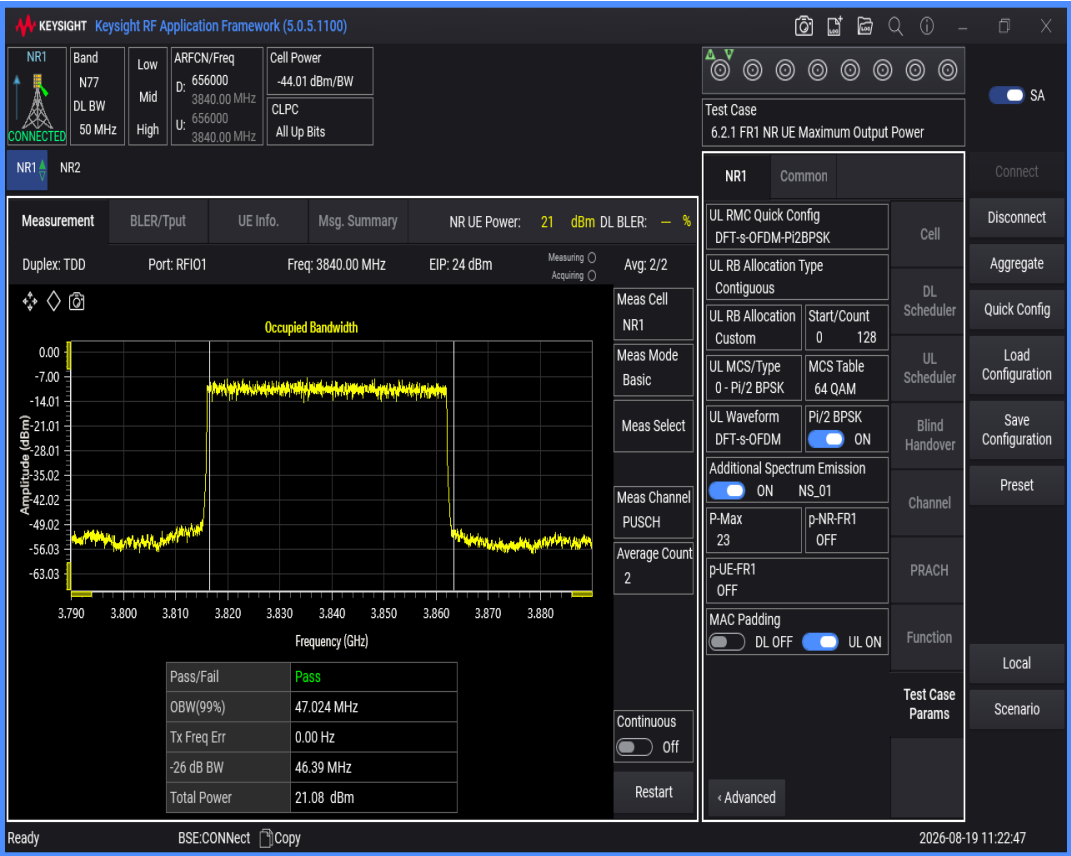
n77(3700-3980) SCS=30kHz DFT_QPSK BW=50MHz Channel=656000 RB=128@0
