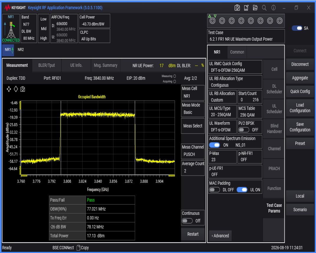
n77(3700-3980) SCS=30kHz DFT_BPSK BW=90MHz Channel=656000 RB=240@0
