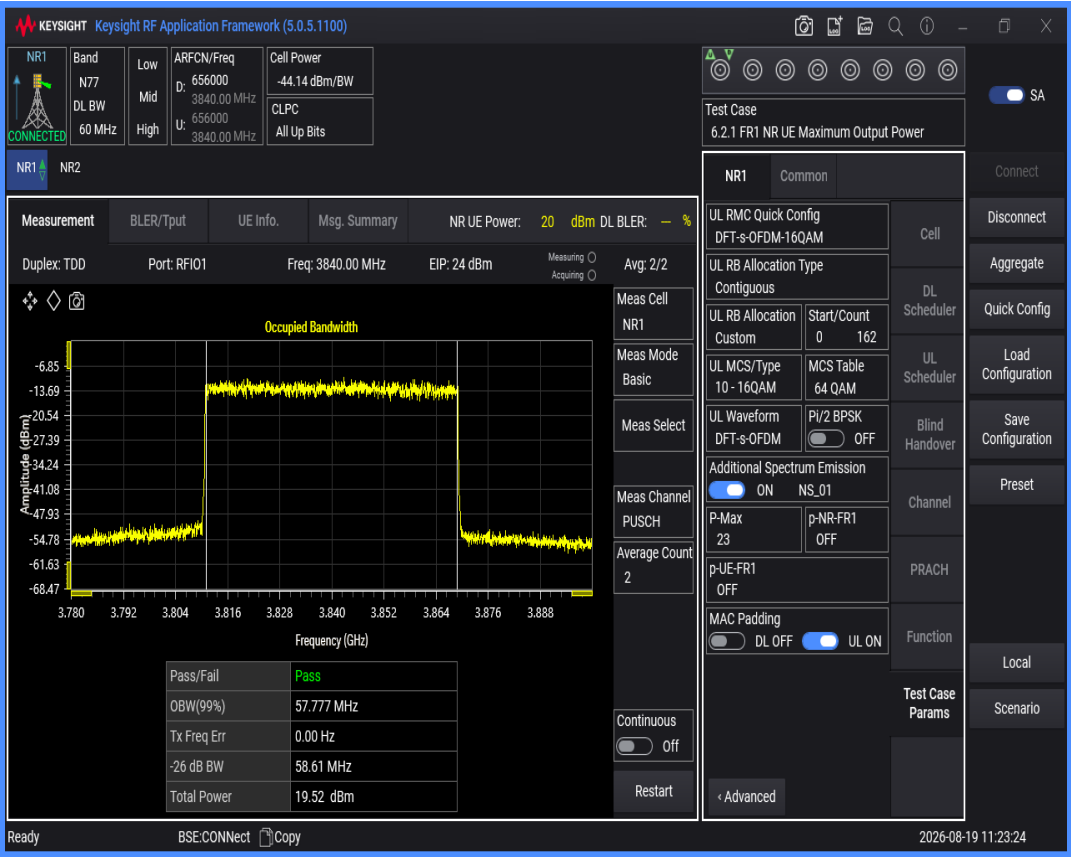
n77(3700-3980) SCS=30kHz DFT_QAM64 BW=60MHz Channel=656000 RB=162@0
