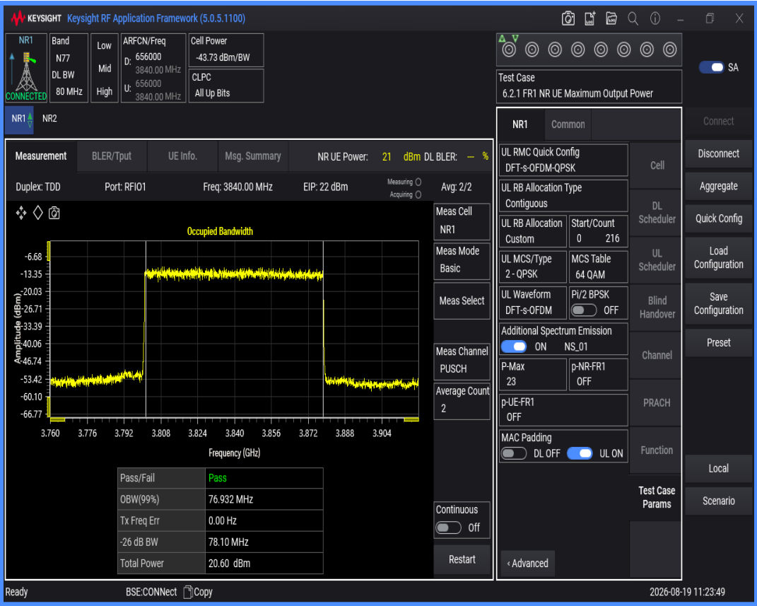
n77(3700-3980) SCS=30kHz DFT_QAM16 BW=80MHz Channel=656000 RB=216@0
