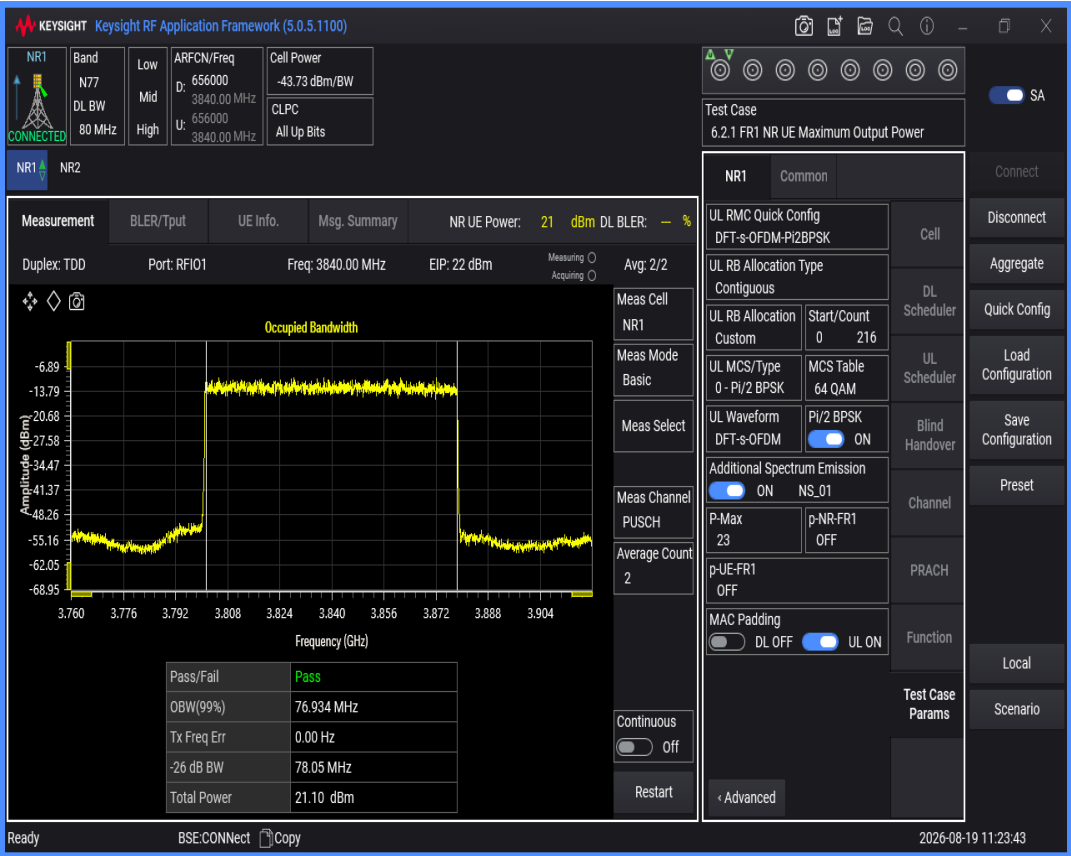
n77(3700-3980) SCS=30kHz DFT_QPSK BW=80MHz Channel=656000 RB=216@0
