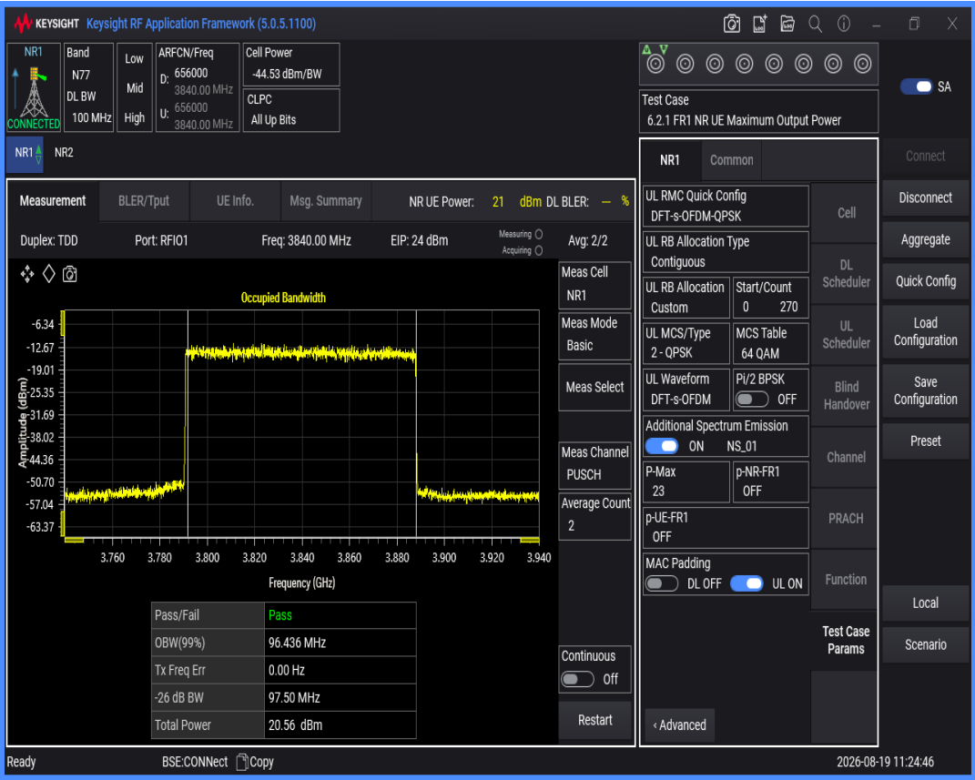
n77(3700-3980) SCS=30kHz DFT_QAM16 BW=100MHz Channel=656000 RB=270@0
