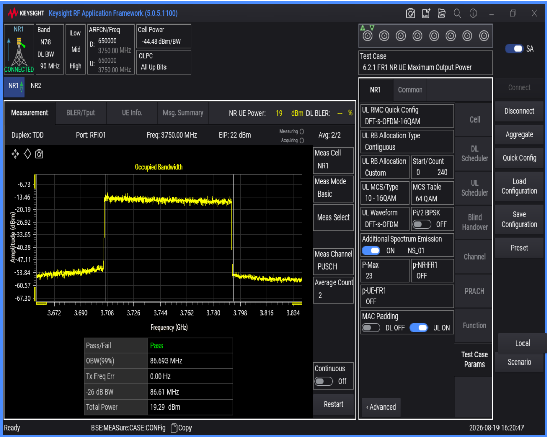
n78(3700-3800) SCS=30kHz DFT_QAM64 BW=90MHz Channel=650000 RB=240@0
