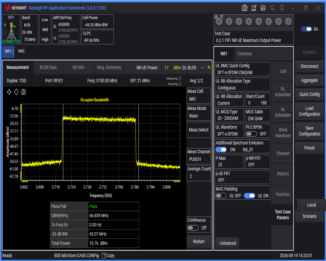
n78(3700-3800) SCS=30kHz DFT_BPSK BW=80MHz Channel=650000 RB=216@0
