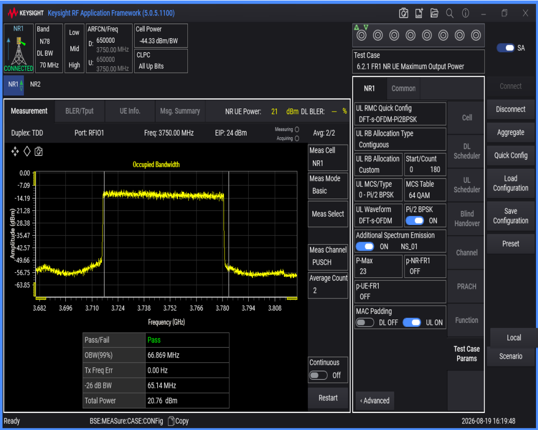
n78(3700-3800) SCS=30kHz DFT_QPSK BW=70MHz Channel=650000 RB=
