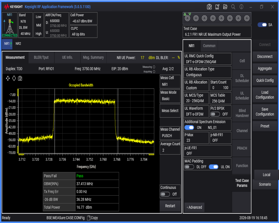
n78(3700-3800) SCS=30kHz DFT_BPSK BW=50MHz Channel=650000 RB=128@0
