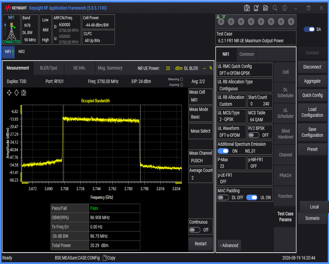
n78(3700-3800) SCS=30kHz DFT_QAM16 BW=90MHz Channel=650000 RB=240@0
