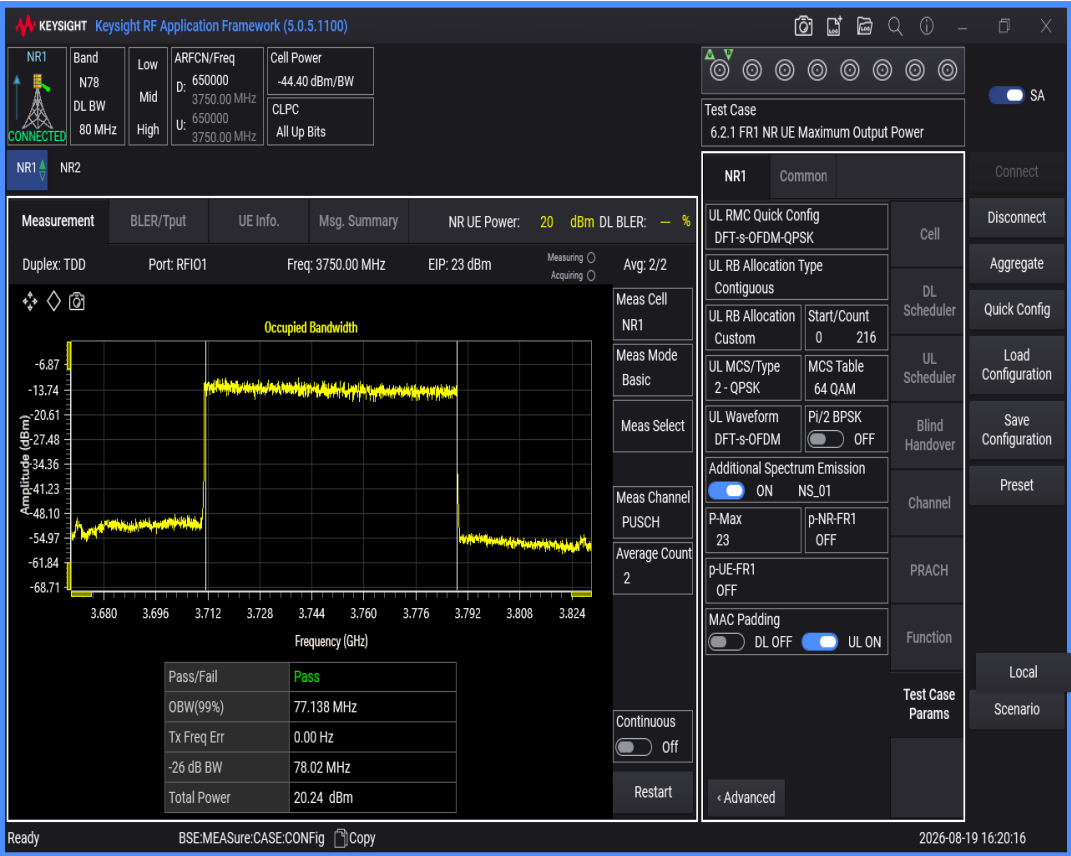
n78(3700-3800) SCS=30kHz DFT_QAM16 BW=80MHz Channel=650000 RB=216@0
