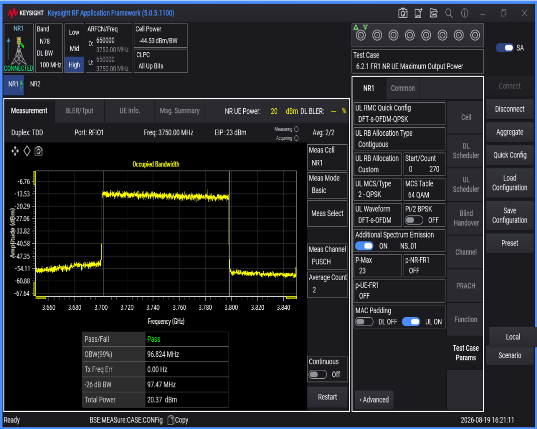
n78(3700-3800) SCS=30kHz DFT_QAM16 BW=100MHz Channel=650000 RB=270@0
