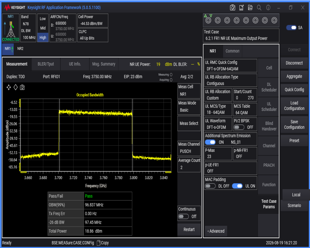
n78(3700-3800) SCS=30kHz DFT_QAM256 BW=100MHz Channel=650000 RB=270@0
