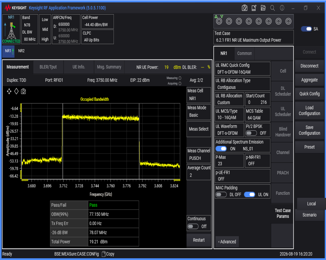
n78(3700-3800) SCS=30kHz DFT_QAM64 BW=80MHz Channel=650000 RB=216@0
