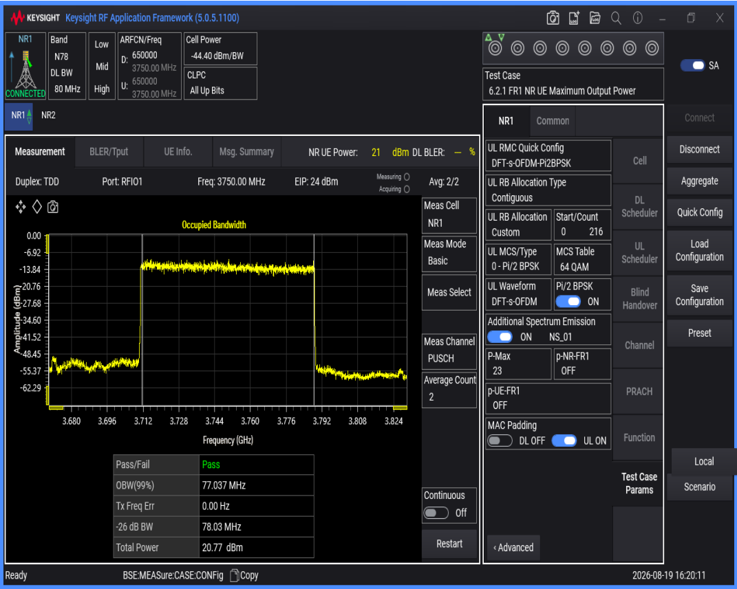
n78(3700-3800) SCS=30kHz DFT_QPSK BW=80MHz Channel=650000 RB=216@0
