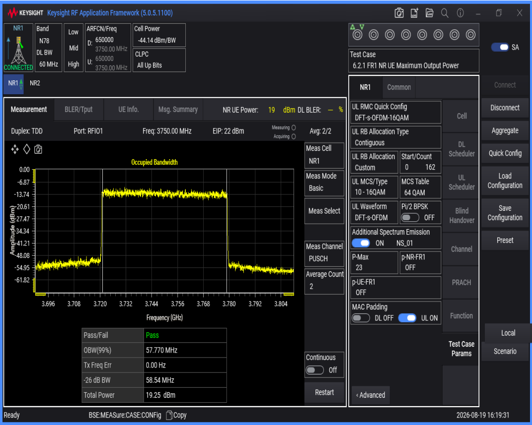
n78(3700-3800) SCS=30kHz DFT_QAM64 BW=60MHz Channel=650000 RB=162@0
