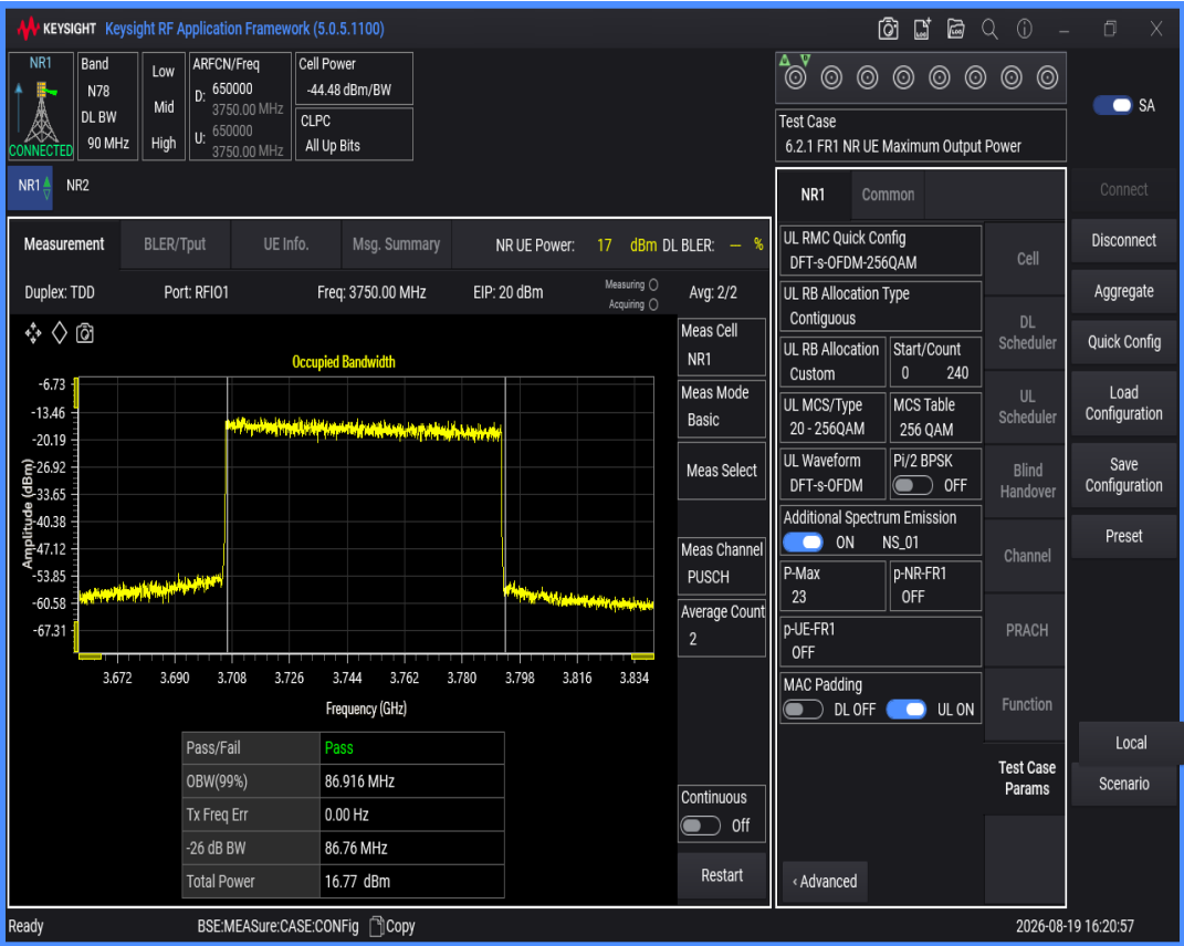
n78(3700-3800) SCS=30kHz DFT_BPSK BW=100MHz Channel=650000 RB=270@0
