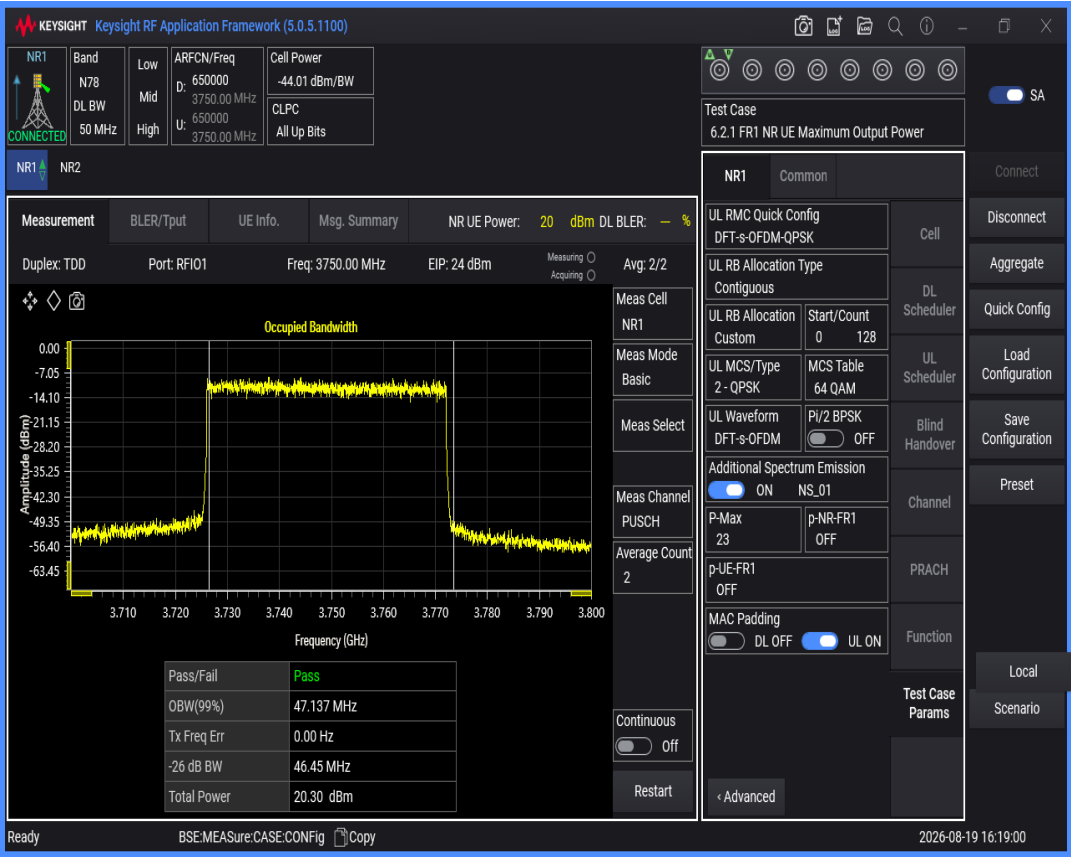
n78(3700-3800) SCS=30kHz DFT_QAM16 BW=50MHz Channel=650000 RB=128@0
