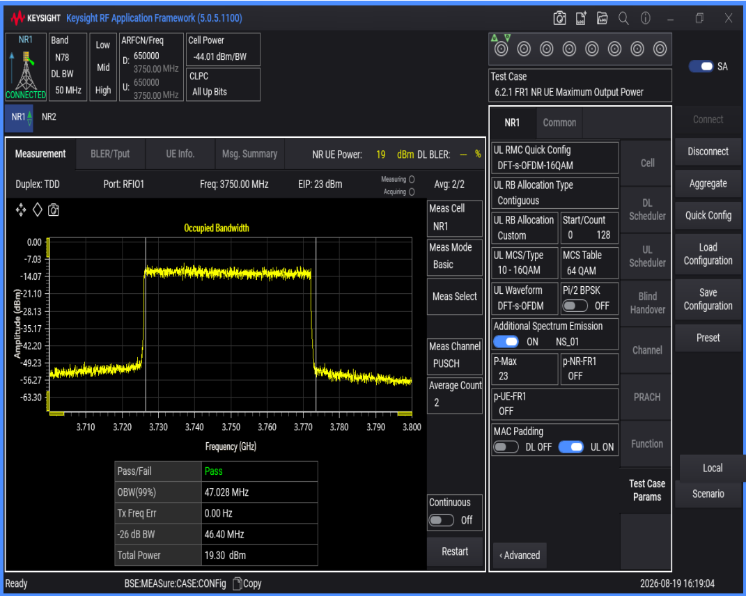
n78(3700-3800) SCS=30kHz DFT_QAM64 BW=50MHz Channel=650000 RB=128@0
