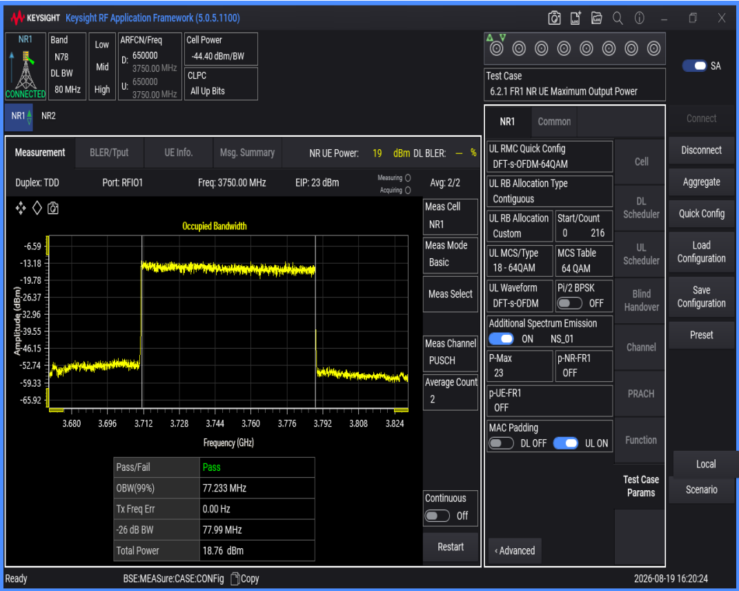
n78(3700-3800) SCS=30kHz DFT_QAM256 BW=80MHz Channel=650000 RB=216@0
