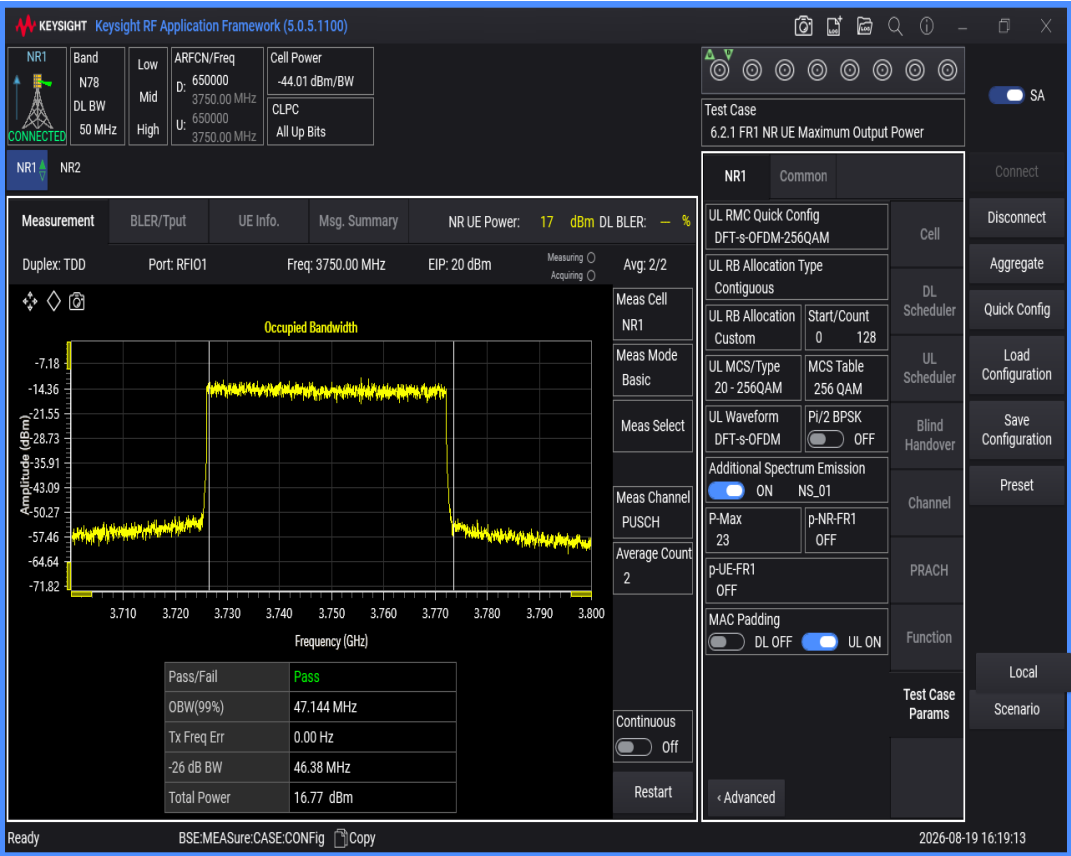
n78(3700-3800) SCS=30kHz DFT_BPSK BW=60MHz Channel=650000 RB=162@0
