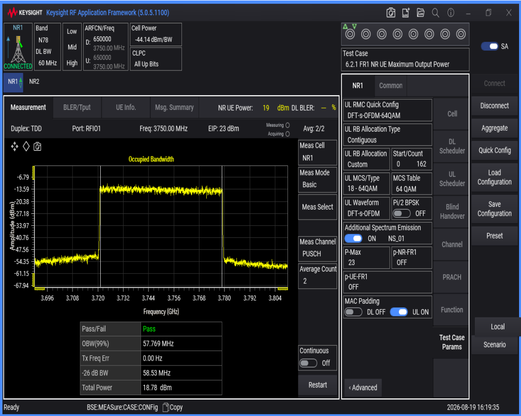
n78(3700-3800) SCS=30kHz DFT_QAM256 BW=60MHz Channel=650000 RB=162@0
