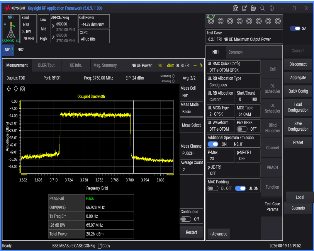
n78(3700-3800) SCS=30kHz DFT_QAM16 BW=70MHz Channel=650000 RB=
