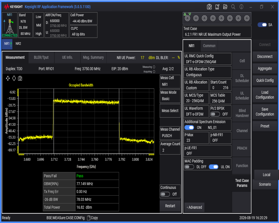
n78(3700-3800) SCS=30kHz DFT_BPSK BW=90MHz Channel=650000 RB=240@0
