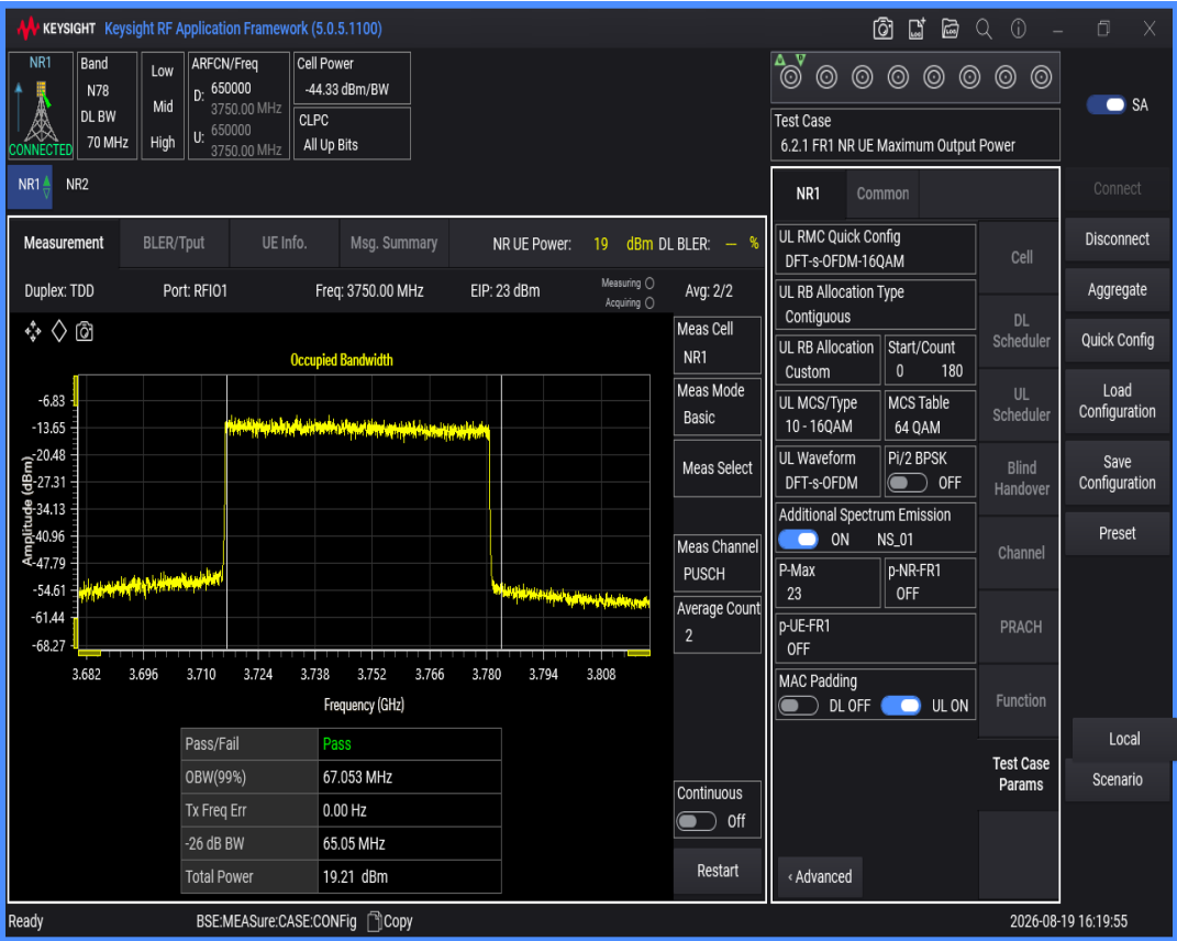
n78(3700-3800) SCS=30kHz DFT_QAM64 BW=70MHz Channel=650000 RB=
