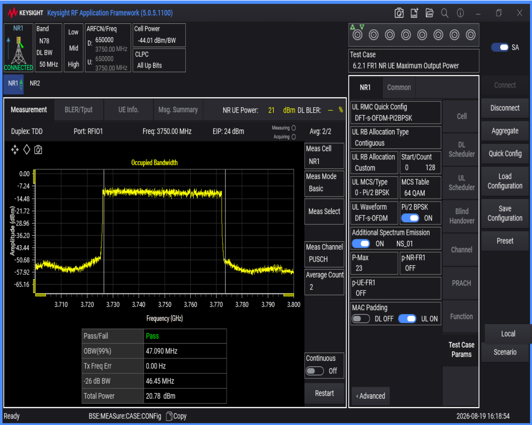
n78(3700-3800) SCS=30kHz DFT_QPSK BW=50MHz Channel=650000 RB=128@0
