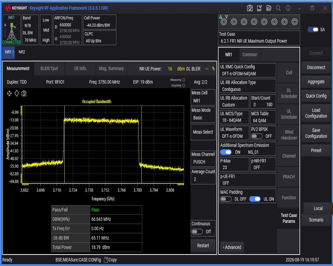
n78(3700-3800) SCS=30kHz DFT_QAM256 BW=70MHz Channel=650000 RB=
