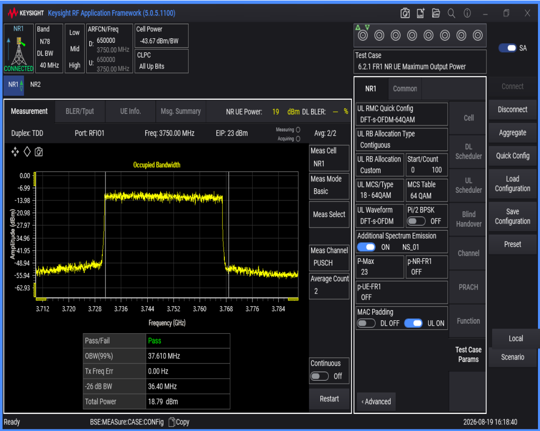
n78(3700-3800) SCS=30kHz DFT_QAM256 BW=40MHz Channel=650000 RB=100@0
