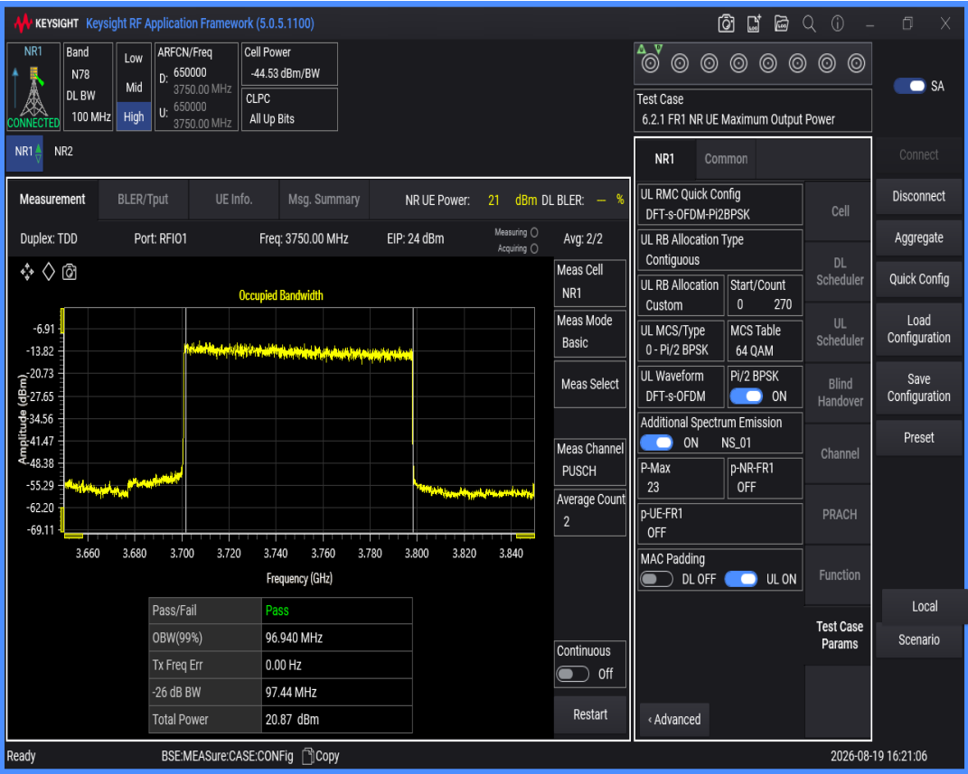
n78(3700-3800) SCS=30kHz DFT_QPSK BW=100MHz Channel=650000 RB=270@0
