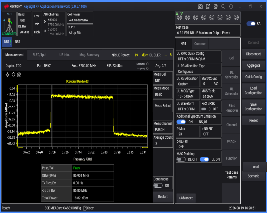
n78(3700-3800) SCS=30kHz DFT_QAM256 BW=90MHz Channel=650000 RB=240@0
