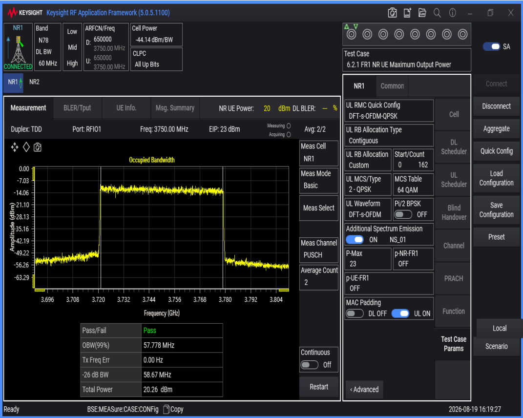
n78(3700-3800) SCS=30kHz DFT_QAM16 BW=60MHz Channel=650000 RB=162@0
