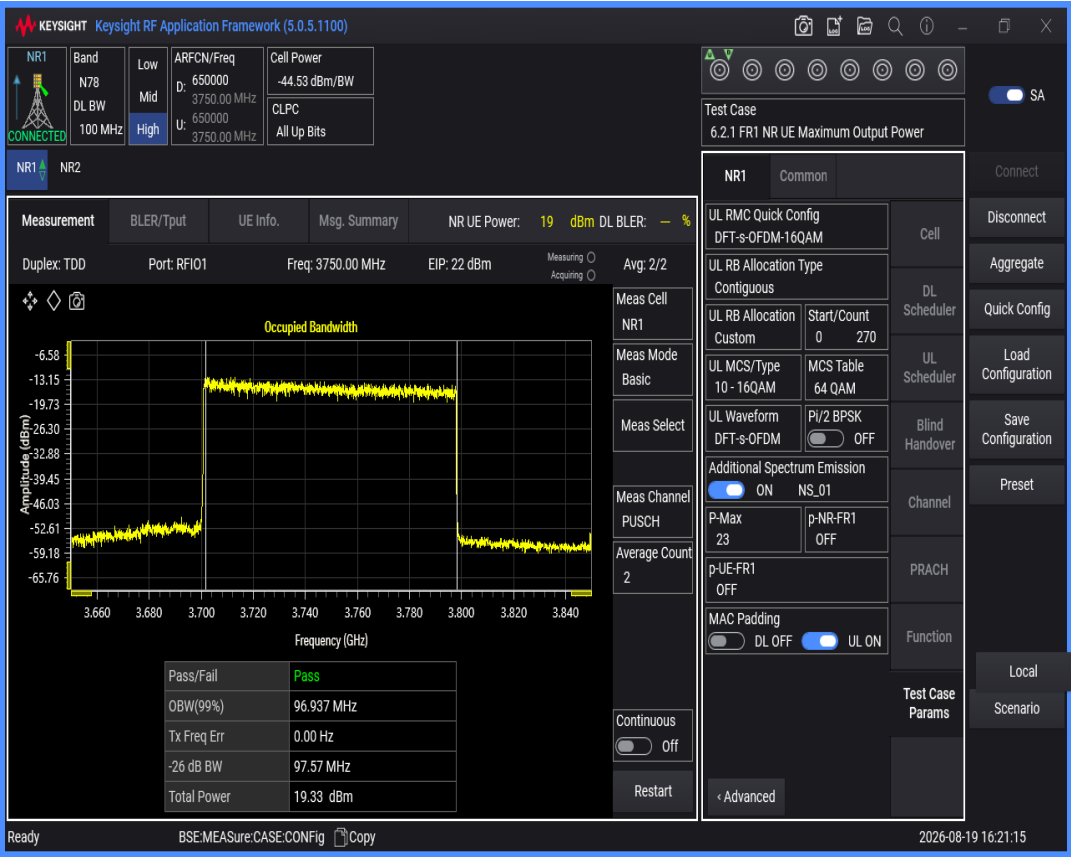
n78(3700-3800) SCS=30kHz DFT_QAM64 BW=100MHz Channel=650000 RB=270@0
