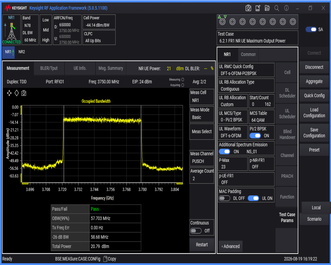
n78(3700-3800) SCS=30kHz DFT_QPSK BW=60MHz Channel=650000 RB=162@0
