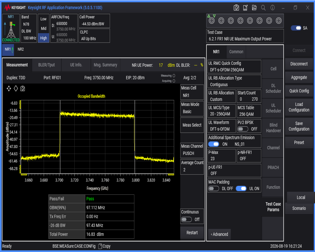
n78(3700-3800) SCS=30kHz DFT_QAM256 BW=100MHz Channel=650000 RB=270@0
