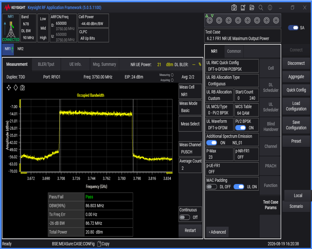
n78(3700-3800) SCS=30kHz DFT_QPSK BW=90MHz Channel=650000 RB=240@0
