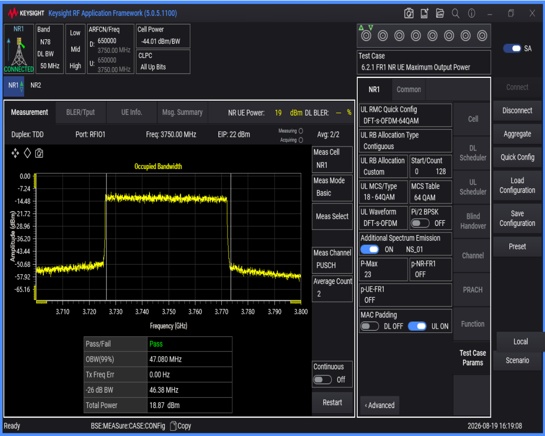
n78(3700-3800) SCS=30kHz DFT_QAM256 BW=50MHz Channel=650000 RB=128@0
