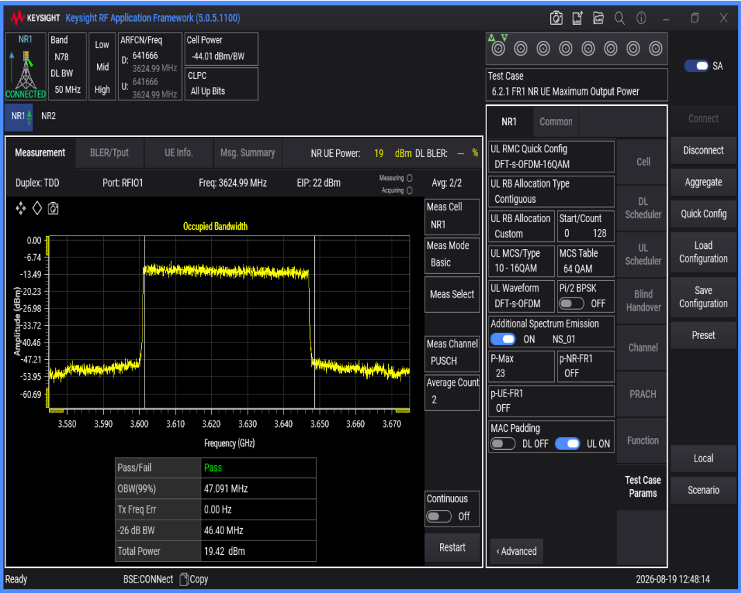
n78(3550-3700) SCS=30kHz DFT_QAM64 BW=50MHz Channel=641666 RB=128@0
