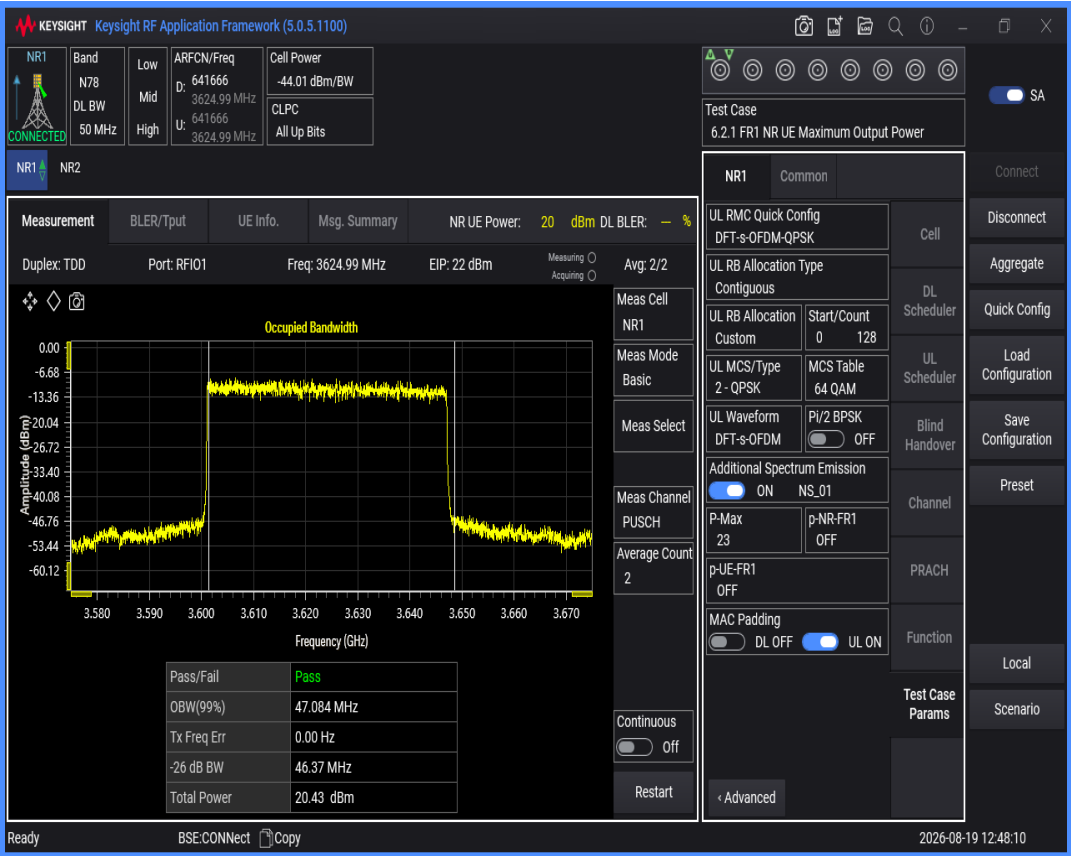
n78(3550-3700) SCS=30kHz DFT_QAM16 BW=50MHz Channel=641666 RB=128@0
