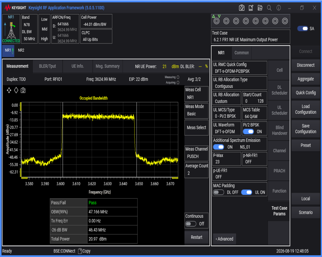
n78(3550-3700) SCS=30kHz DFT_QPSK BW=50MHz Channel=641666 RB=128@0
