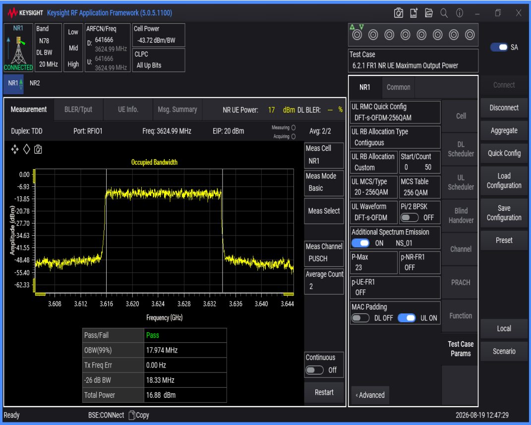
n78(3550-3700) SCS=30kHz DFT_BPSK BW=40MHz Channel=641666 RB=100@0
