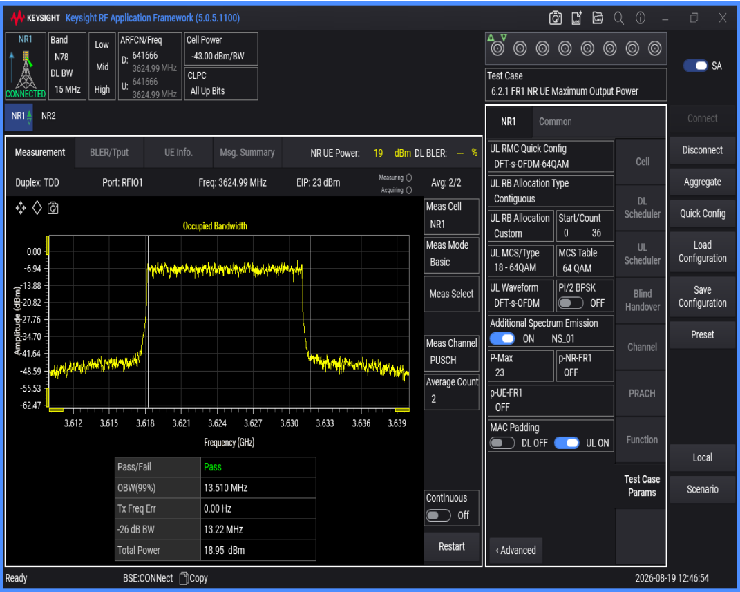
n78(3550-3700) SCS=30kHz DFT_QAM256 BW=15MHz Channel=641666 RB=36@0
