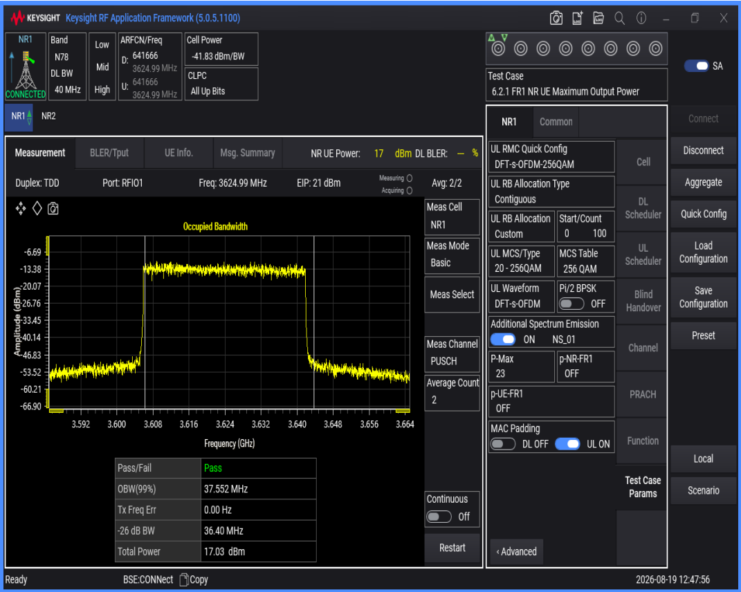
n78(3550-3700) SCS=30kHz DFT_BPSK BW=50MHz Channel=641666 RB=128@0
