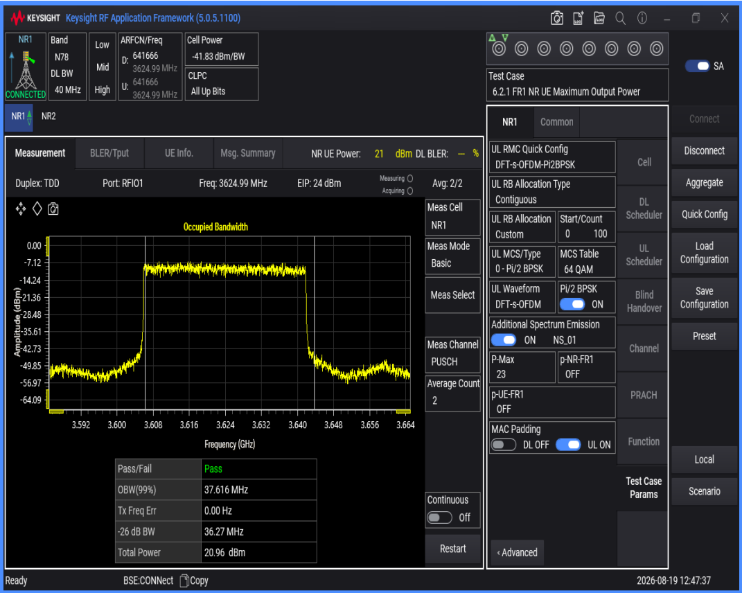
n78(3550-3700) SCS=30kHz DFT_QPSK BW=40MHz Channel=641666 RB=100@0
