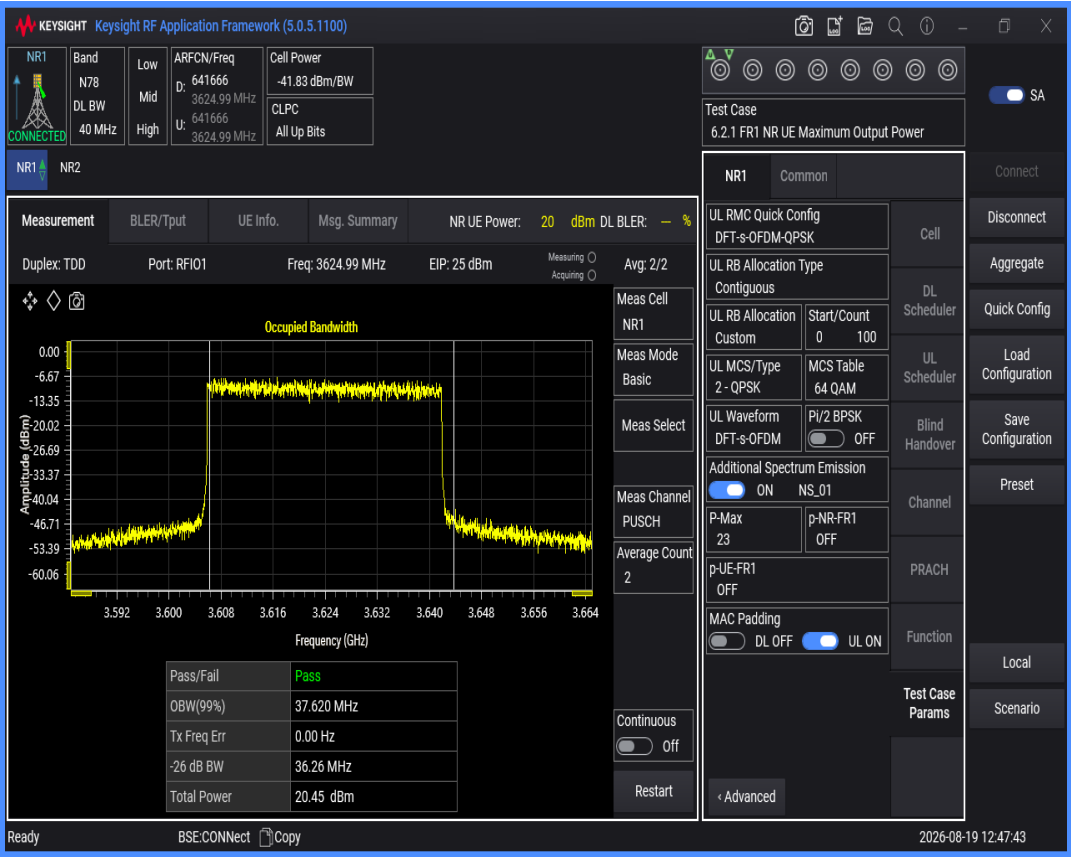
n78(3550-3700) SCS=30kHz DFT_QAM16 BW=40MHz Channel=641666 RB=100@0
