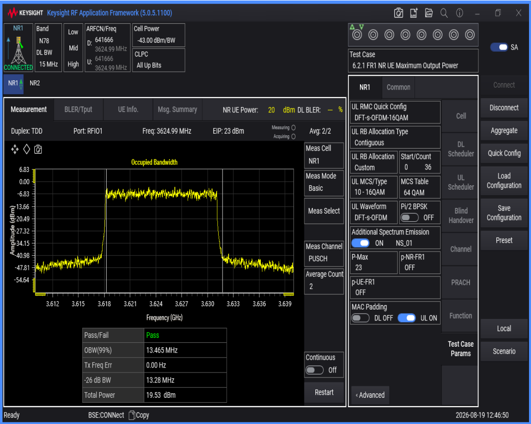
n78(3550-3700) SCS=30kHz DFT_QAM64 BW=15MHz Channel=641666 RB=36@0
