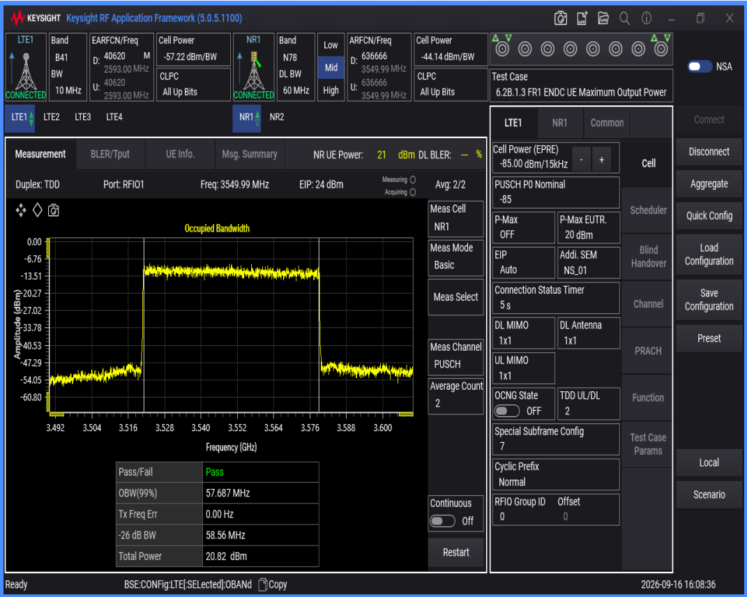
n78 SCS=30kHz DFT_QAM64 BW=80MHz Channel=636666 RB=216@0
