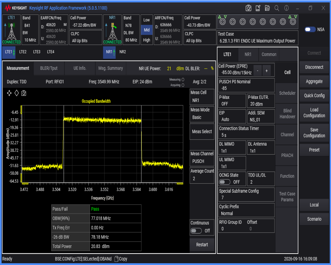
n78 SCS=30kHz DFT_QAM64 BW=90MHz Channel=636666 RB=240@0
