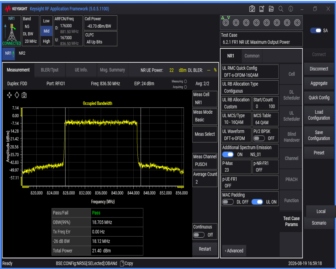
n5 SCS=15kHz DFT_QAM64 BW=20MHz Channel=167300 RB=100@0
