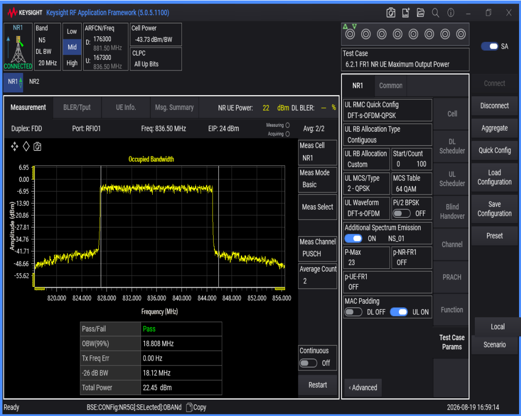
n5 SCS=15kHz DFT_QAM16 BW=20MHz Channel=167300 RB=100@0
