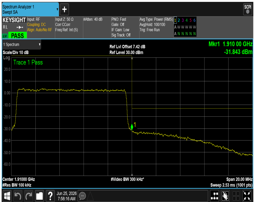
Band2 QPSK BW=15MHz Channel=18675 RB Size=75 Position=#0
