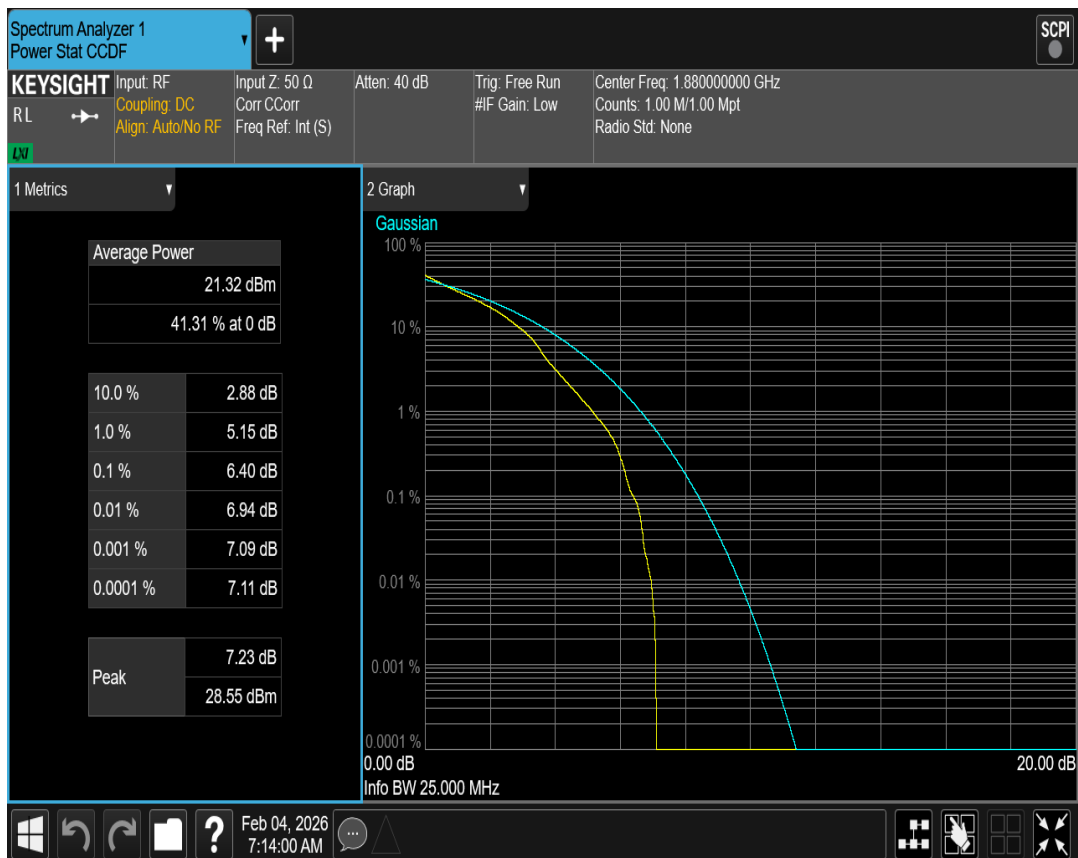
Band2 QPSK BW=10MHz Channel=18900 RB Size=1 Position=#0
