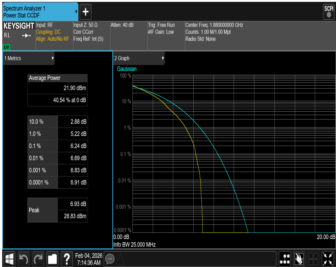
Band2 QPSK BW=3MHz Channel=18900 RB Size=1 Position=#0
