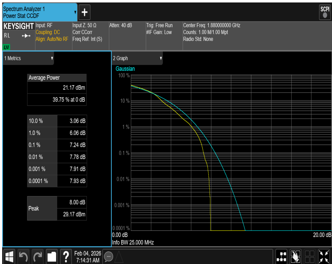
Band2 QAM16 BW=20MHz Channel=18900 RB Size=1 Position=#0
