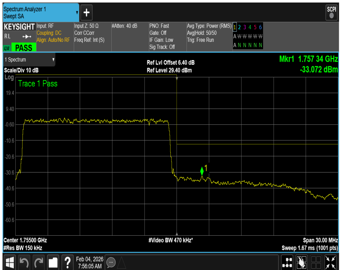
Band4 QPSK BW=20MHz Channel=20050 RB Size=100 Position=#0
