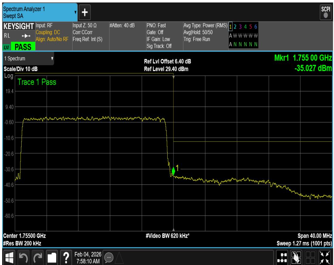
Band4 QPSK BW=3MHz Channel=19965 RB Size=15 Position=#0
