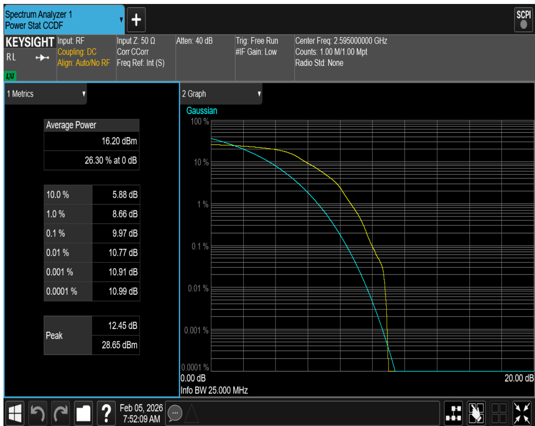
Band41(2535-2655) QPSK BW=5MHz Channel=40640 RB Size=1 Position=#0
