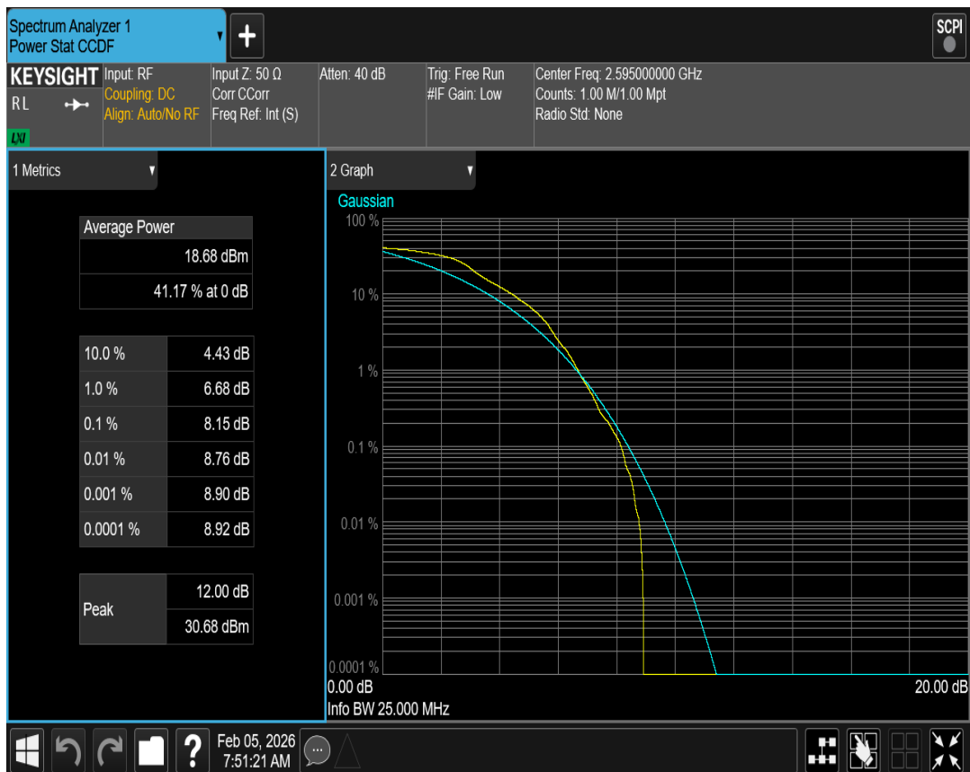
Band41(2535-2655) QPSK BW=15MHz Channel=40640 RB Size=1 Position=#0
