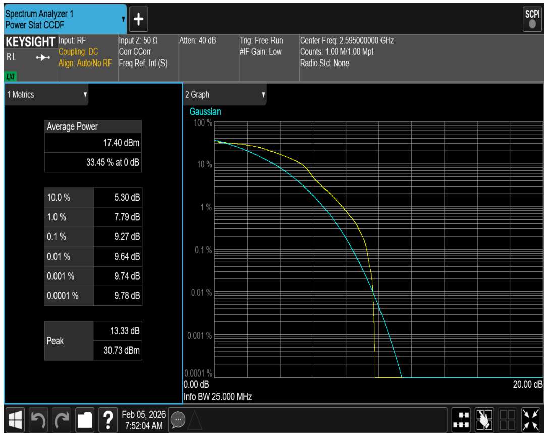
Band41(2535-2655) QAM16 BW=20MHz Channel=40640 RB Size=1 Position=#0
