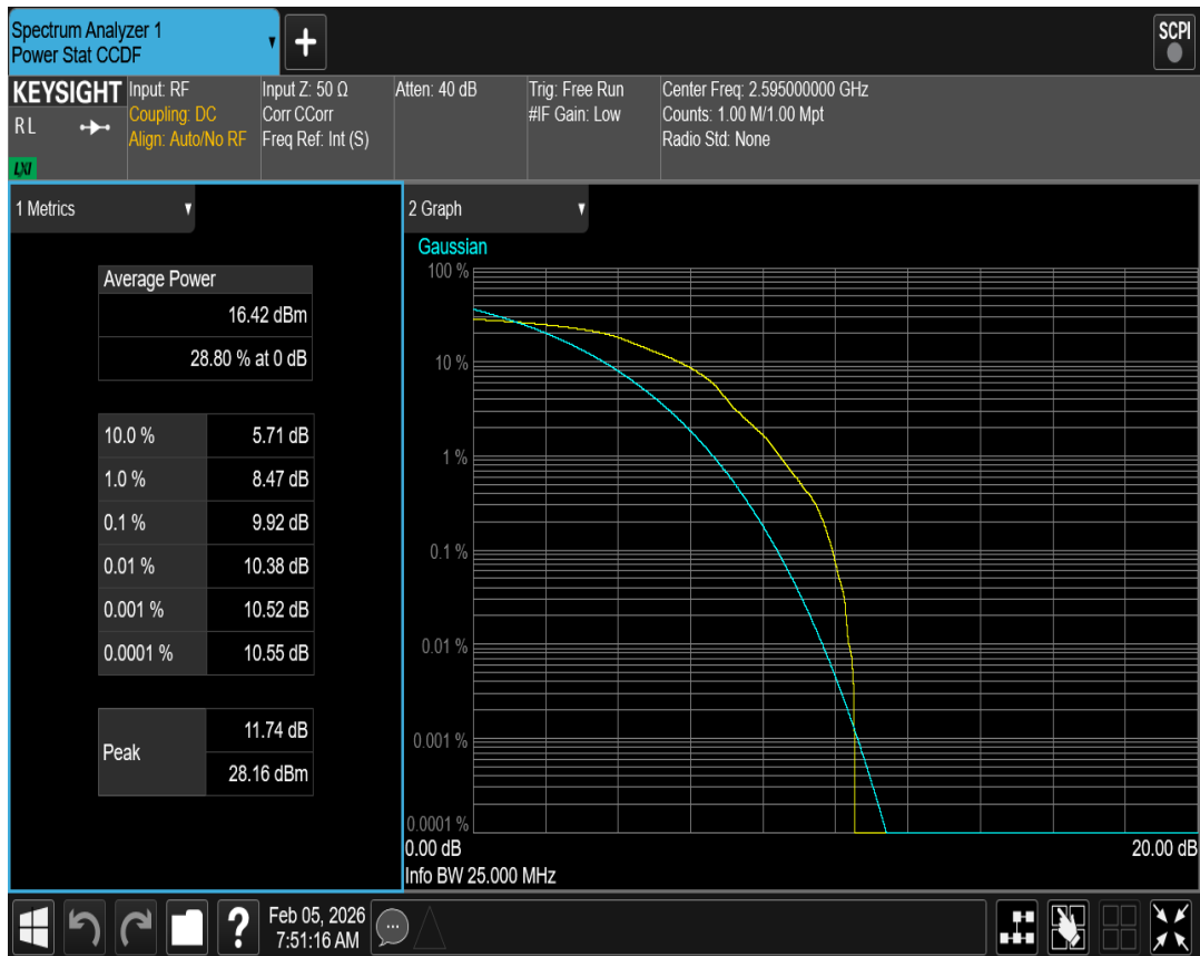
Band41(2535-2655) QPSK BW=10MHz Channel=40640 RB Size=1 Position=#0
