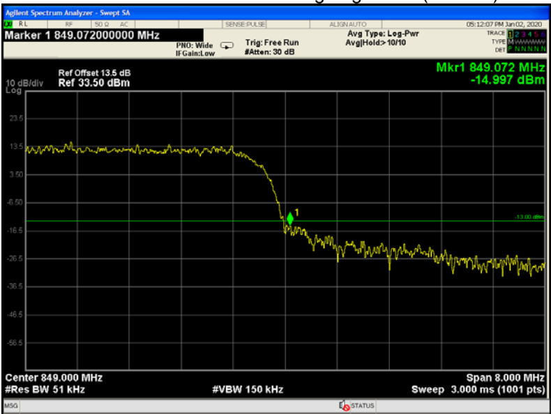
WCDMA band V band edge-right side (HSUPA)
