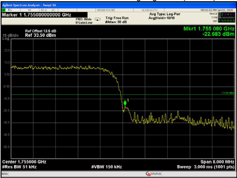
WCDMA band IV band edge-right side (HSUPA)
