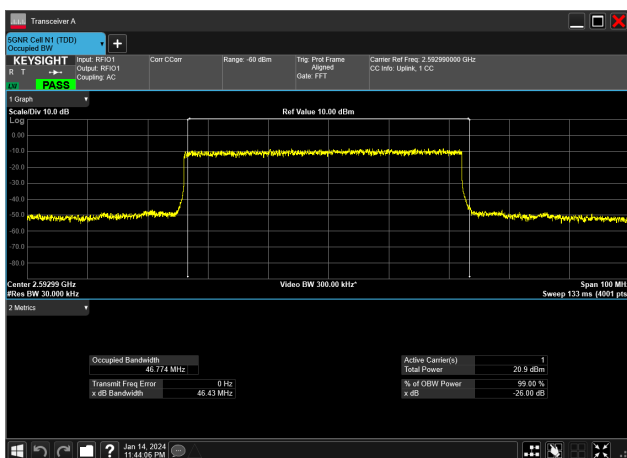
50MHz_30kHz_2592.99MHz_DFT-s-OFDM 16 QAM_RB128@0&amp;46.774 MHz
