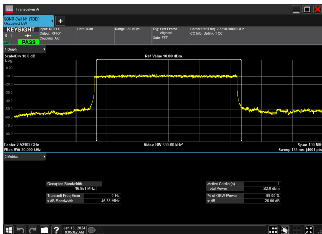
50MHz_30kHz_2521.02MHz_DFT-s-OFDM PI/2 BPSK_RB128@0&amp;46.951 MHz
