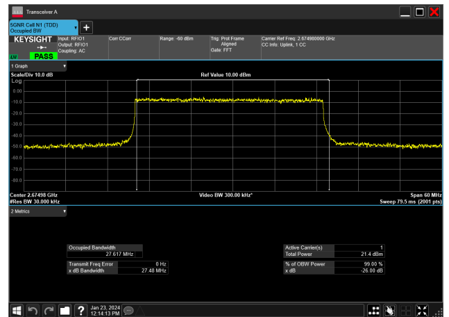
30MHz_30kHz_2674.98MHz_DFT-s-OFDM 16 QAM_RB75@0&amp;27.617 MHz
