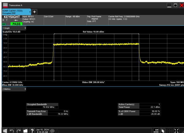
80MHz_30kHz_2536.02MHz_DFT-s-OFDM PI/2 BPSK_RB216@0&amp;76.932 MHz
