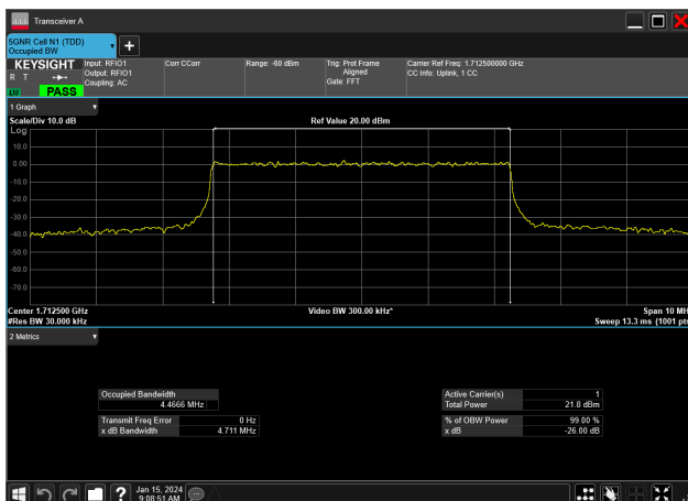
5MHz_15kHz_1712.5MHz_DFT-s-OFDM 16 QAM_RB25@0&amp;4.467 MHz
