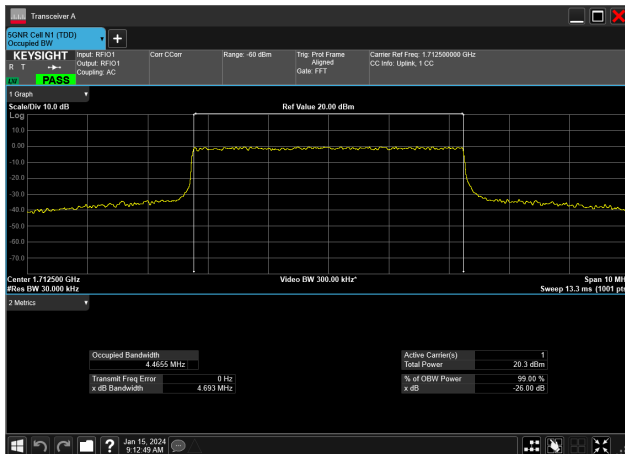
5MHz_15kHz_1712.5MHz_CP-OFDM 64 QAM_RB25@0&amp;4.466 MHz
