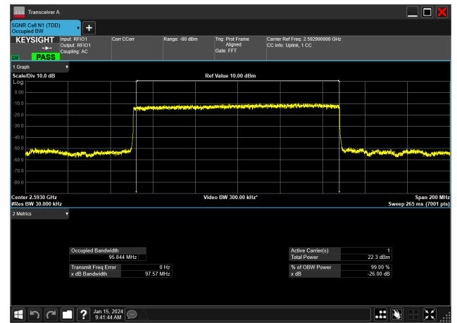
100MHz_30kHz_2592.99MHz_DFT-s-OFDM PI/2 BPSK_RB270@0&95.844 MHz
