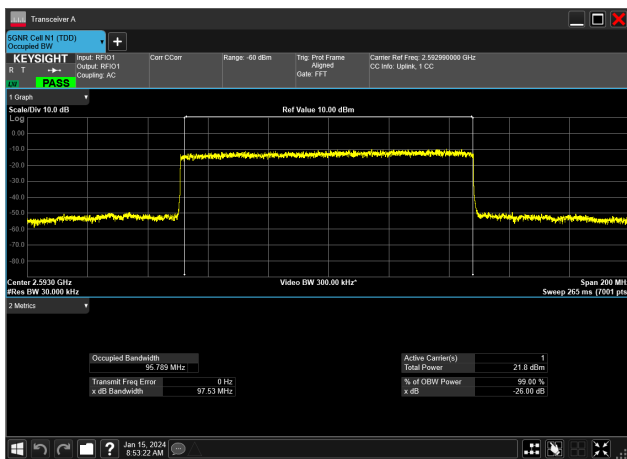
100MHz_30kHz_2592.99MHz_DFT-s-OFDM QPSK_RB270@0&95.789 MHz
