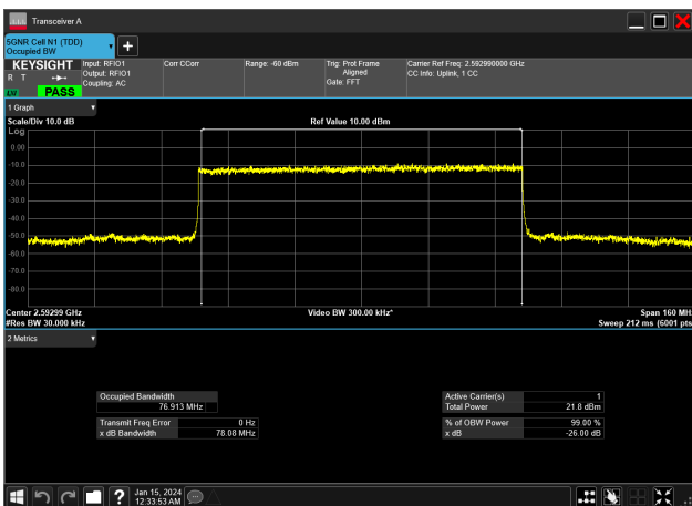
80MHz_30kHz_2592.99MHz_DFT-s-OFDM QPSK_RB216@0&76.913 MHz
