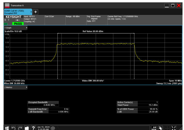
5MHz_15kHz_1712.5MHz_DFT-s-OFDM 256 QAM_RB25@0&amp;4.465 MHz
