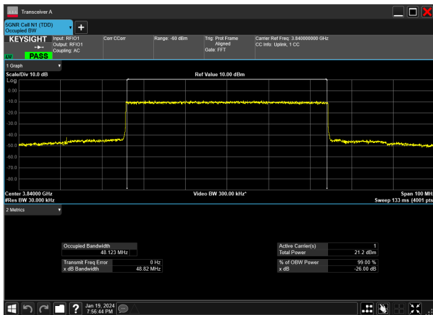
50MHz_15kHz_3840MHz_DFT-s-OFDM 64 QAM_RB270@0&amp;48.123 MHz
