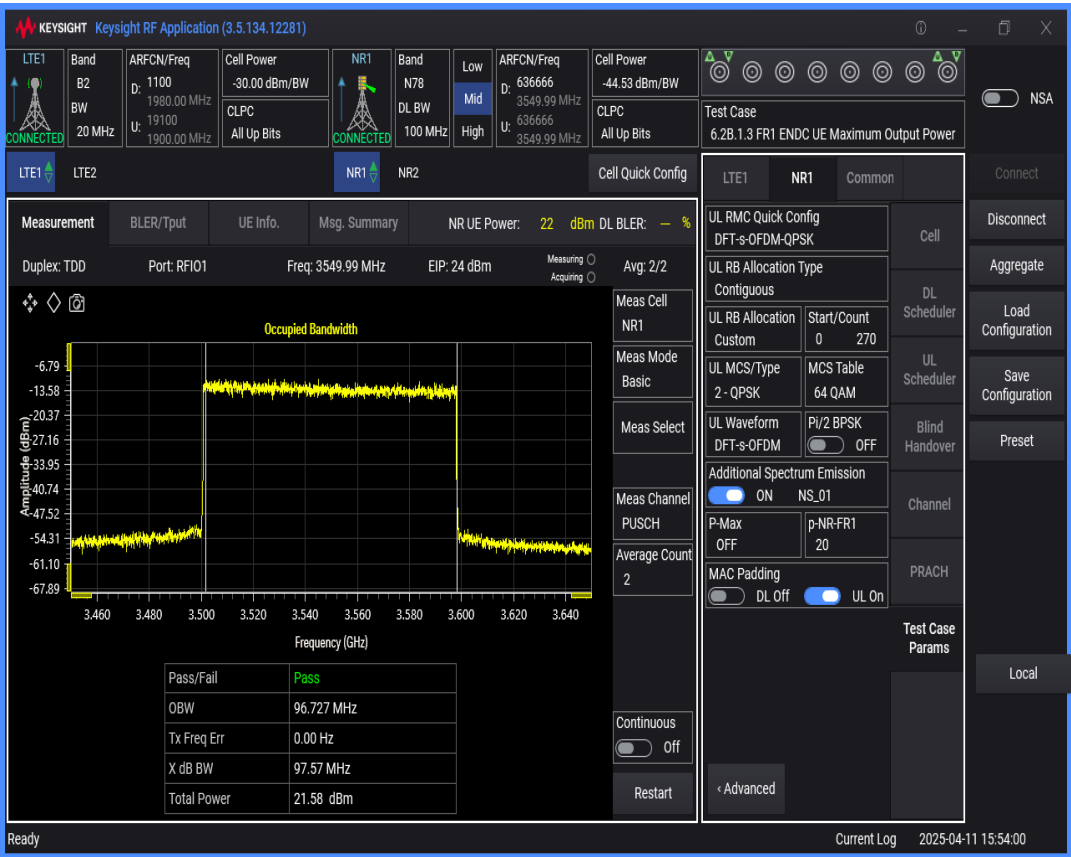
n78 SCS=30kHz DFT_QPSK BW=10MHz Channel=636666 RB=24@0
