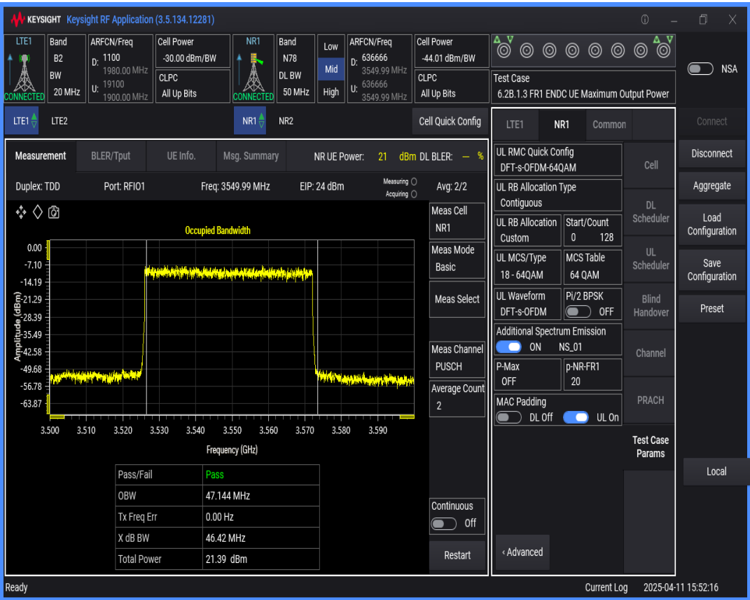
n78 SCS=30kHz DFT_QAM64 BW=15MHz Channel=636666 RB=36@0
