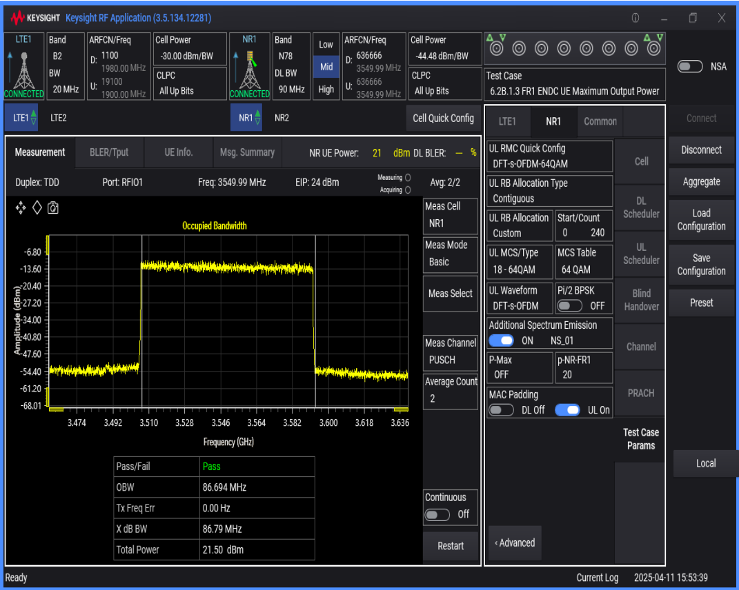
n78 SCS=30kHz DFT_QAM64 BW=50MHz Channel=636666 RB=128@0
