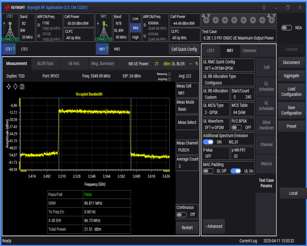
n78 SCS=30kHz DFT_QPSK BW=60MHz Channel=636666 RB=162@0
