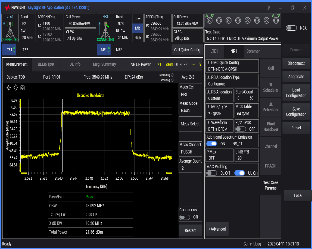
n78 SCS=30kHz DFT_QPSK BW=100MHz Channel=636666 RB=270@0
