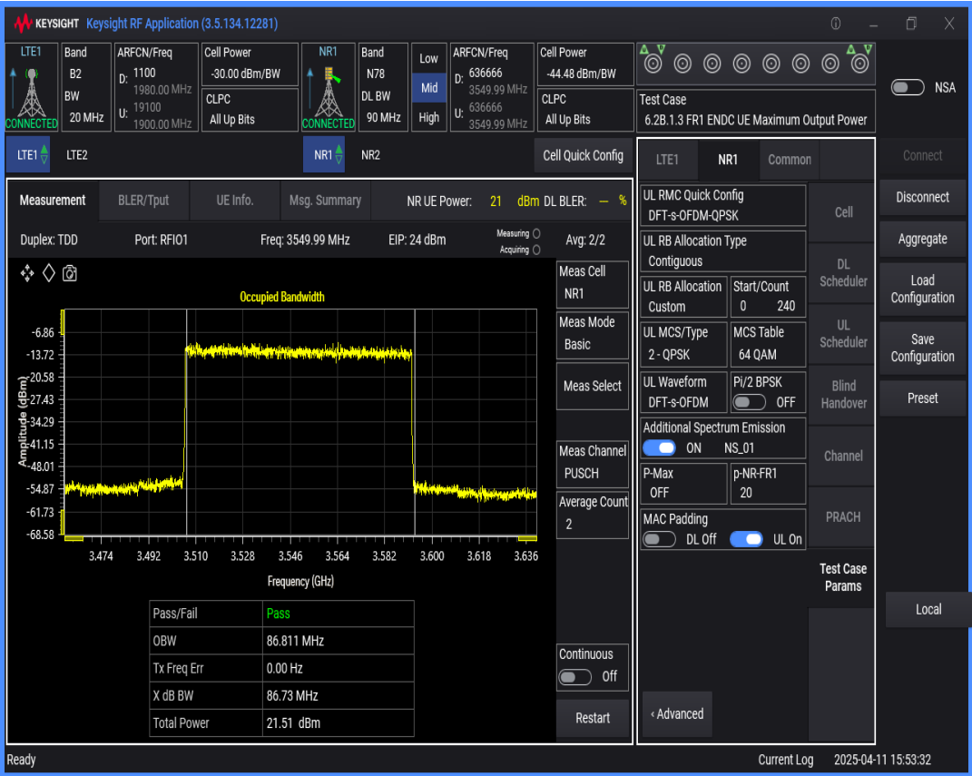
n78 SCS=30kHz DFT_QPSK BW=50MHz Channel=636666 RB=128@0
