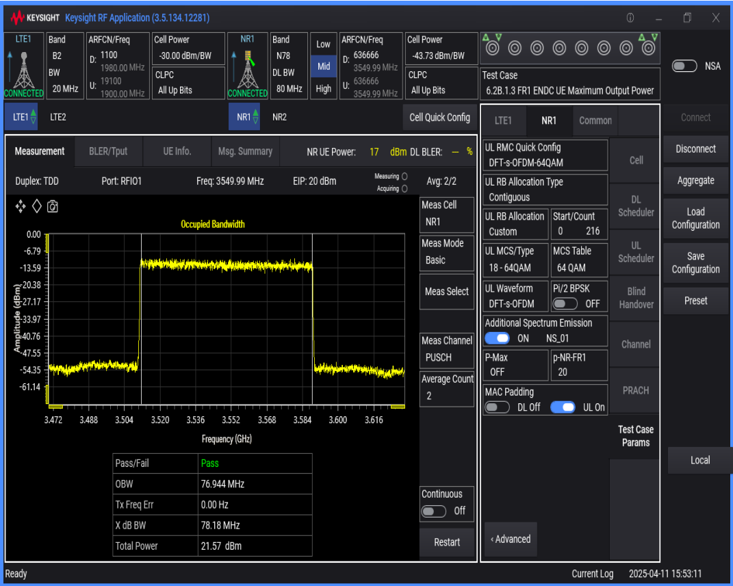
n78 SCS=30kHz DFT_QAM64 BW=90MHz Channel=636666 RB=240@0
