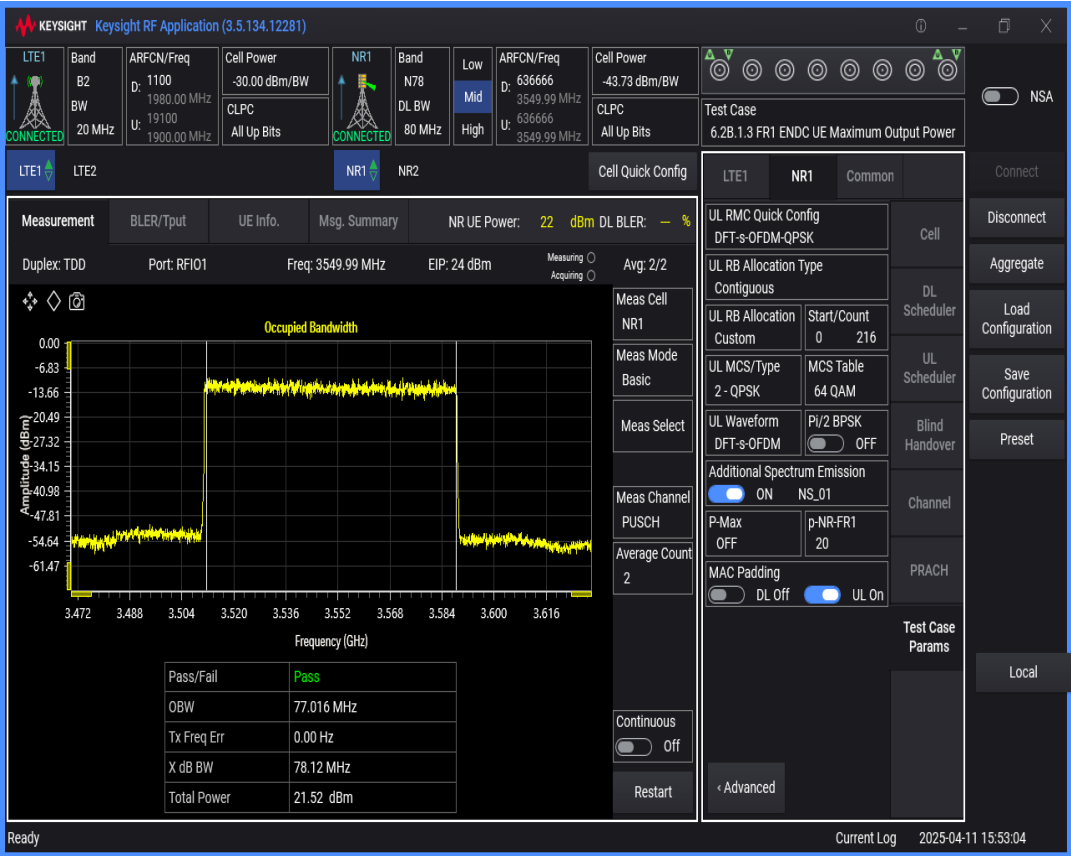
n78 SCS=30kHz DFT_QPSK BW=90MHz Channel=636666 RB=240@0
