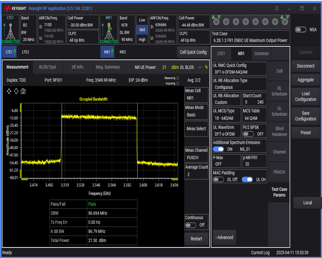
n78 SCS=30kHz DFT_QAM64 BW=60MHz Channel=636666 RB=162@0
