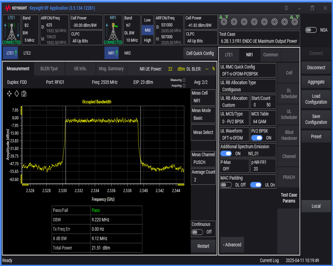
n7 SCS=15kHz DFT_BPSK BW=5MHz Channel=507000 RB=25@0
