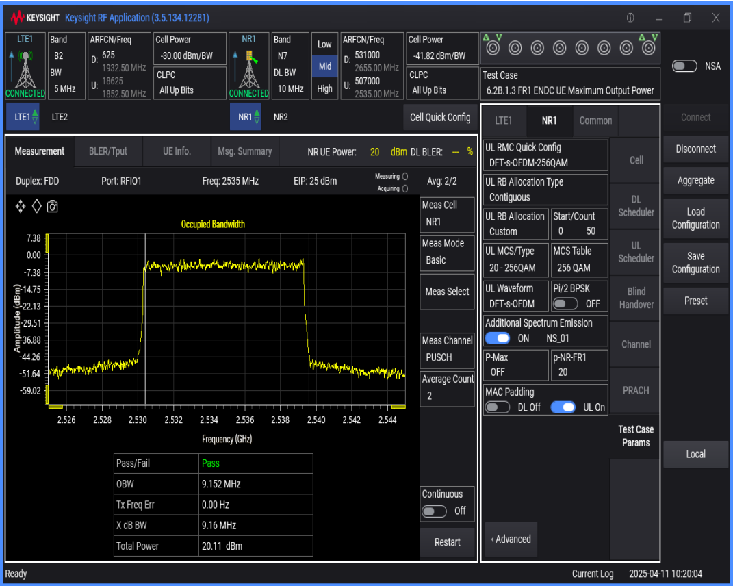
n7 SCS=15kHz DFT_QAM16 BW=5MHz Channel=507000 RB=25@0
