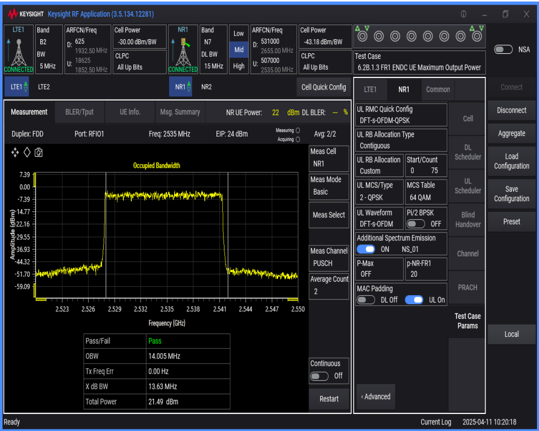
n7 SCS=15kHz DFT_QAM64 BW=20MHz Channel=507000 RB=100@0
