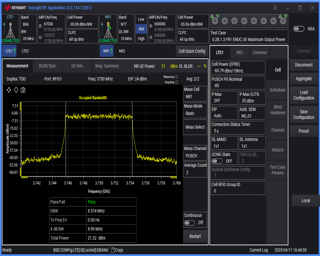
n77 SCS=30kHz DFT_QAM16 BW=100MHz Channel=650000 RB=270@0
