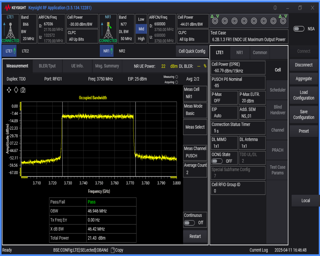
n77 SCS=30kHz DFT_QAM16 BW=40MHz Channel=650000 RB=100@0
