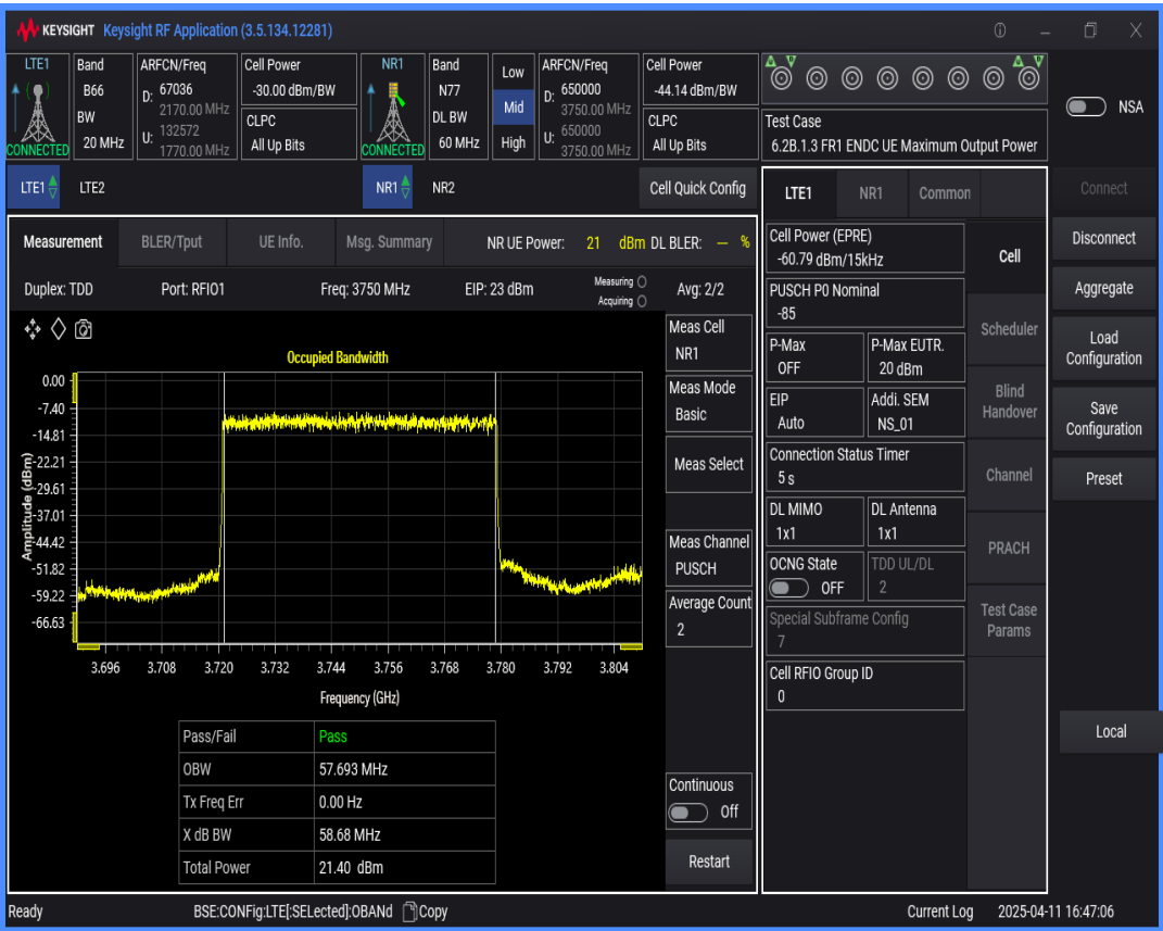
n77 SCS=30kHz DFT_BPSK BW=90MHz Channel=650000 RB=240@0
