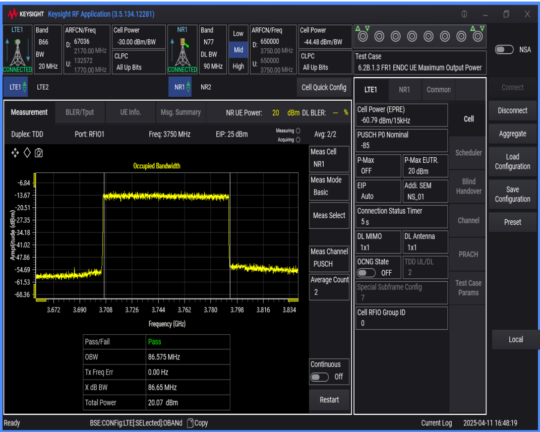
n77 SCS=30kHz DFT_QAM256 BW=80MHz Channel=650000 RB=216@0
