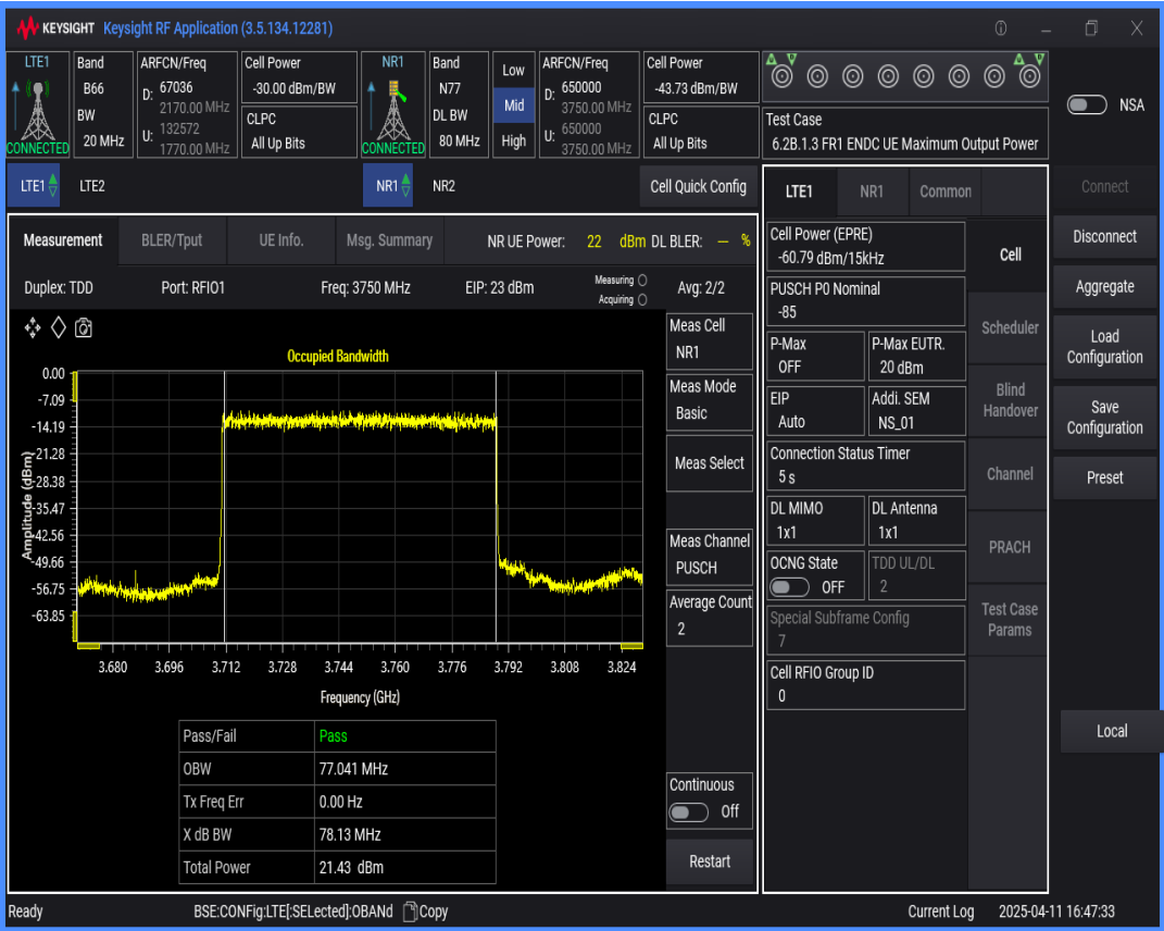
n77 SCS=30kHz DFT_BPSK BW=60MHz Channel=650000 RB=162@0
