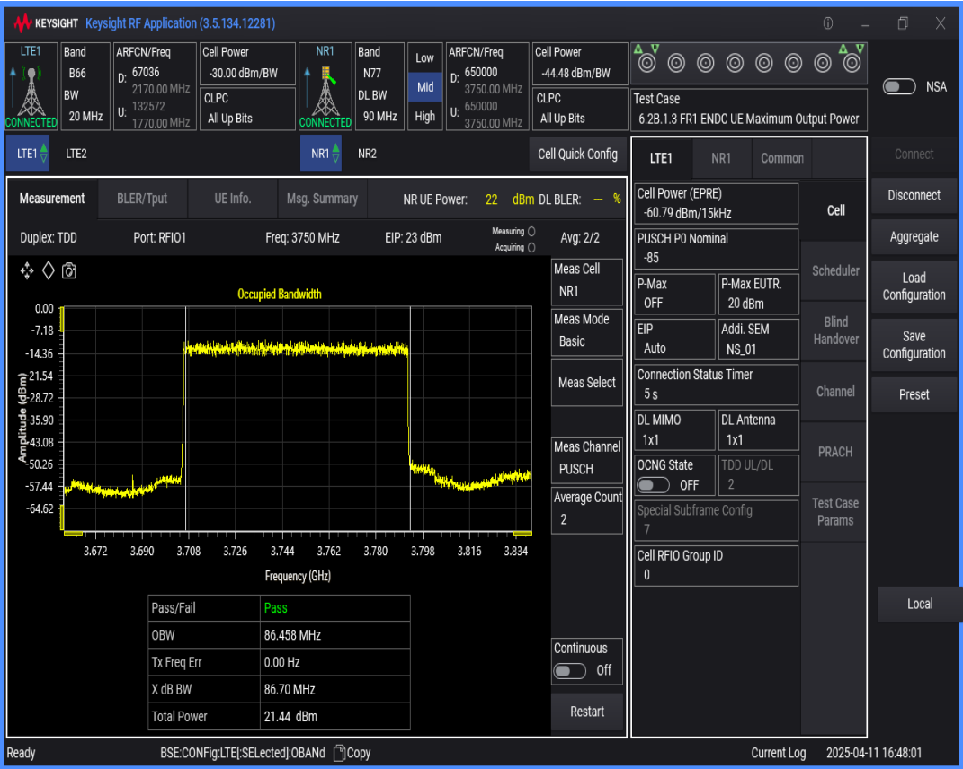
n77 SCS=30kHz DFT_QAM16 BW=10MHz Channel=650000 RB=24@0
