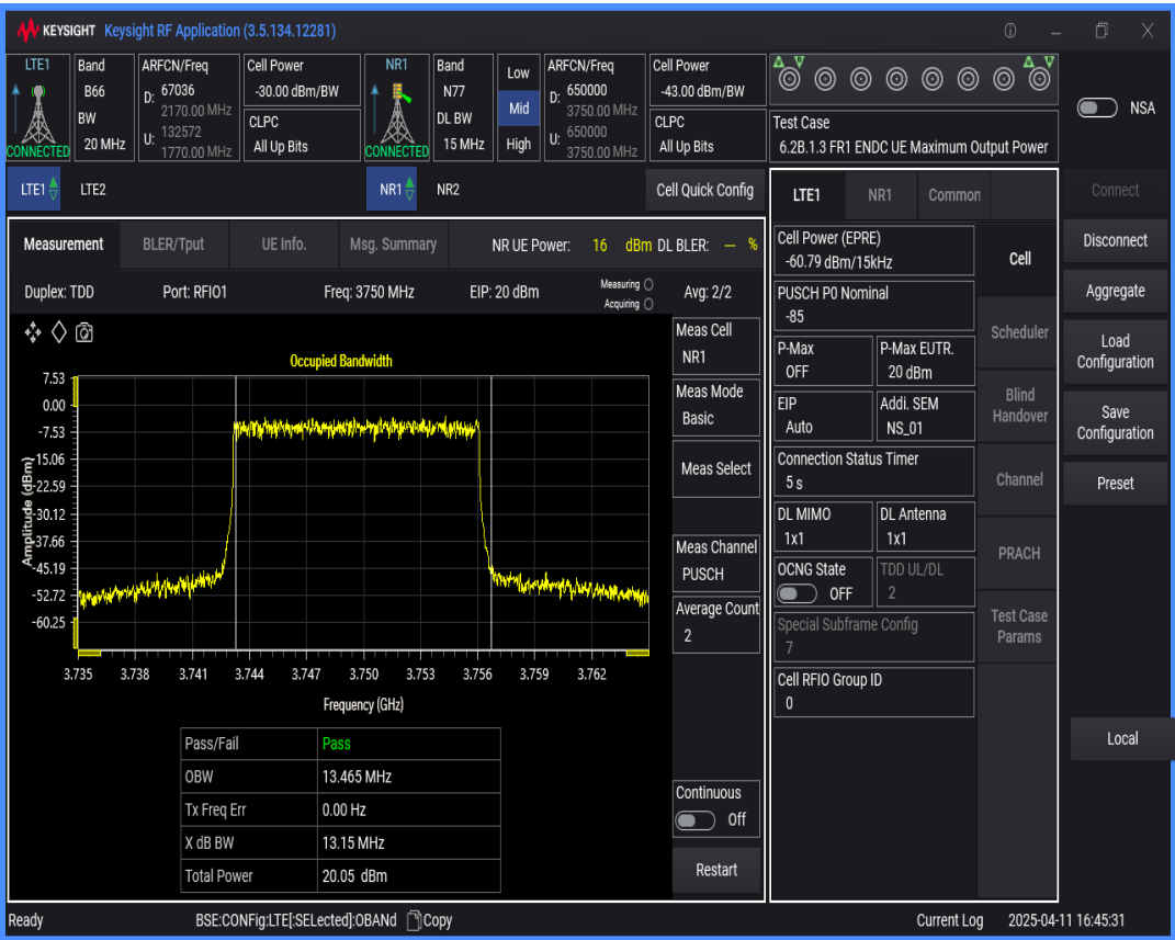
n77 SCS=30kHz DFT_QAM256 BW=40MHz Channel=650000 RB=100@0
