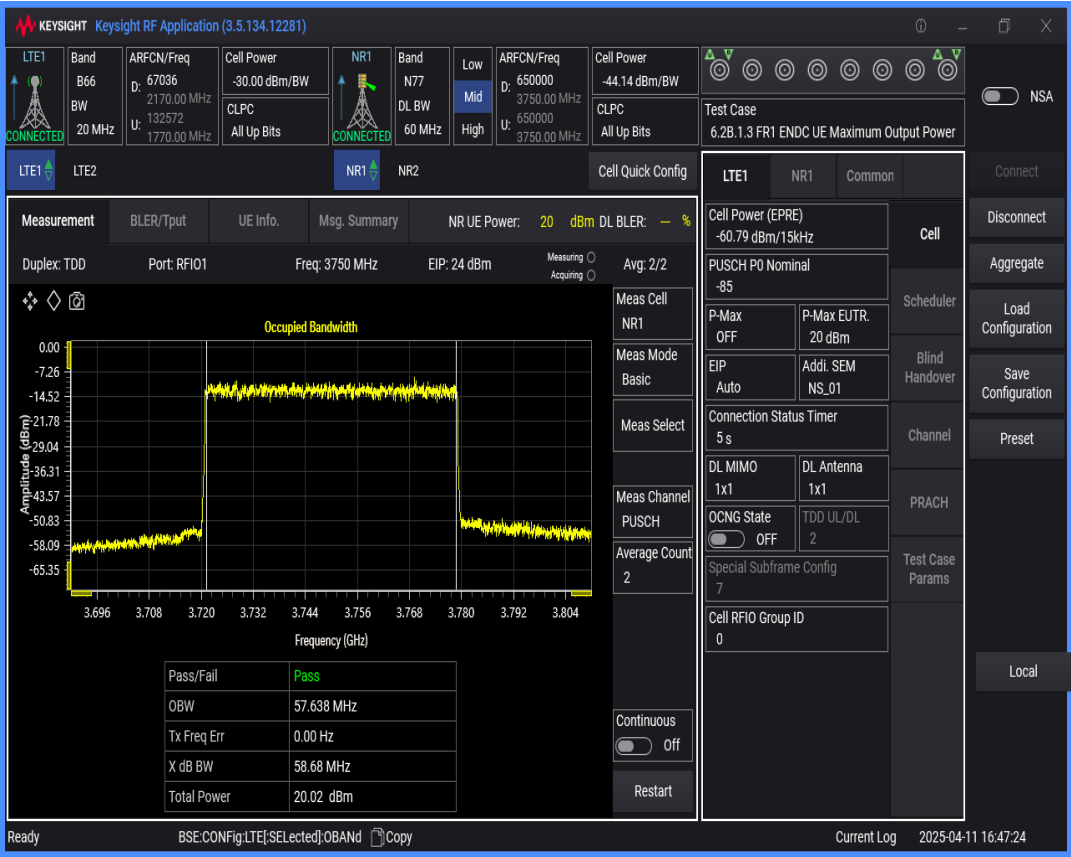
n77 SCS=30kHz DFT_QAM256 BW=50MHz Channel=650000 RB=128@0
