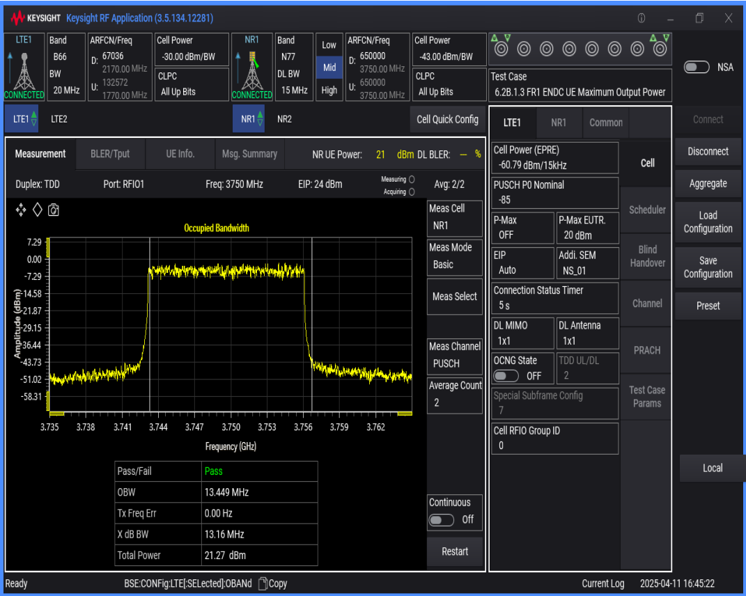
n77 SCS=30kHz DFT_QAM16 BW=50MHz Channel=650000 RB=128@0
