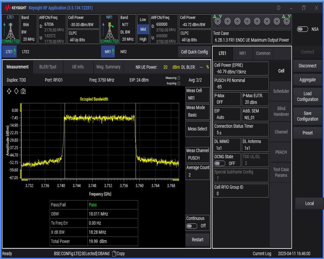
n77 SCS=30kHz DFT_QAM256 BW=15MHz Channel=650000 RB=36@0
