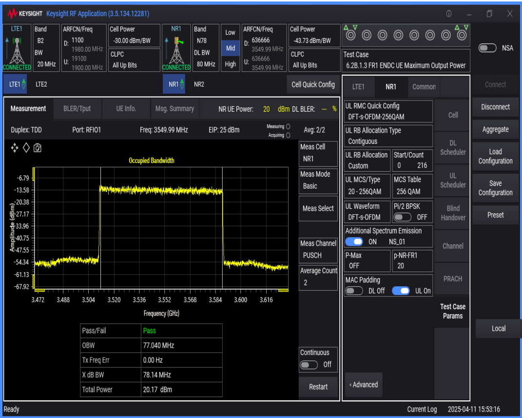
n78 SCS=30kHz DFT_QAM256 BW=90MHz Channel=636666 RB=240@0
