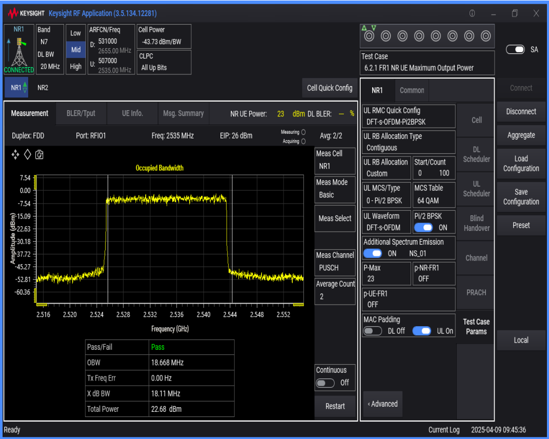
n7 SCS=15kHz DFT_BPSK BW=5MHz Channel=507000 RB=25@0
