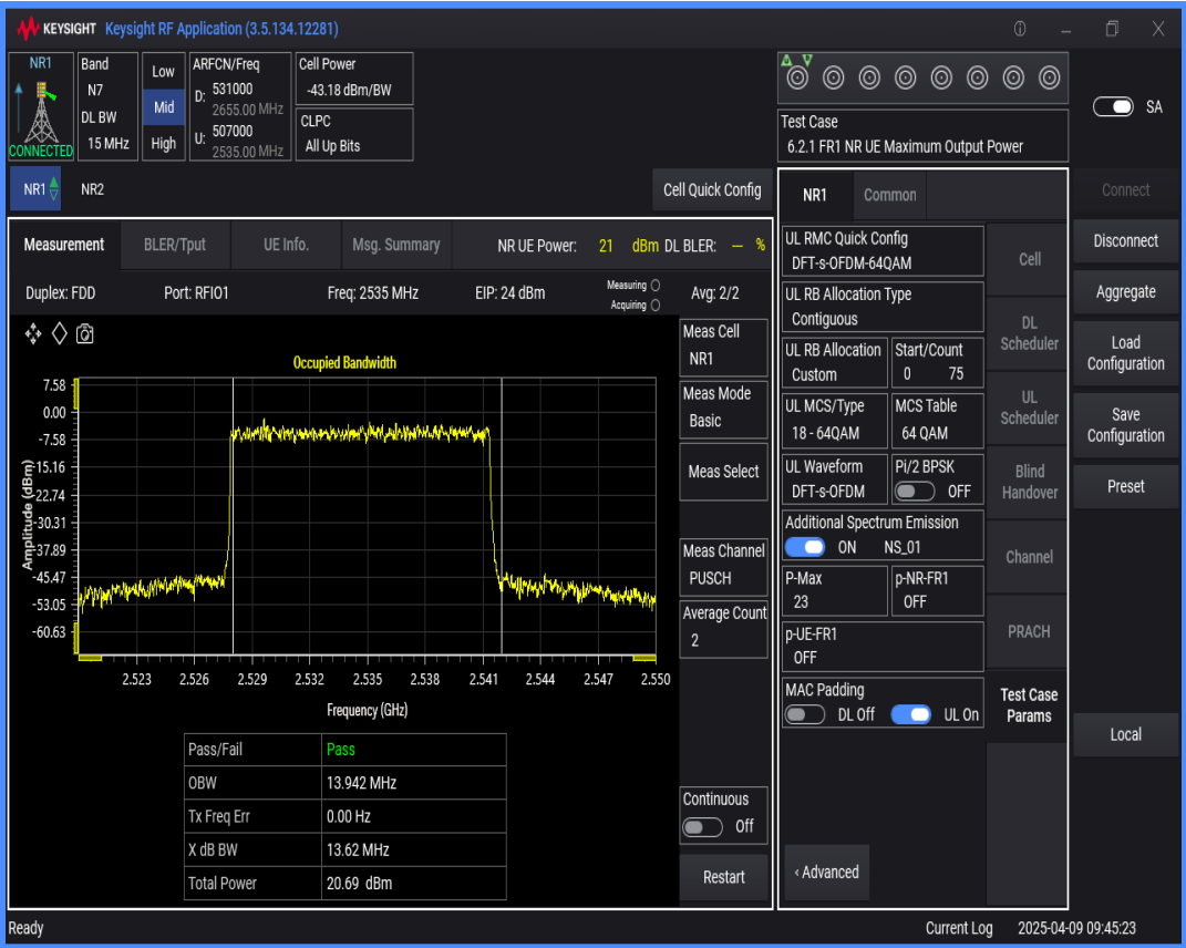
n7 SCS=15kHz DFT_QAM64 BW=5MHz Channel=507000 RB=25@0
