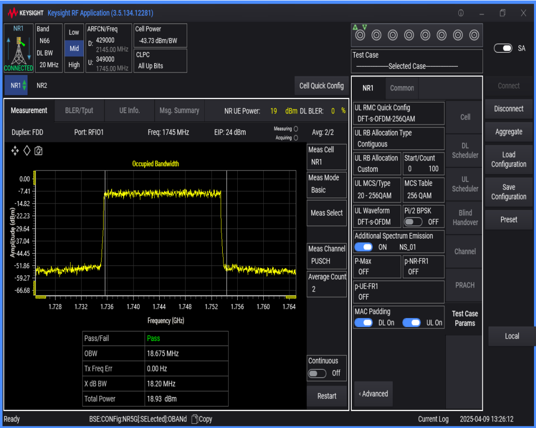
n66 SCS=15kHz DFT_QAM256 BW=40MHz Channel=349000 RB=216@0
