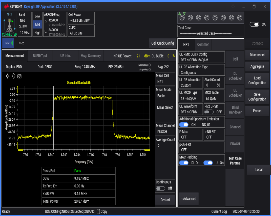
n66 SCS=15kHz DFT_QAM64 BW=20MHz Channel=349000 RB=100@0
