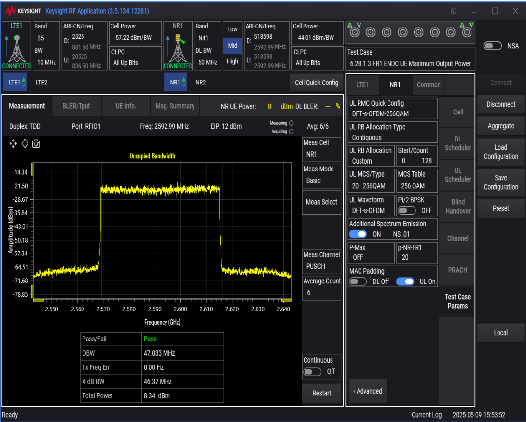
n41 SCS=30kHz DFT_QAM256 BW=60MHz Channel=518598 RB=162@0
