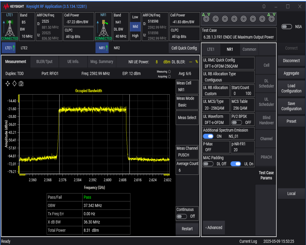
n41 SCS=30kHz DFT_QAM256 BW=50MHz Channel=518598 RB=128@0
