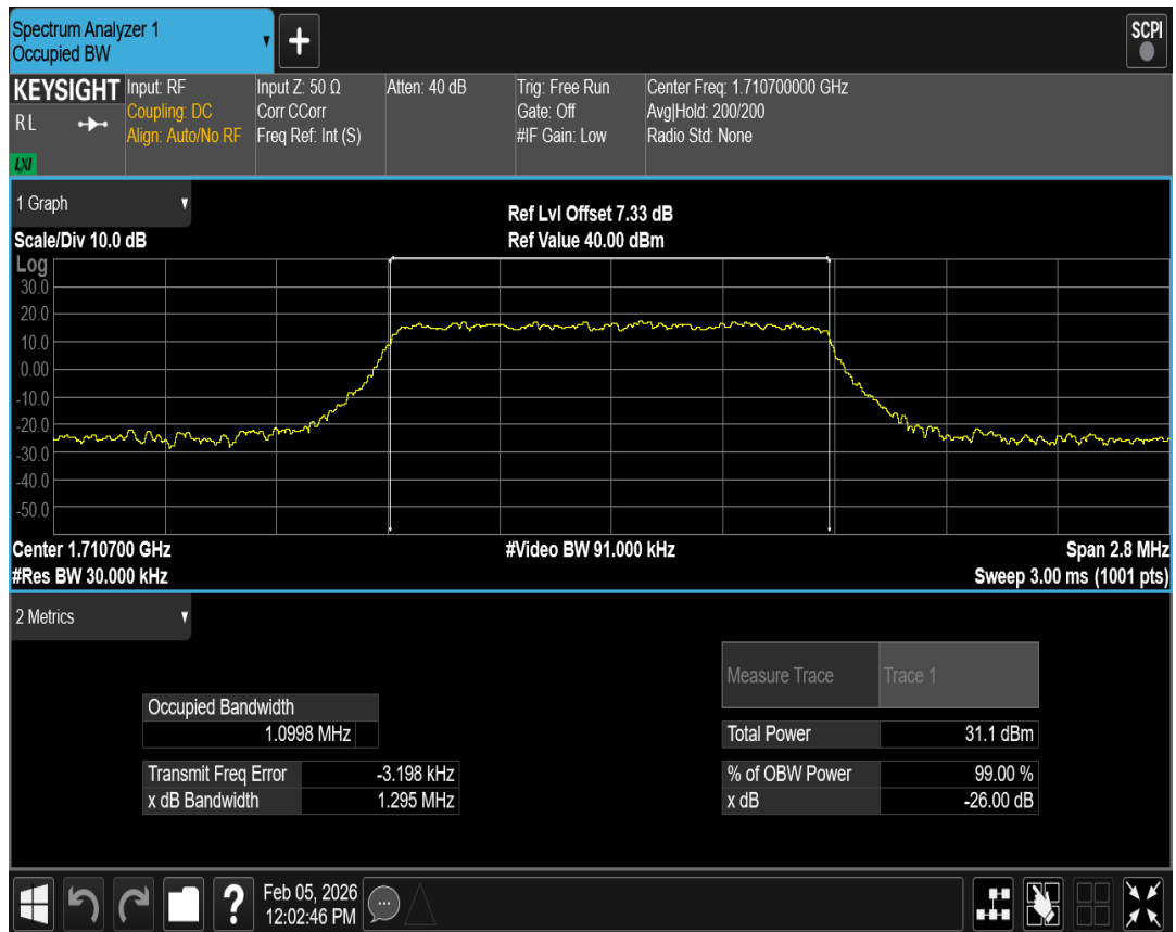
Band4 QPSK BW=1.4MHz Channel=20175 RB Size=6 Position=#0
