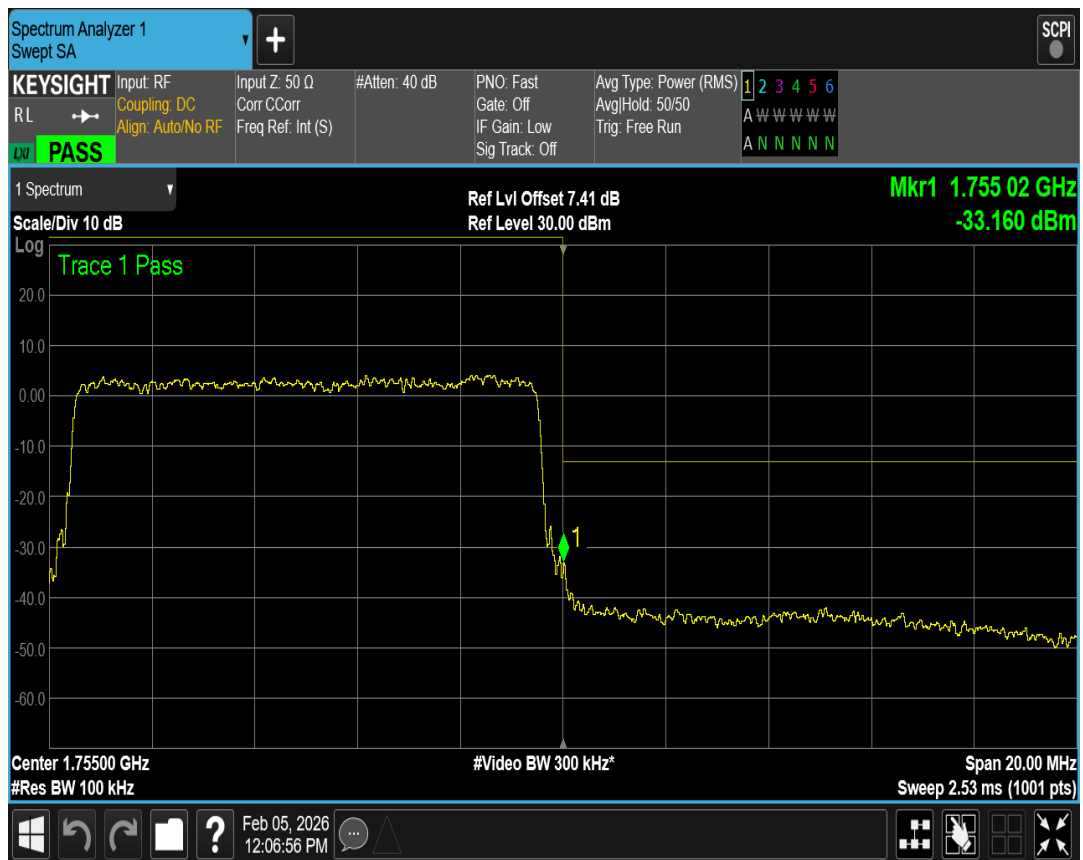
Band4 QAM16 BW=15MHz Channel=20025 RB Size=75 Position=#0
