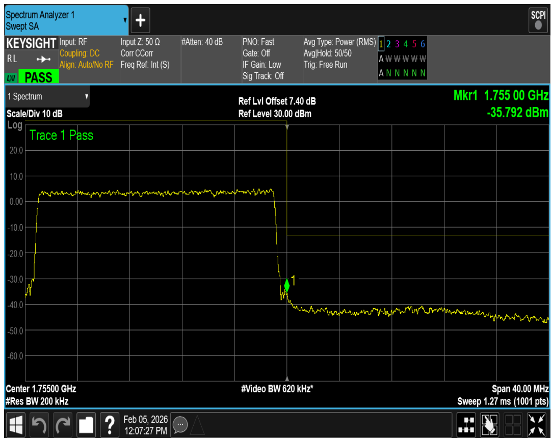
Band4 QPSK BW=3MHz Channel=19965 RB Size=15 Position=#0
