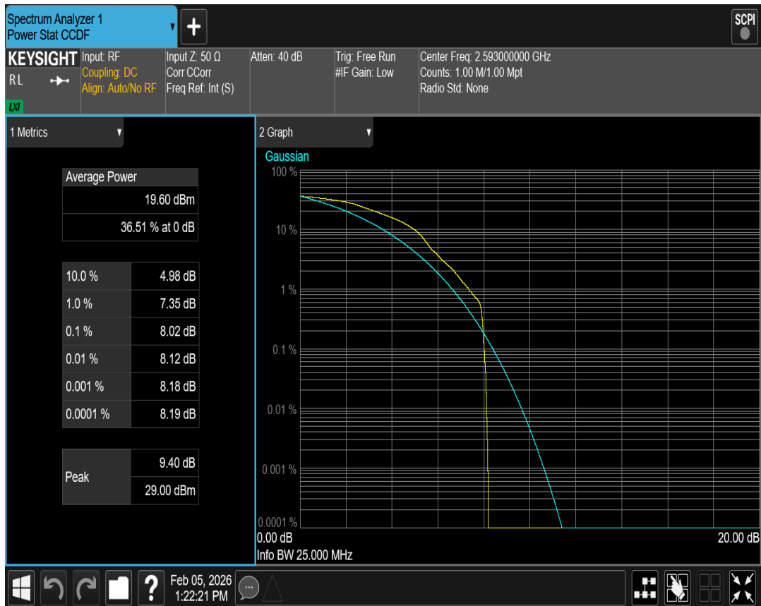
Band41 QPSK BW=10MHz Channel=40620 RB Size=1 Position=#0
