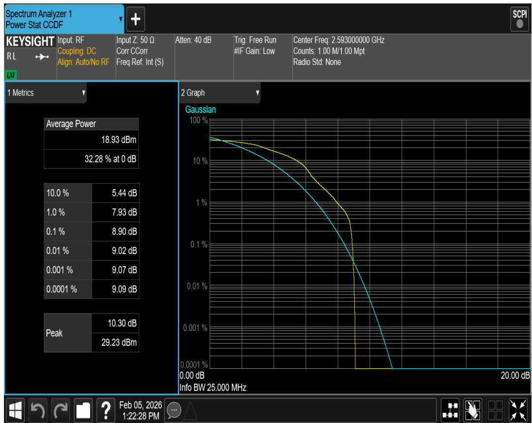
Band41 QAM16 BW=15MHz Channel=40620 RB Size=1 Position=#0
