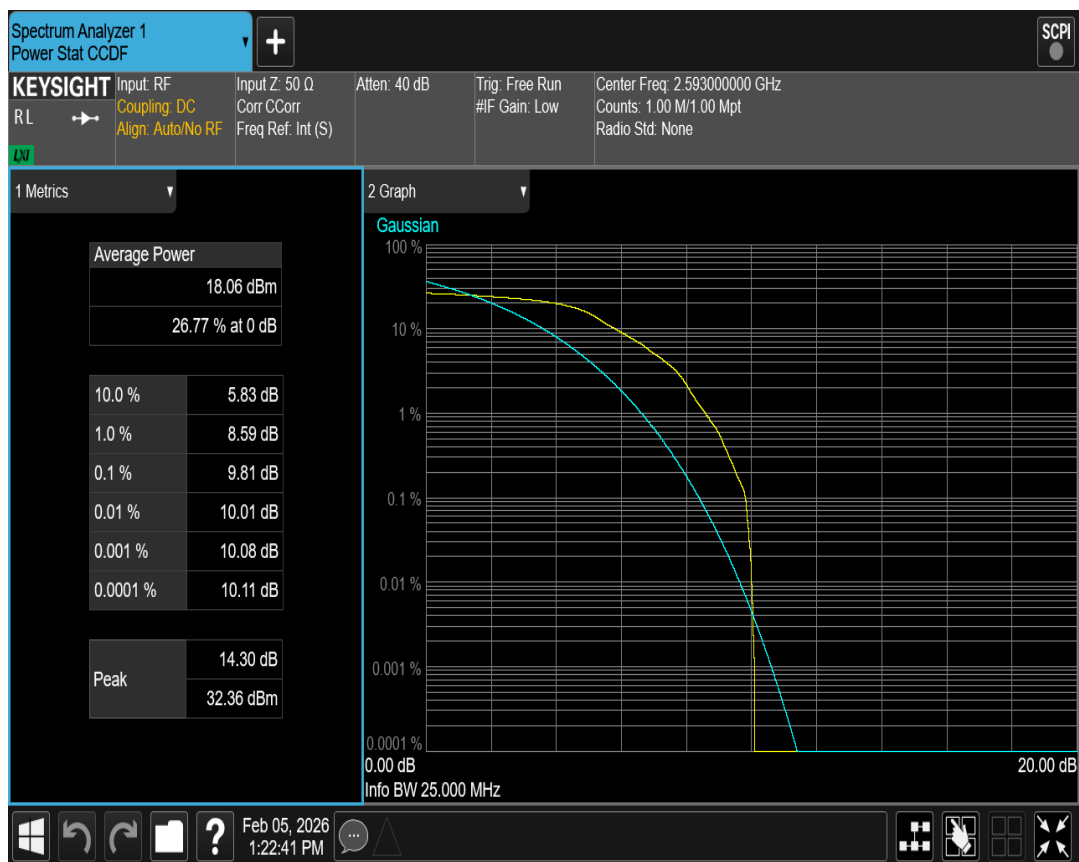
Band41 QPSK BW=5MHz Channel=40620 RB Size=1 Position=#0
