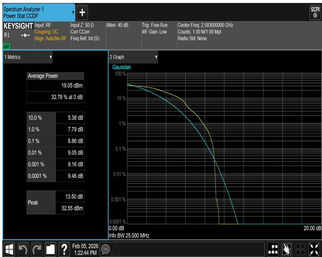
Band41 QAM16 BW=5MHz Channel=40620 RB Size=1 Position=#0
