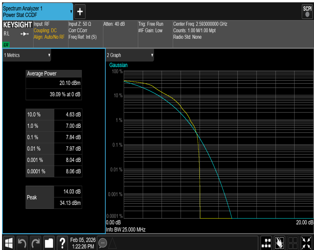
Band41 QPSK BW=15MHz Channel=40620 RB Size=1 Position=#0
