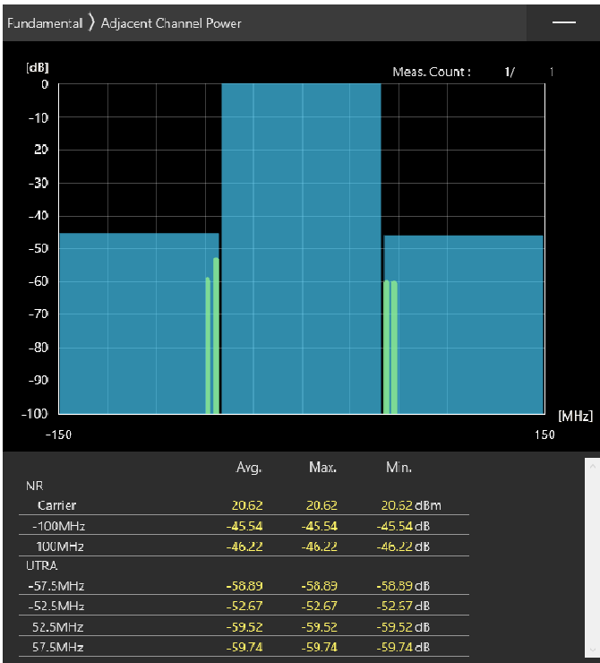
100MHz_30kHz_3600MHz-OFDM QPSK_RB1@0 -45.54,-46.22dB
