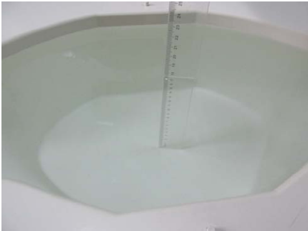
Photo 21: 2450 Body Liquid Depth \geq 15.0\text{cm}
