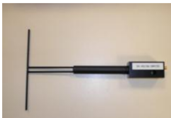
Figure 1 – Satimo COMOSAR Validation Dipole
