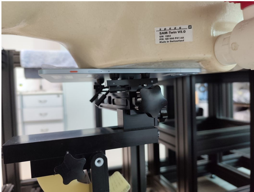
WLAN 2.4G Body Back Setup Photo (0 mm)
