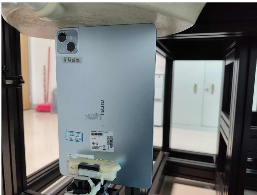
WLAN 2.4G Body Top Setup Photo (0 mm)
