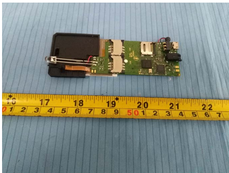
EUT – Mainboard Bottom Shielding off View
