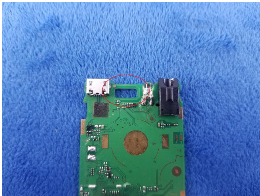
BT - Antenna View
