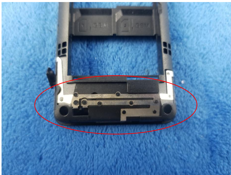
GSM/PCS - Antenna View
