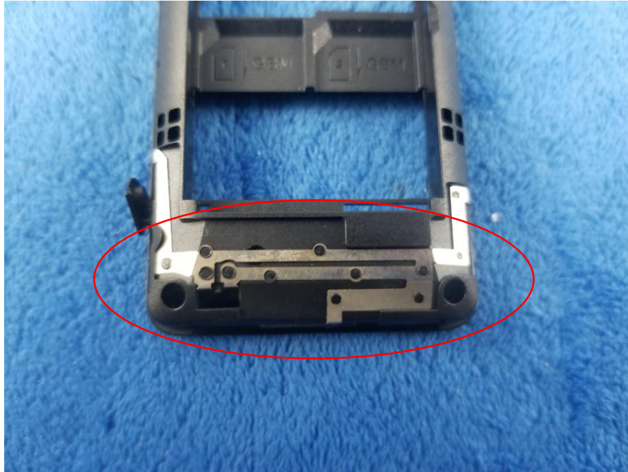
GSM/PCS/UMTS-FDD - Antenna View
