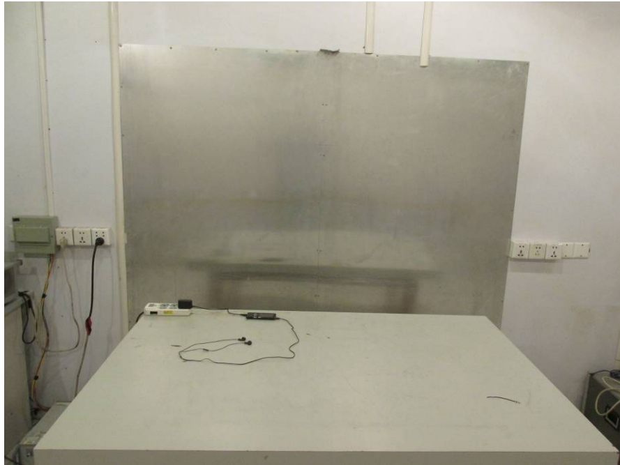
CONDUCTED EMISSION TEST
